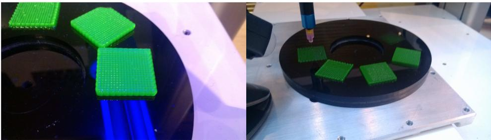
**Figure 1.3.:** Demonstration of our print at the “notte dei ricercatori” (researchers night), extruding a fluorescein loaded gel. A 3 dimensional grid was manufactured with 20 layers
