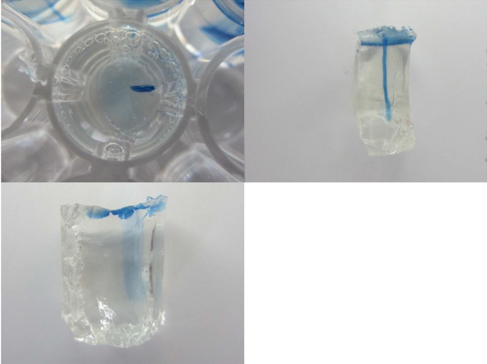
**Figure 2.4.:** 30 vertical injection in gelatin forming a continuous 3mm section in x-z. (hydrogel formed starting from a PBS solution)
