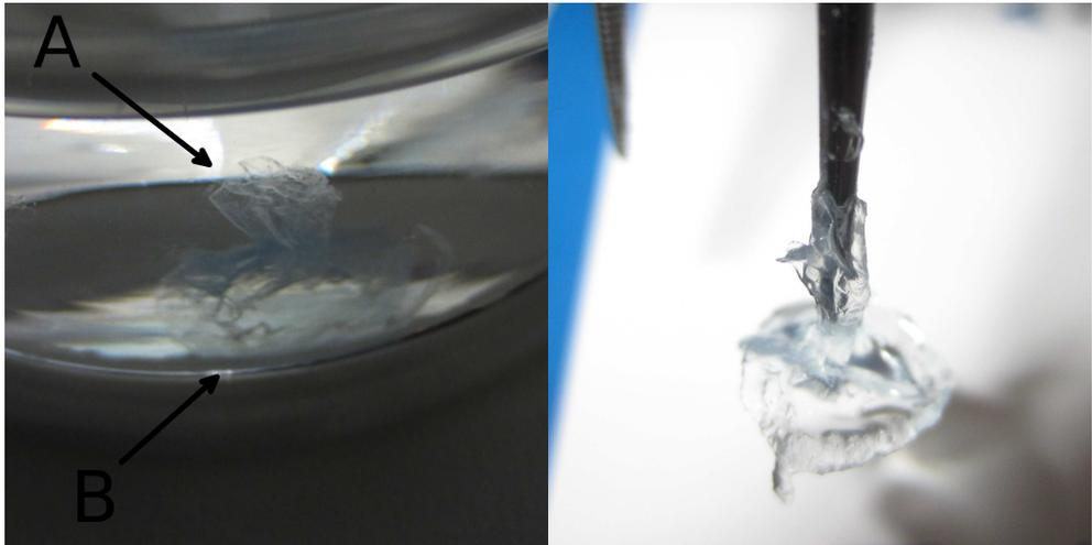
**Figure 2.6.:** Alginate sample after postprocessing. Left: sample inside the warm PBS bath. The upper part marked as A is the parallelepiped injected while the lower part B is a residue of the injection process. Right: Sample removed from the bath.
