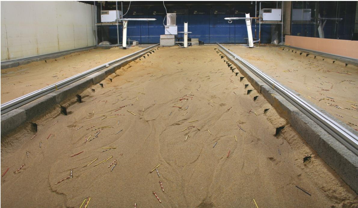
Figure 4.31: The TES Flume showing the configuration used for the present work. Flow is towards the camera.
