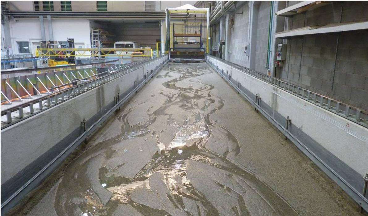
Figure 4.1: The Pi Flume. Flow is towards the camera.
