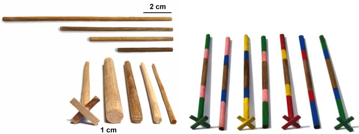
Figure 4.7: Size range of the dowels and an example of colour-coding.
