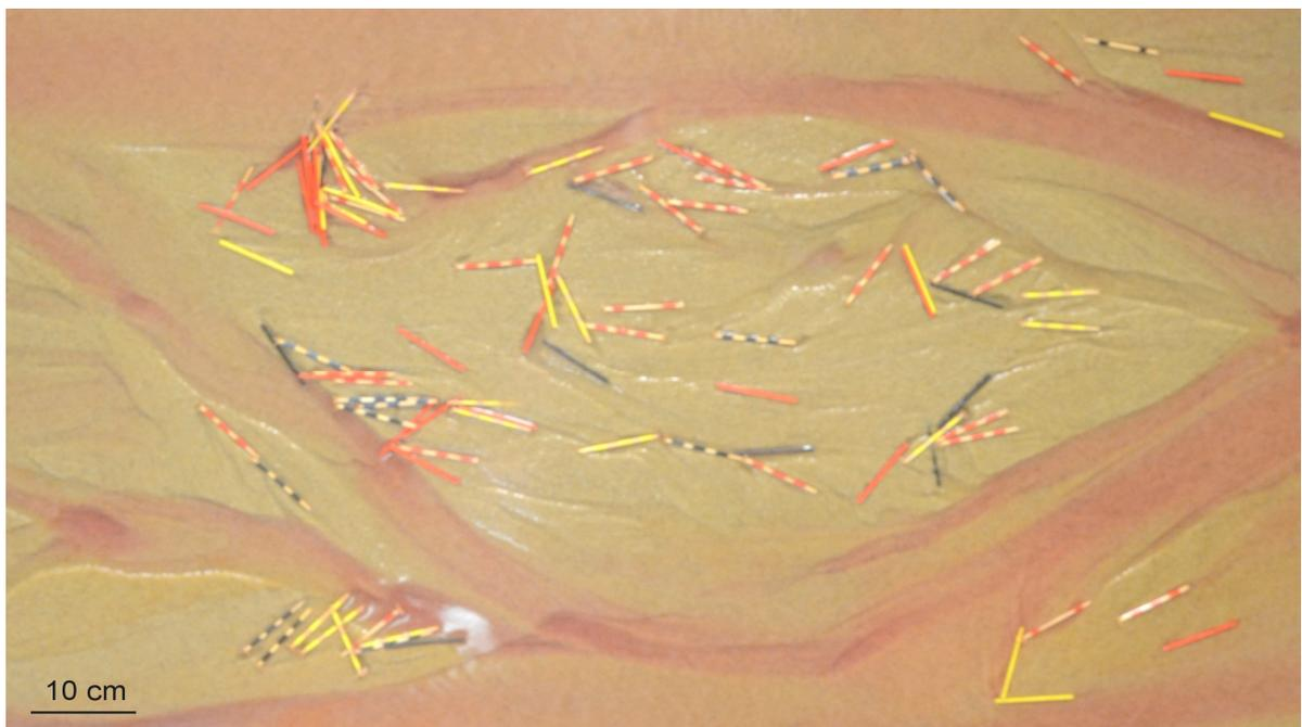
Figure 4.33: Detail of wood deposited on a bar, including jams of various size and isolated log; solid colour dowels have no root wad. Flow is from left to right.
