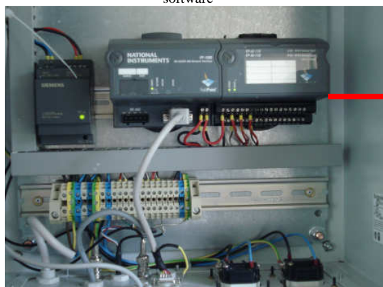
C. Acquisition hardware (Field Point FP 1000 and FP-AI-110)
