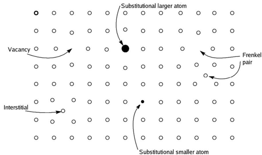
**Figure 1.1:** Schematic representation of possibilities of dopants in lattice sites [47]
