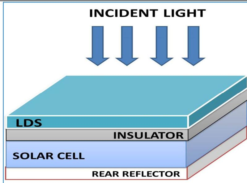
**Figure 1.12:** Schematic representation of a solar cell device with a luminescent down-shifting layer placed onto the top of the solar cell [216]
