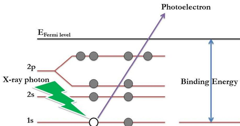
**Figure 2.6:** A scheme of X-ray photoelectron spectroscopy process
