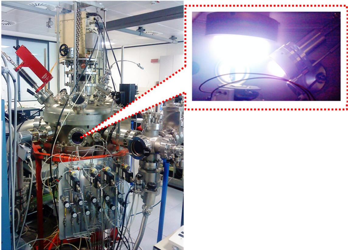
**Figure 2.2:** A photograph of vacuum system used in the present study and plasma generated during the RF co-sputtering process.
