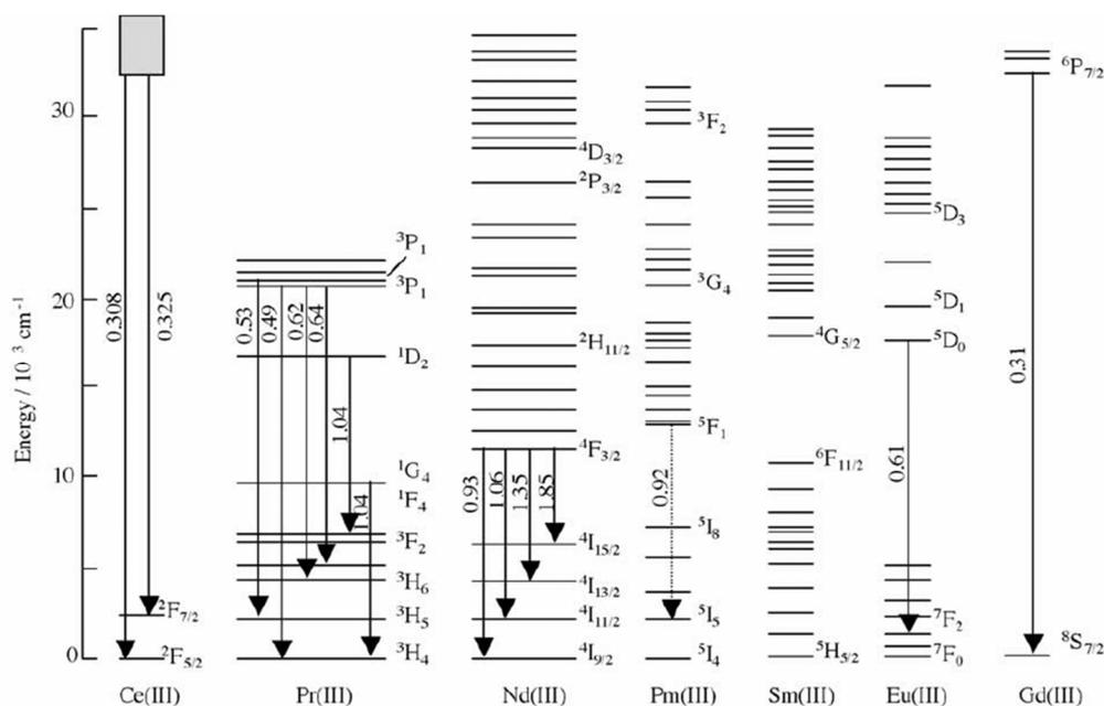
**Figure 1.9:** Electronic states (Dieke diagram) for a selective of Ln(III) ions (Cerium, Praseodymium, Neodymium promethium, Samarium, Europium, Gadolinium). Solid black arrows indicate radiative transitions [Figure adapted from 231]
