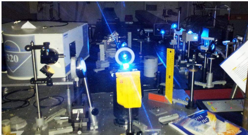
**Figure 2.11:** *Photoluminescence instrumentation set up equipped with YAG laser for 355 nm excitation*
