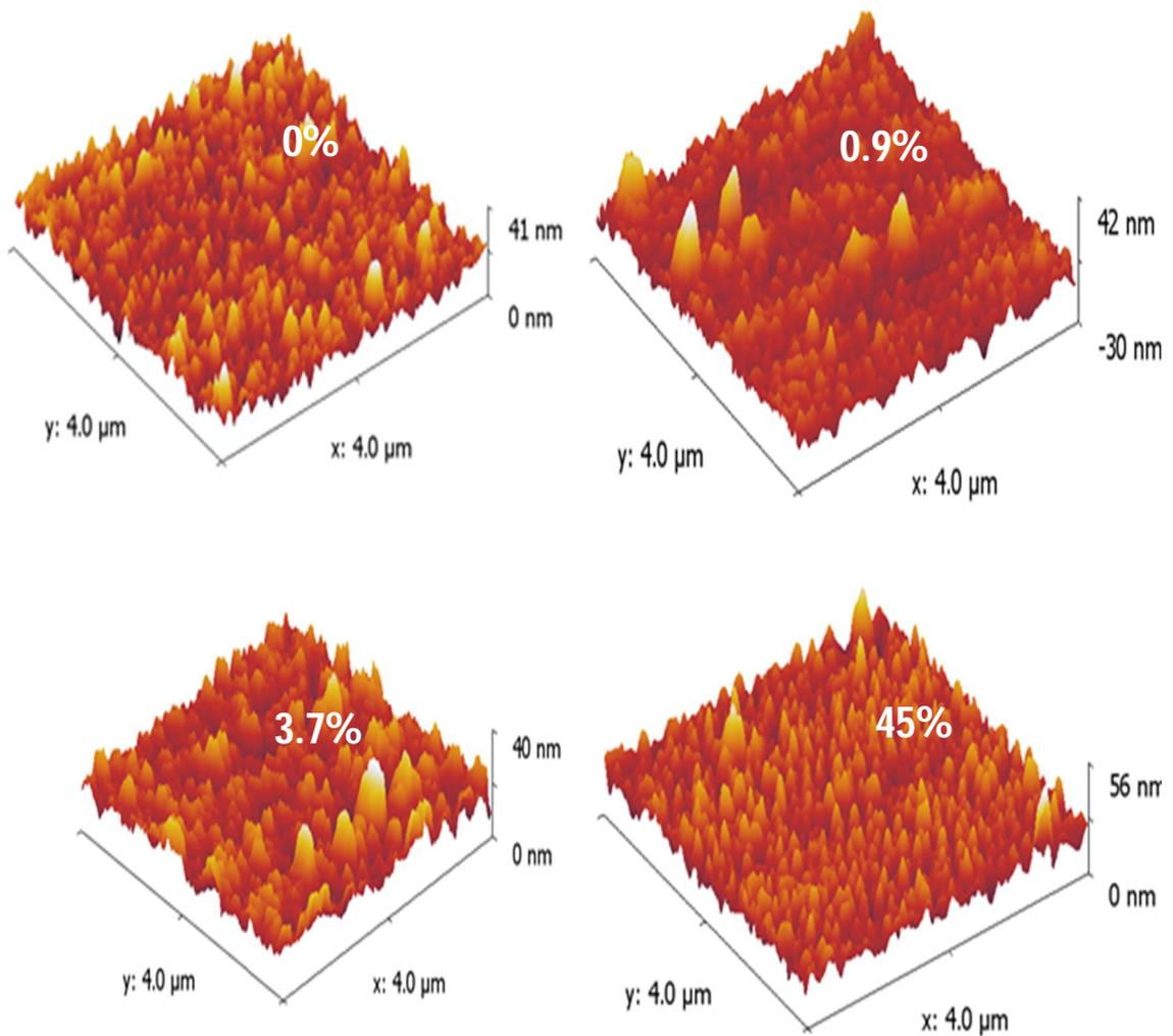
**Figure 3.11:** Three dimensional AFM Images of Undoped (0%), and doped  $\text{TiO}_2$  with Nd/Ti ratio of 0.9%, 3.7% and 45% on quartz substrates.
