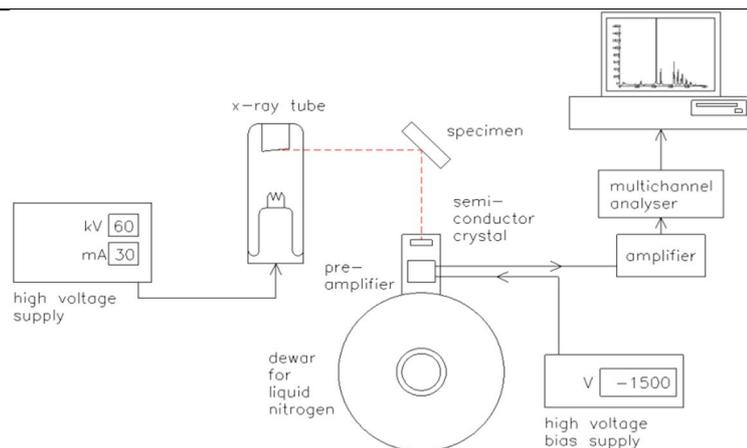
**Figure 2.8:** *Typical XRF set up*
