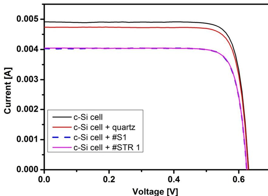
**Figure 6.13:** *I-V curves of the c-Si cell with and without the DS layer located on the top surface of the cell.*
