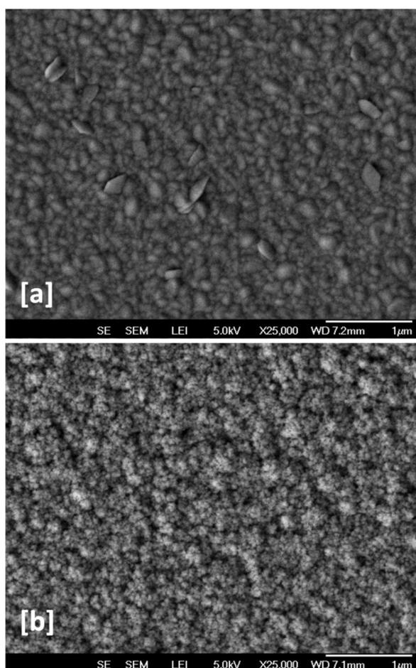
**Figure 4.10:** SEM micrographs of (a) a pure ZnO film (sample S1) and (b) sample S5.
