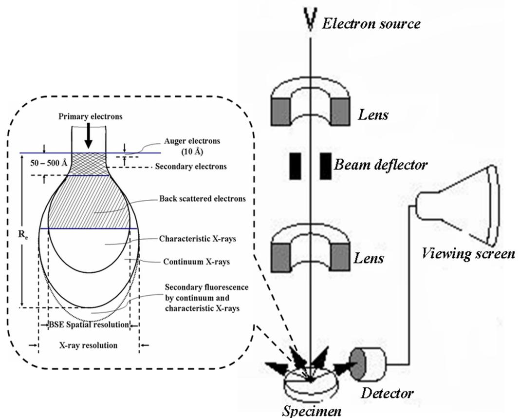
**Figure 2.9:** The ray diagram of SEM with an insert of interaction of X-rays with the specimen.
