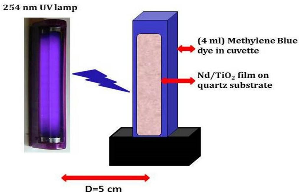
**Figure 2.14:** Schematic set up of Photocatalytic experiment
