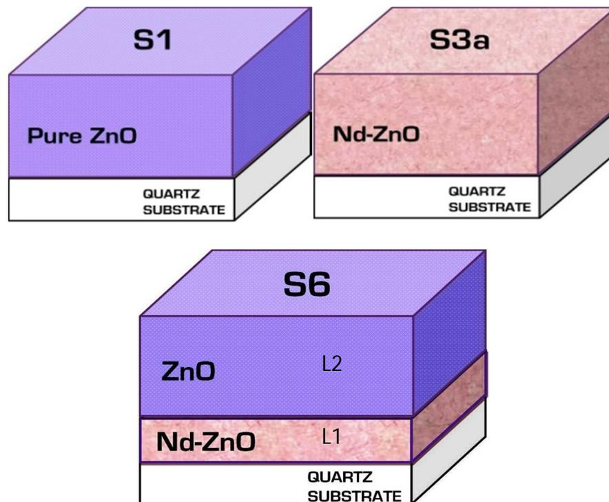
**Figure 4.12:** Schematic illustration of the sample S1, S3a and S6.
