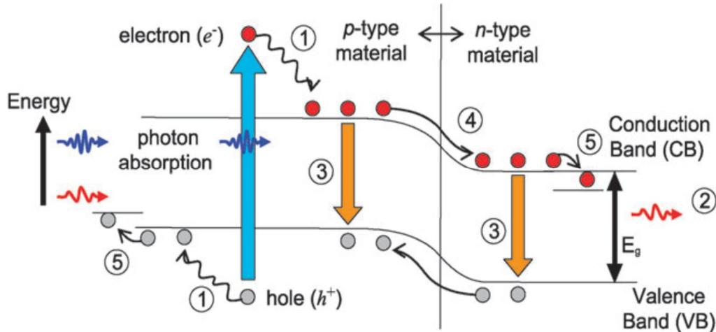
**Figure 1.11:** Loss Mechanism in a single junction solar cell [adapted from 210, 211]
