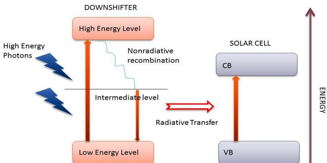
**Figure 1.13:** Schematic Energy diagram of a solar cell in combination with active luminescence downshifter layer [217]
