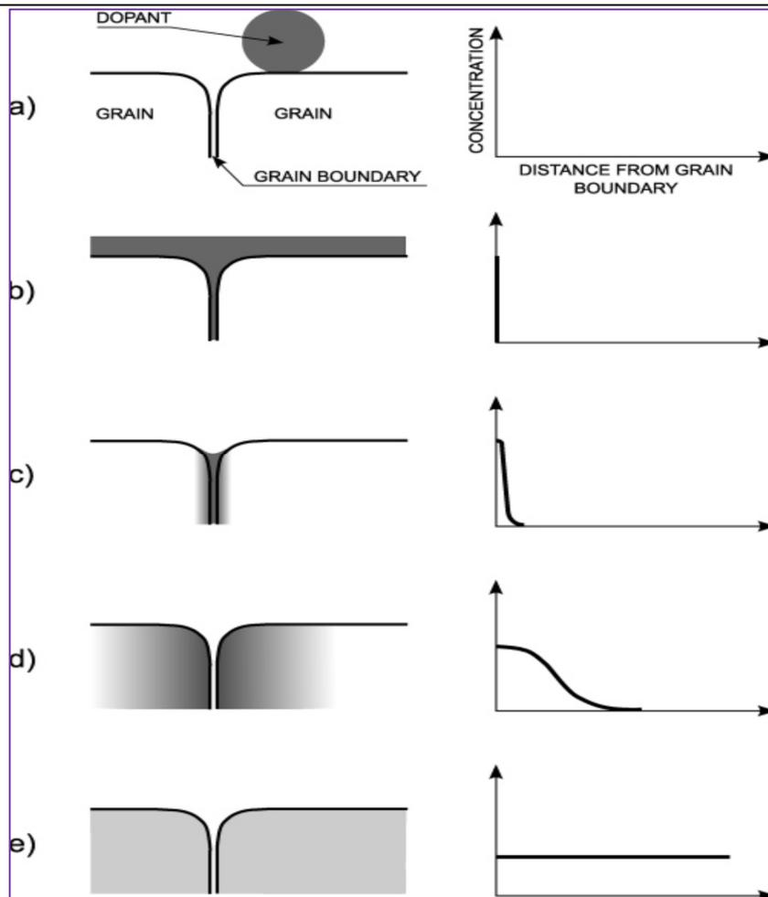
**Figure 1.2:** Possible doping mechanisms of polycrystalline  $\text{TiO}_2$ , involving (a) deposition of isolated islets on the surface, (b) spread of the dopants on the surface and within grain boundaries, (c) filling of grain boundaries leading to limited diffusion profile, (d) limited bulk transport leading to the formation of a concentration gradient, and (e) homogeneous distribution of the dopant within the specimen. [Figure & concepts adapted from Reference 50]
