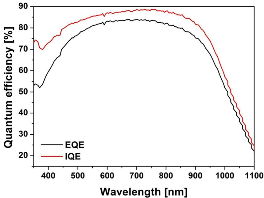
**Figure 6.12:** Internal (red curve) and External (black curve) quantum efficiency of the c-Si cell.
