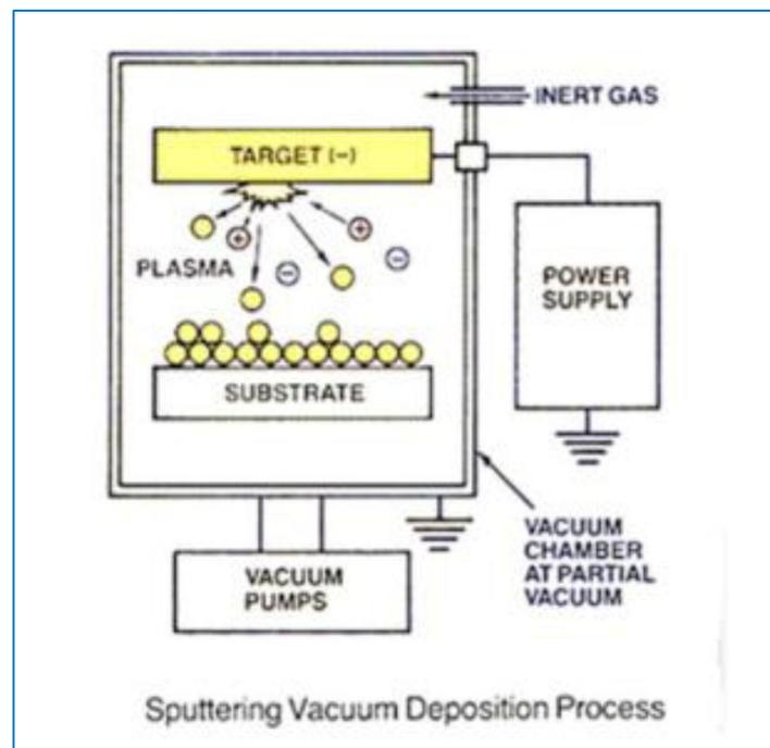
**Figure 2.1:** *The principle of RF Sputtering*
