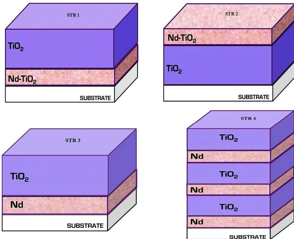
**Figure 6.8:** Layer Architecture of the selected  $\text{TiO}_2$ : Nd samples #STR 1, #STR 2, #STR 3 and #STR 4 and the corresponding sample deposition parameters are described in Table 6.3.
