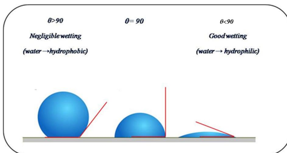
**Figure 2.12:** Schematic representation of contact angle of sessile drop on the substrate [adapted from the reference 12].
