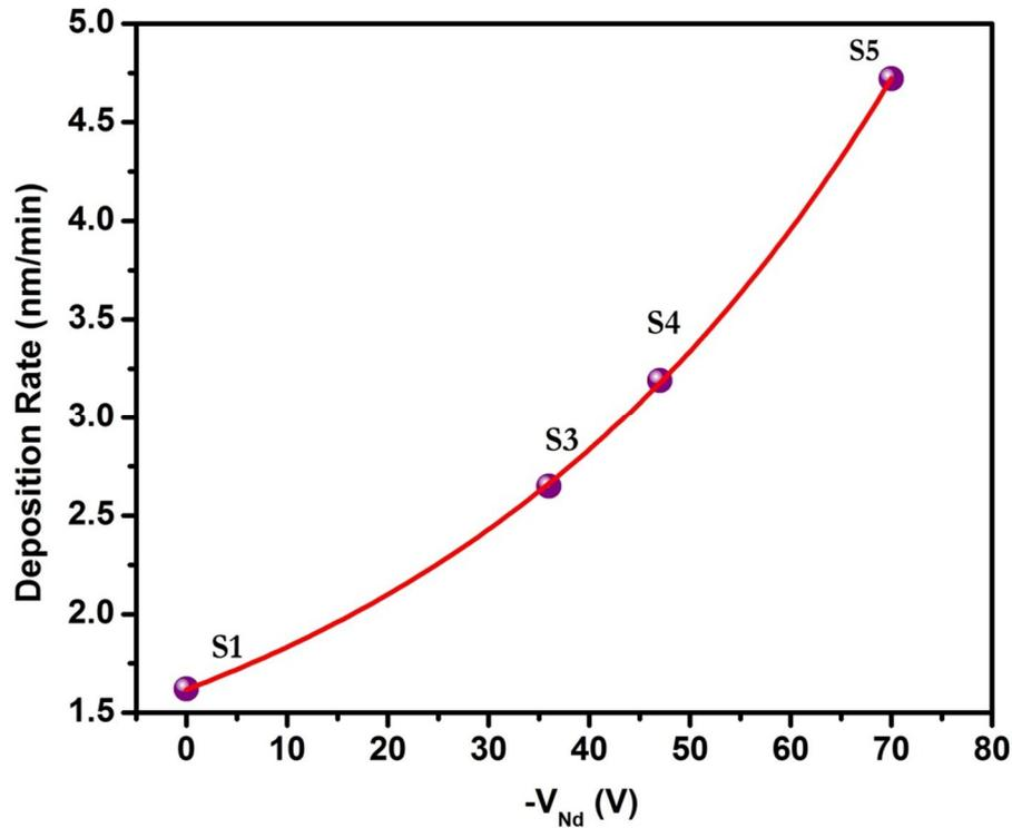
**Figure 3.1:** Film growth rate for co-sputtered at room temperature Nd-  $TiO_2$  deposited in Ar plasma as a function of the self-bias on Nd target,  $V_{Nd}$ , with a constant  $V_{TiO_2}$ . The data are also identified by the sample labeling.
