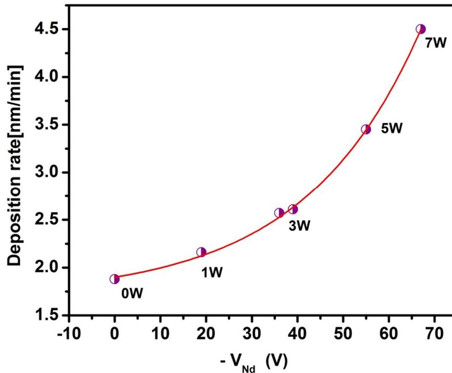
**Figure 4.1:** Film growth rate for co-sputtered Nd- ZnO films as a function of the self-bias voltage at Nd target,  $V_{Nd}$ . The relative electrical powers are given in the plot.
