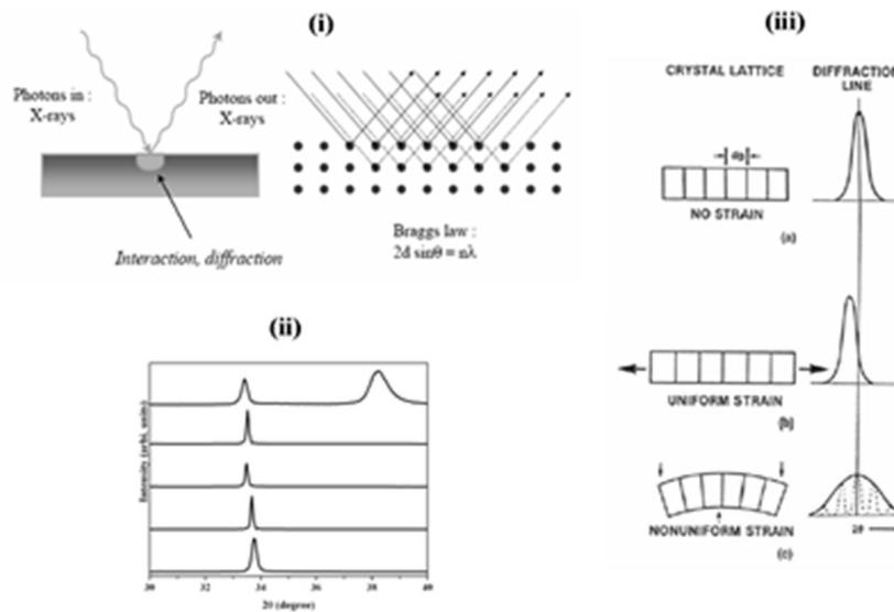
**Figure 2.3:** X-ray reflection characteristic of the material, and the changes in peak shape due to different strains (adapted from the Reference [6])
