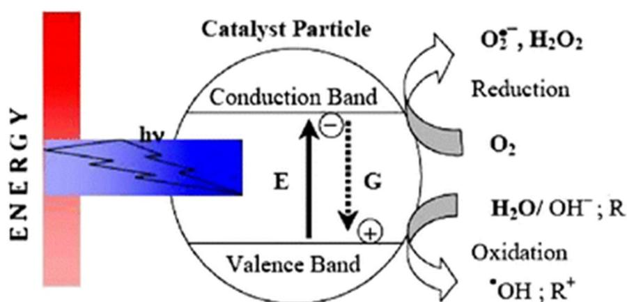
**Figure 1.14:** Schematic representation of photocatalytic process [figure adapted from 230]
