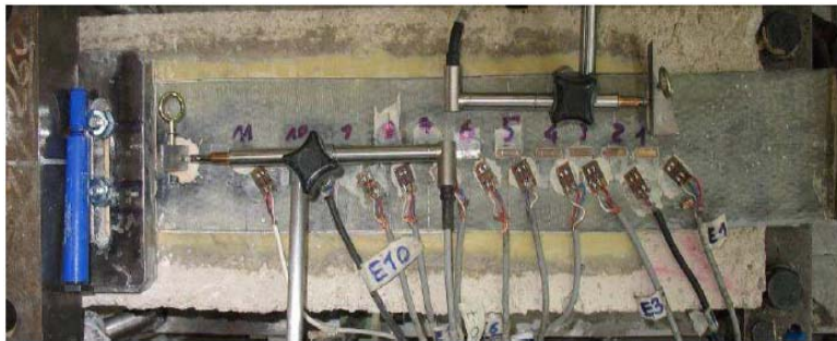
Fig. 57 Test a "single shear" (Iovinella, 2010)
