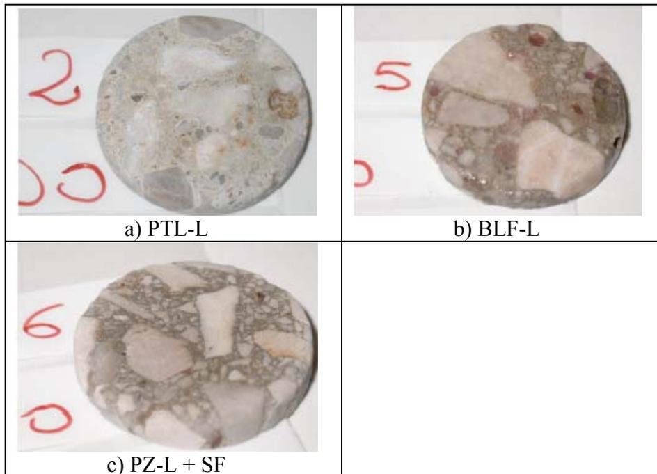
**Figure 7 – Phenolphthalein method results (EN 9944) on three mixtures ( a) PTL-L, b) BLF-L and c) PZ-L+SF) after 2000 hour of acid/sulphate attack.**
