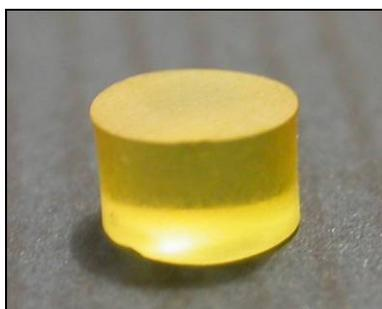
**Figure 63 – Bulk sample obtained heating the xerogel up to 130°C for 1 h**
