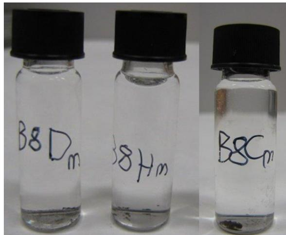
**Figure 3.6.9** Subsamples of the residues of the washing solutions after magnetic separation. B8Dm: sample B2008 washed in DCM (sample on the left); B8Hm: sample B2008 washed in DCM:cyclohexane (1:1 v/v) (sample in the middle); B8Cm: sample B2008 washed in chloroform after 3 minutes ca of ultrasound treatment (sample on the right).
