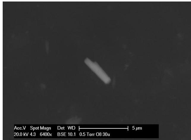
**Figure 4.3.26** SEM micrograph of a zincite particle on a 30 μm nylon membrane through which the residual DCM washing solution used for 2008 needles collected at site O was filtered.
