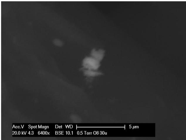
**Figure 4.3.29** SEM micrograph of a barite particle on a 30 µm nylon membrane through which the residual DCM washing solution used for 2008 needles collected at site O was filtered.
