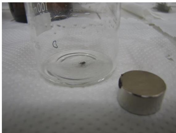
**Figure 3.6.8** The becker after magnetic separation containing on the bottom only the magnetic fraction of the particles washed by DCM from the surface of the needles. On the right the magnet used for separation.
