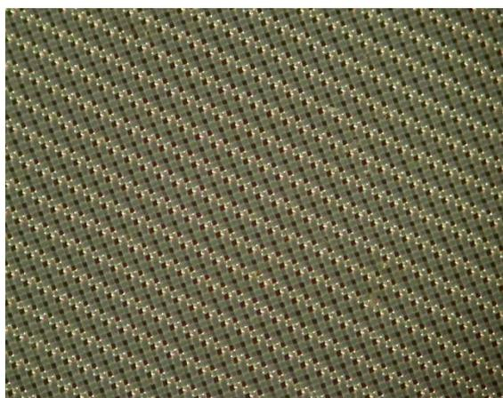
**Figure 2.2.2** Optical microscope image of a woven nylon net filter with 30  $\mu\text{m}$  mesh.
