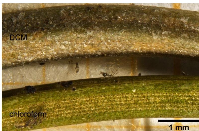
**Figure 3.2.1** OM pictures of the surfaces of washed needles. Top: DCM Bottom: chloroform.
