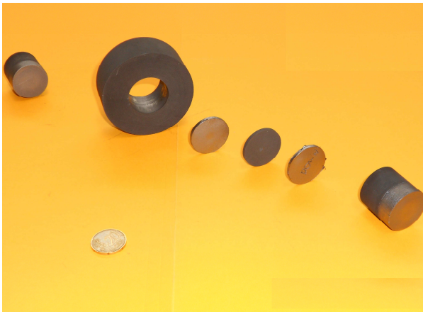
Figure 3.5: Photograph showing the elements constituting the core of the SPS ensemble. From the left, a graphite punch, a graphite die, a laminate sample, a graphite spacer, a laminate sample and a graphite punch are recognizable.
