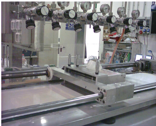
Figure 3.3: Lab-scale apparatus used to cast slurries in the present work.
