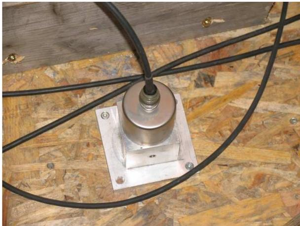
Figure 6.30: Accelerometer
