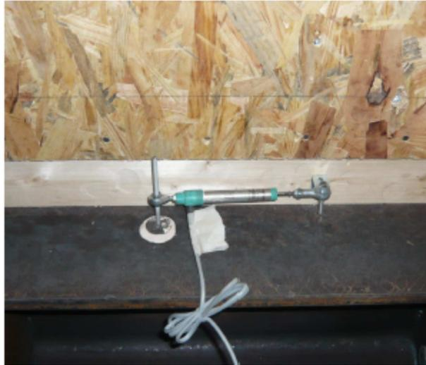
**Figure 6.10:** *LVDT for the measure of the relative displacement of the steel basement and the base timber beam*
