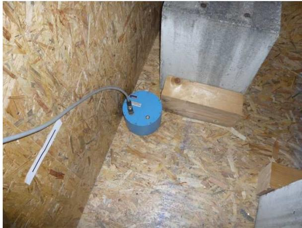
**Figure 6.28:** *Geophones used for the dynamical identification of the structure*
