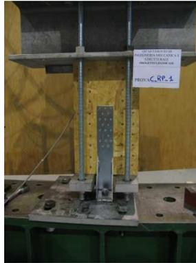
**Figure 1.5:** *Hold Down Load Test*
