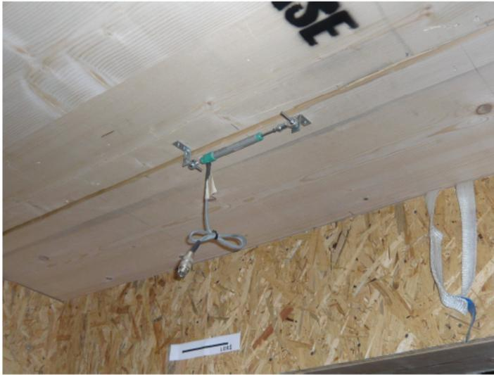
**Figure 6.9:** *Floor box element LVDTs*
