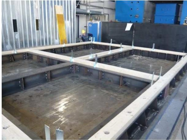
**Figure 6.3:** *Base timber beam and steel basement*
