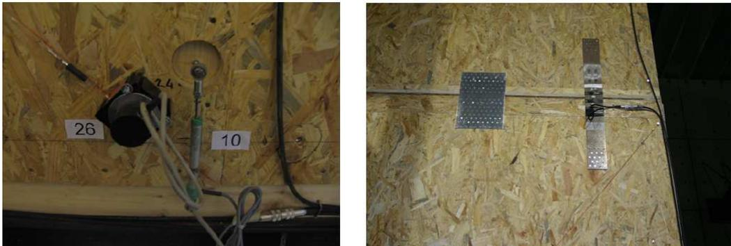
**Figure 6.7:** Wire potentiometers (26), uplift LVDT (10) and Tie-down strain gauges
