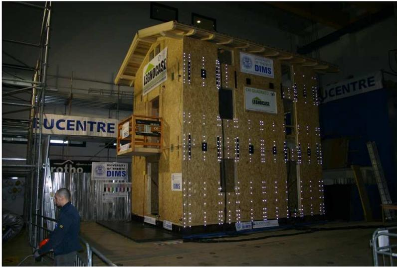
**Figure 6.12:** *Optical system marker arrangement*
