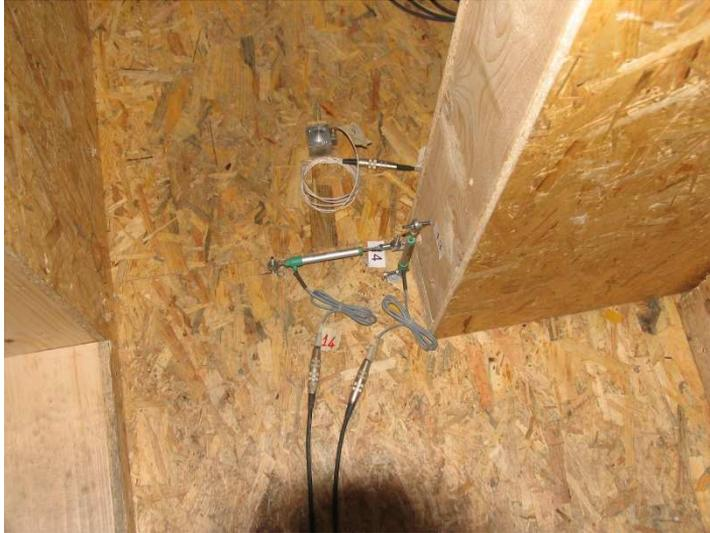
**Figure 6.8:** *Corner uplift and rigid translation LVDTs*
