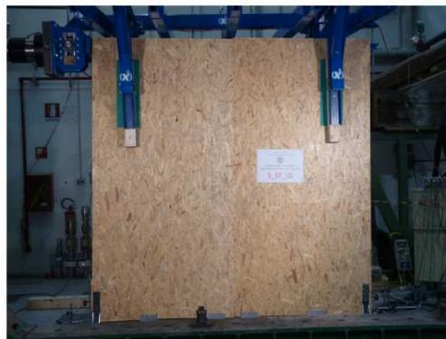
**Figure 1.6:** *Timber Frame Wall Load Test*
