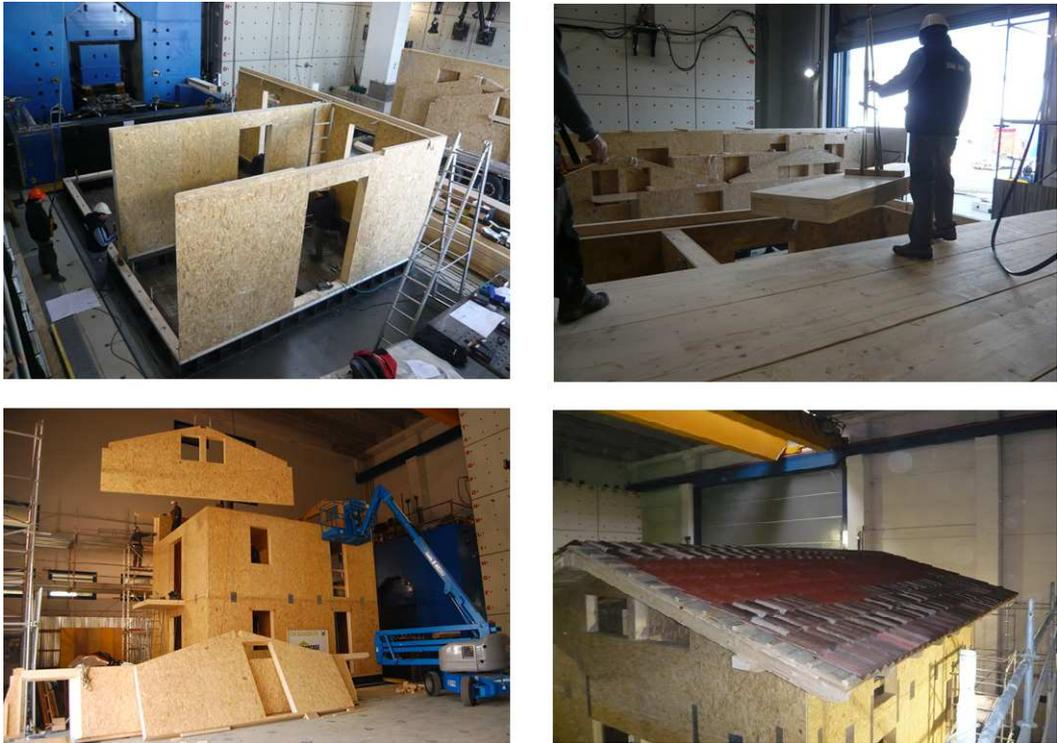
**Figure 6.6:** *Phases of assembly at Eucentre TreesLab*
