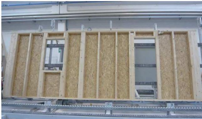
**Figure 2.6:** *Openings in a prefabricated timber-framed wall*
