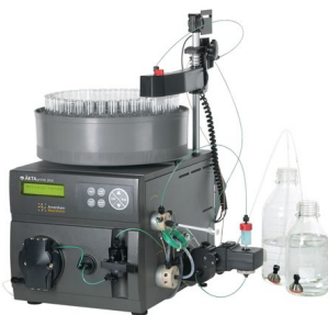
Figure 3.1: AKTA-FPLC system, with in evidence the several fraction collecting tubes
