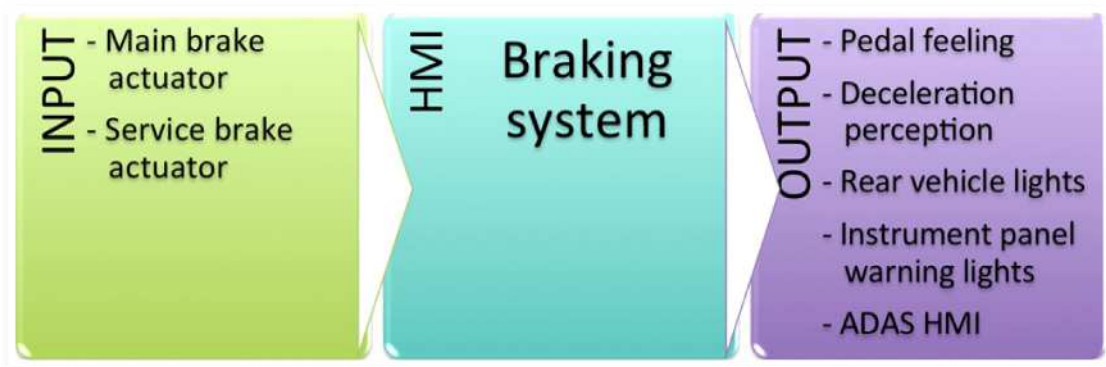
Figure 5: Braking System HMI Input-Output
