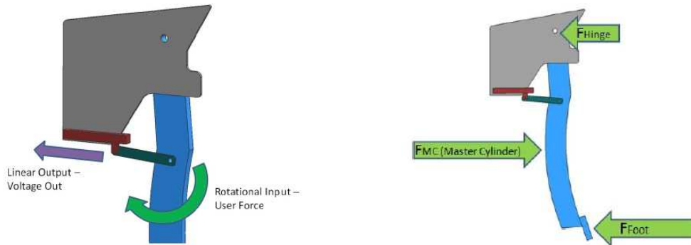
Figure 70: Mount sensor to pedal and back bracket with a four-bar linkage (Pan, 2007).
