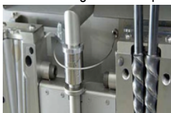
Figure III-10. (a) DSM twin-screw micro-extruder and (b) DSM micro-injection molding unit.
