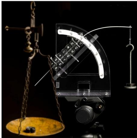
**Figure 1.5:** Scales across millennia: a traditional balance (left) is based on the lever principle, while the innovative elastica arm scale (right) is based on deformation and principles from configurational mechanics. In this particular configuration, the deformable arm scale is working without counterweight.
