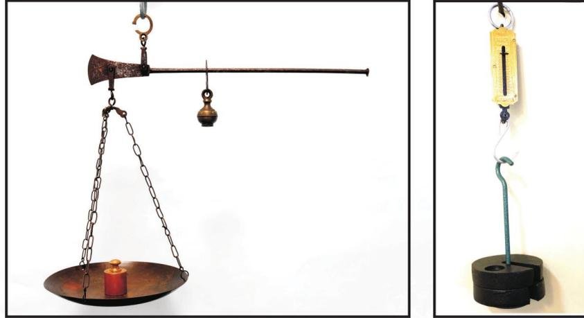
**Figure 6.1:** (Left) A classical steelyard based on rigid lever principle and (right) a spring balance based on deformation.
