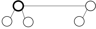
Figure 3.1: Centralized Architecture. All devices form an Environment. A controller (thick circle) manages resources and routings of all devices.
