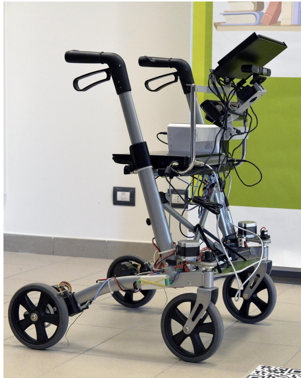
Figure 1.2: The c-Walker is a novel cognitive walking assistant developed within the DALi project. It safely guides the user through complex indoor environments.
