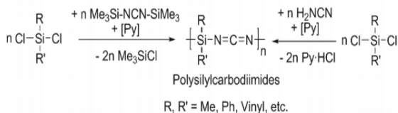
Scheme 6: Carbodiimidolysis and cyanamidolysis of chlorosilanes with bis(trimethylsilyl)carbodiimide and cyanamide.[36]
