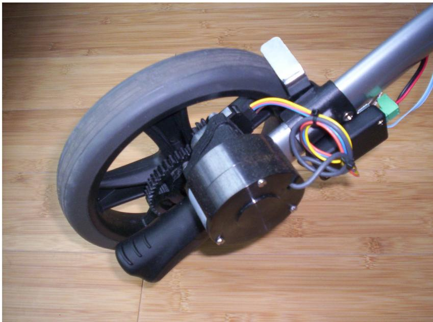
Figure 2.3: Back wheel: CAN bus node, brake and gear of the incremental encoder are visible.
