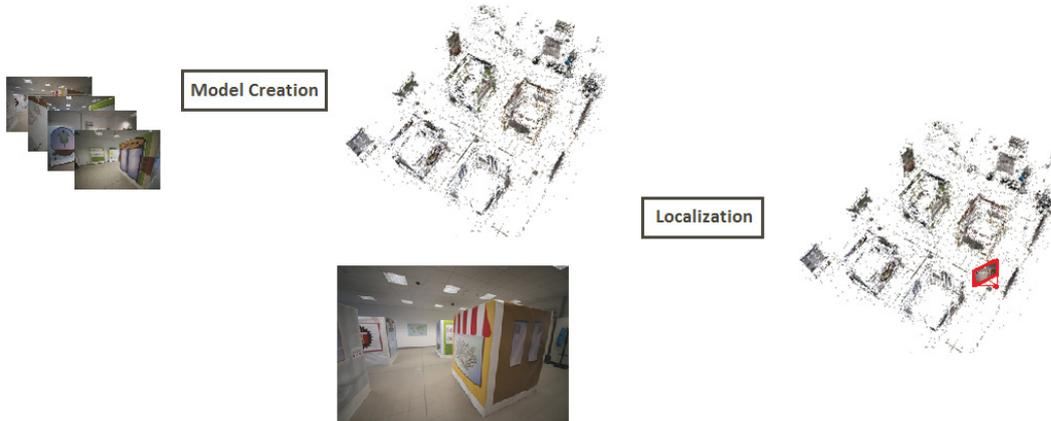
Figure 3.1: Model based Visual Localization Pipeline. Multiple overlapping Images are used to create a synthetic model of the environment. In the localization stage, 2D-3D correspondences are found to compute the camera pose within this model.
