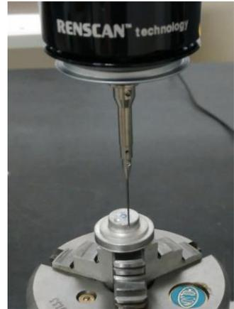
**Figure 53. CMM machine measuring the complete co-sintered component.**
