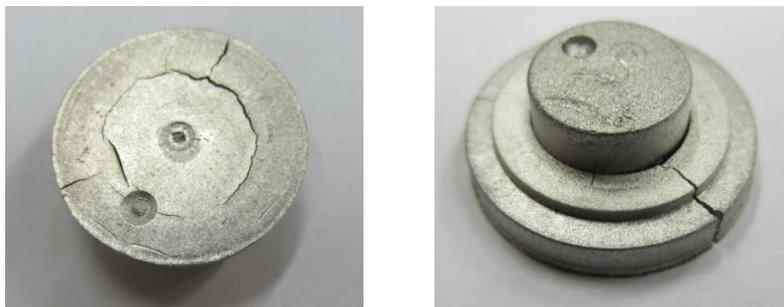
**Figure 33.** The sintered component produced using the two prealloy feedstocks, evident tangential cracks and delamination are visible.
