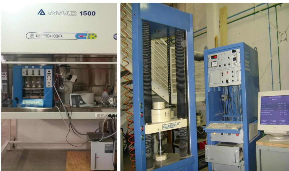
**Figure 2.2:** Soxhlet extractor and rotary evaporator under hood (left) and hydraulic press (right).
