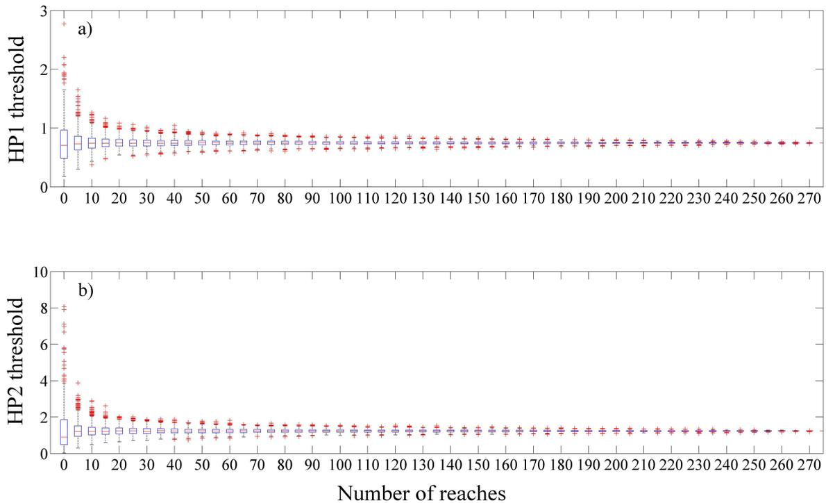
**Figure 2.8:** Threshold for *HP1* (a) and *HP2* (b) calculated on an increasing number of reaches, selected at random. The red line indicates the median, the boxplot the interquartile range and the red cross the extreme values, respectively.
