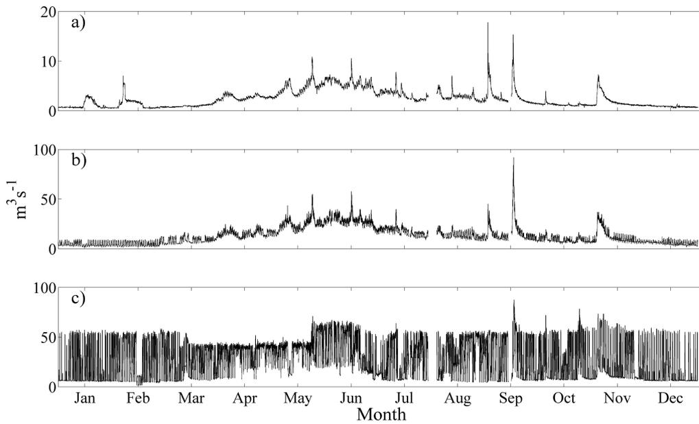
**Figure 1.4:** The hydrograph of a glacial natural Alpine River (a) and of two gauged stations downstream hydropower plant releases (b and c).
