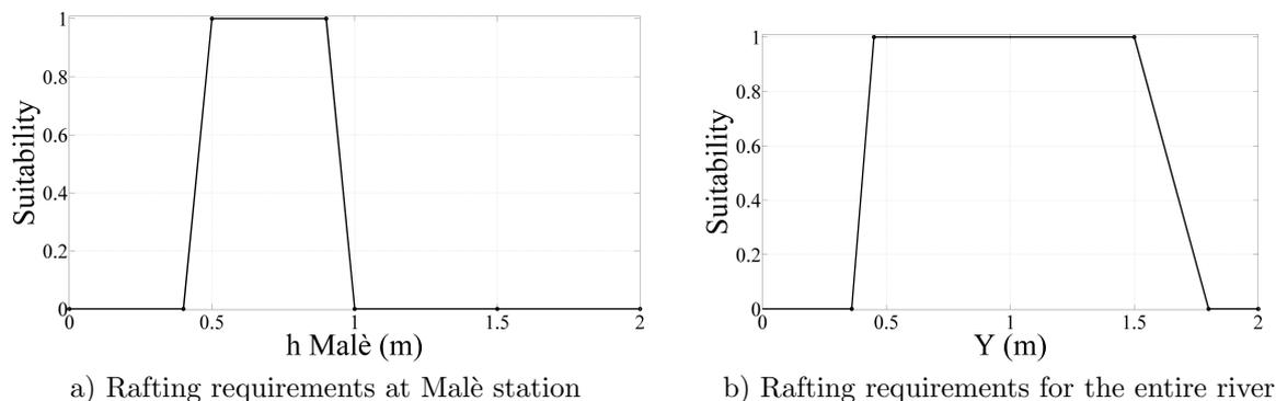
**Figure 4.3:** a) Preference curve for rafting suitability resulting from the interviews with local experts. The controlling hydraulic metric is the water level measured at a reference hydrometric station (Malè for the presented case study). b) Rafting requirements simulated with the hydraulic model as the minimum depth for the lower threshold and maximum depth for the upper threshold in the reference reach corresponding to the water level at the Malè section.
