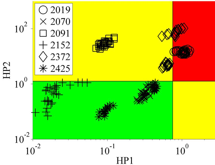
**Figure 2.9:** Distribution of six stations used as control group. The displayed thresholds are the global thresholds. Different groups are denoted with cross (unpeaked) and circles (peaked). The four regions identify the three different classes of hydropeaking pressure: class 1 (absent or low pressure, green colour, left bottom); classes 2a and 2b (moderate pressure, yellow colour, right bottom and left top respectively) and class 3 (high pressure, red colour, right top).
