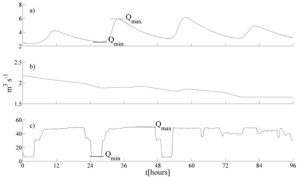
**Figure 1.5:** Daily hydrograph of a) a natural river, b) a lake emissary and c) a river impacted by hydropeaking.
