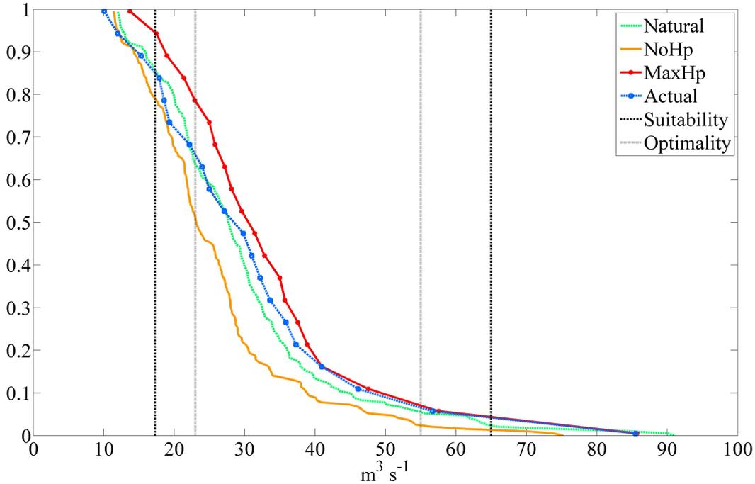
**Figure 4.8:** Example of the duration curves and thresholds relative to the fourth reach. Four flow patterns are represented here: dotted green line is the *Nat* pattern, orange line is the *NoHp* pattern, red line is the *MaxHp* pattern and blue dotted line is the *Act* pattern. Dotted black and grey lines are the thresholds of suitability and optimality, respectively.
