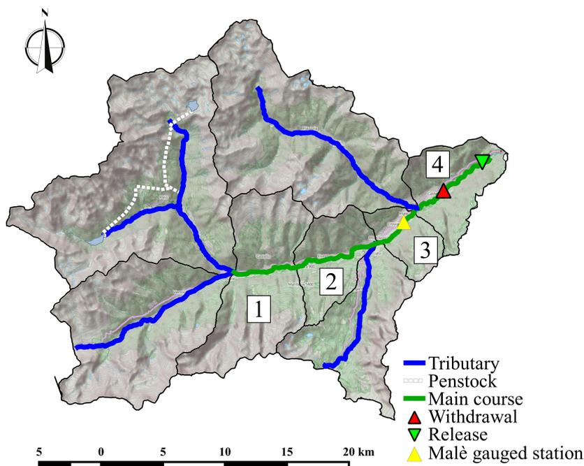
**Figure 4.1:** Map of the Upper Noce River catchment where the study reach is located. The blue lines denote tributaries, the dotted line indicates the penstock, the green line points out the studied reach, the numbers indicate the sub basin in which the area is divided, the red and green triangles denote uptake and release respectively and the yellow triangle indicates the river main gauging station.
