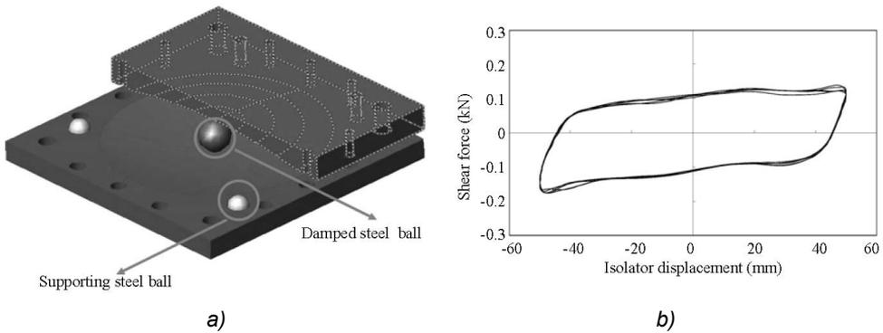
Fig. 2.26 a) Exploded perspective view of SDI-BPS device; b) related force-displacement hysteresis loop (from Tsai et al., 2010).
