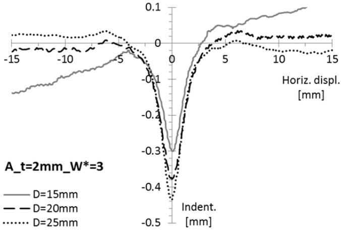
Fig. 6.41 Comparison of the geometric profiles of the residual indentation for the case of rubber A,  $t=2\text{mm}$ ,  $W^*=3$ , for different values of the ball diameter ( $D=15, 20, 25$ ).
