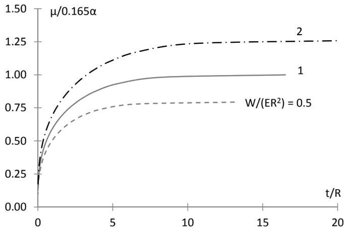
Fig. 3.14 New calculation of the theoretical plots of rolling friction ratio  $\mu$ , scaled using  $\alpha$ , versus dimensionless ratio of rubber layer thickness to ball radius (Eqs. (3.28),(3.16)).  $W/ER^2$  is the stress parameter.
