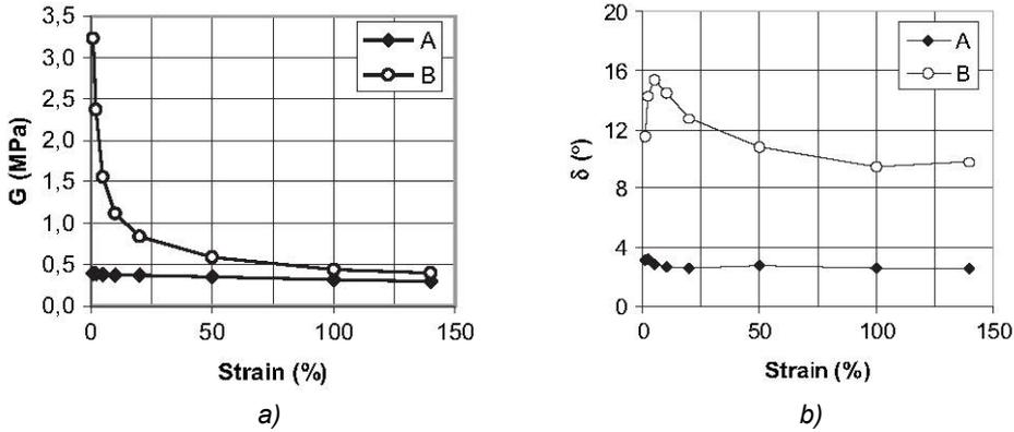
Fig. 3.22 Dynamic shear properties of rubbers A (unfilled) and B (filled) used for the RBRL devices in the ECOEST project. Rubber B shows Payne effect (from Guerreiro et al., 2007).
