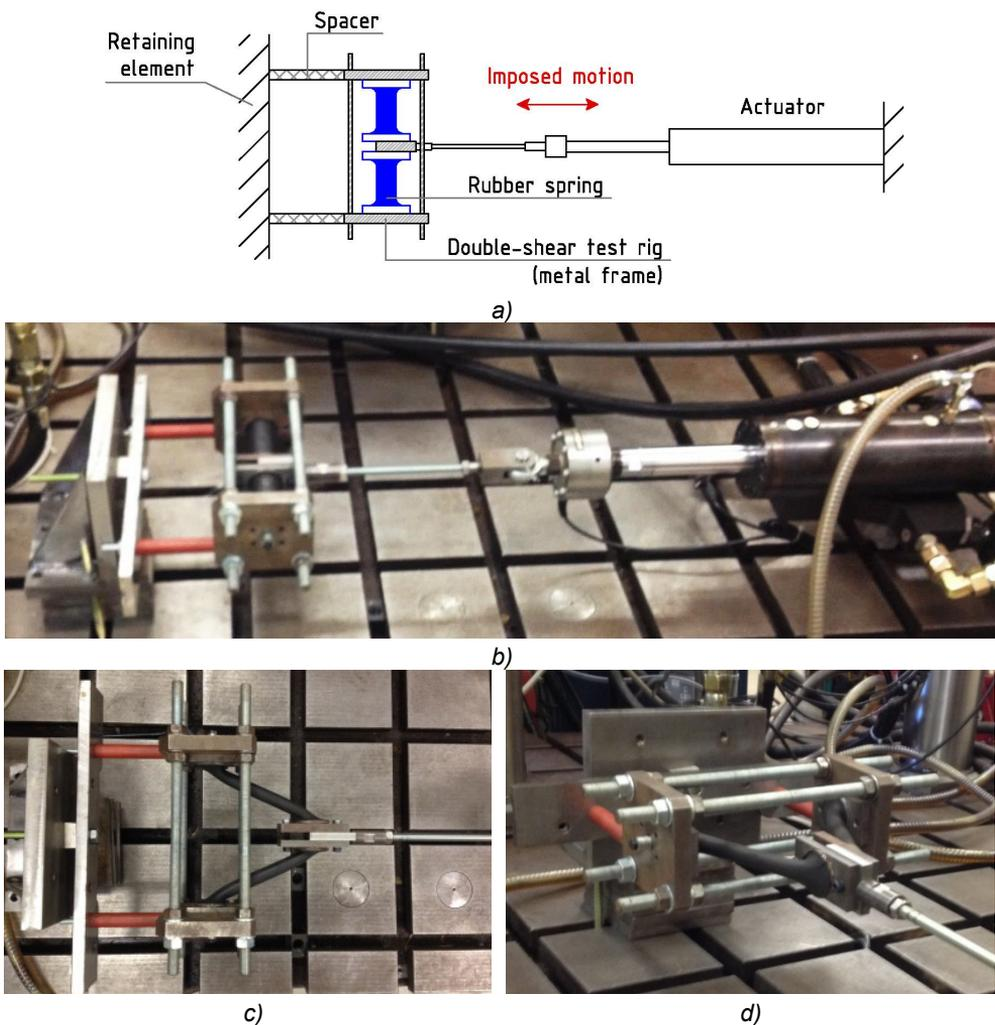
Fig. 5.23 a) Schematic drawing and b) image of the double shear test setup for the behaviour characterization of the recentering rubber springs. c),d) Images from quasi-static test for spring  $\phi 30$  at 150 mm of deflection.
