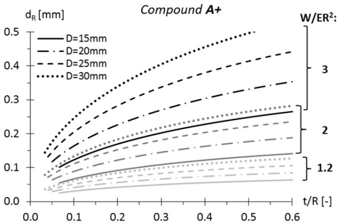
Fig. 6.55 Estimate of the maximum residual indentation  $d_R$  through the Eq. (6.12), after a dwell time of the load of 25 hours, for the rubber A+ and for a certain range of  $t/R$  and  $W/ER^2$ .
