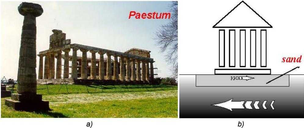
Fig. 1.1 a) Image of the Temple of Paestum in Capaccio (III c. BC). b) Scheme of the mechanism to protect the Temple by the earthquake: base of sand and gravel inserted between the foundation and the ground (image from Martelli, 2010).
