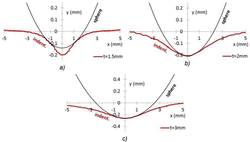
Fig. 6.40 Geometric profiles of Fig. 6.39 with the indication of the relative indenter.
