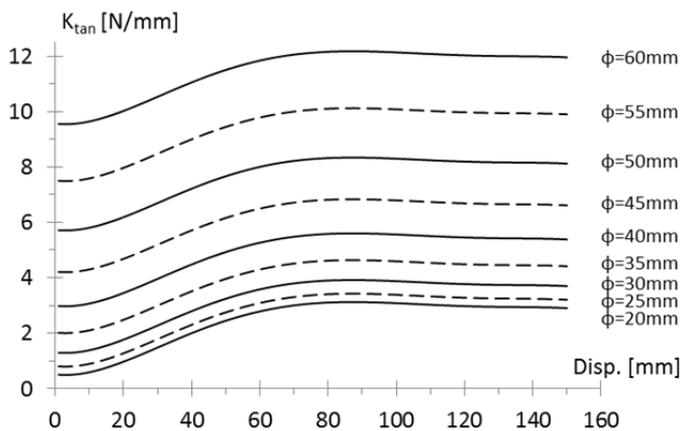
Fig. 6.83 Prediction of the tangent stiffness  $K_{tan}$  values using Eq. (5.15), proposed again in Eq.(6.21), for different diameters of the spring: 30, 40 and 50 mm.
