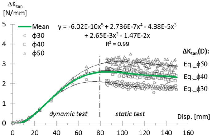
Fig. 5.34 Nonlinear dependence of the tangent stiffness  $K_{tan}$  of the springs on deflection.
