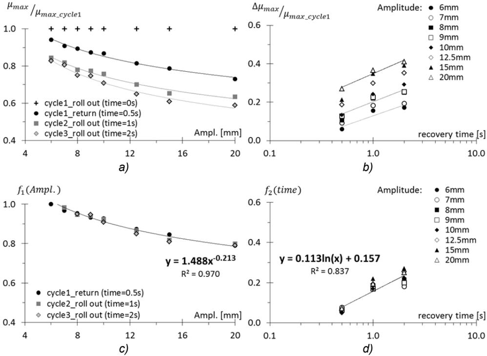
Fig. 6.78 a), b) Effects of the recovery of the rubber on the maximum rolling friction  $\mu_{max}$  due to the roll-out of the balls from their pits. c), d) Interpolating equations for the functions  $f_1(Ampl.)$  and  $f_2(time)$  necessary to apply the equation Eq. (6.20).
