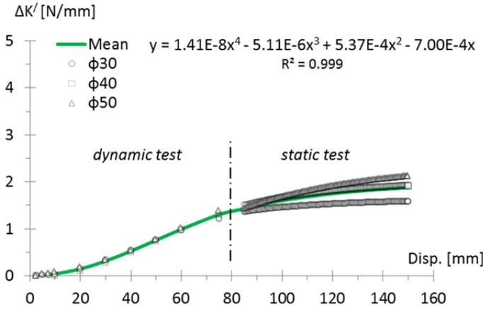
Fig. 5.32 Nonlinear dependence of the stiffness  $K'$  on deflection. Values obtained by the ones of Fig. 5.31 subtracting the initial values of stiffness  $K'$  associated with each diameter.
