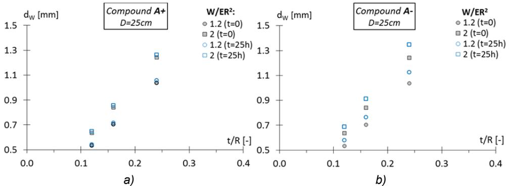
Fig. 6.51 Maximum indentations under load given by Waters' equations (Eqs. (6.6) and (6.7)), considering the Young's modulus ( $t=0$ ) and the one relaxed after 25 hours ( $t=25h$ ), for different values of  $t/R$  and  $W/ER^2$ , and for the case of rubber A+ (a) and A- (b).
