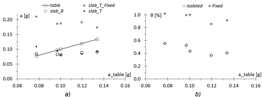
Fig. 4.8 As Fig. 4.4, for EC8(02) different-scaled earthquakes ( $K = -12, -9, -9, -7, -6$  dB). For these tests a combination of rolling tracks A (low damping) – B (high damping) was used.
