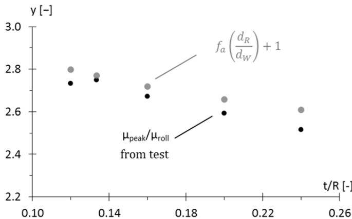
Fig. 6.69 Comparison that shows the same dependence of the ratio  $\mu_{peak}/\mu_{roll}$  and of the function  $f_a$  (shown in Fig. 6.66) on the parameter  $t/R$ .
