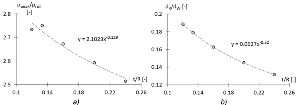
Fig. 6.64 Same dependence of the ratio  $\mu_{peak}/\mu_{roll}$  (a) and  $d_R/d_W$  (b) on the parameter  $t/R$ . The values of  $\mu_{peak}$  were obtained by sinusoidal tests performed with same  $W/ER^2$  and rubber A, presented in section 6.2.
