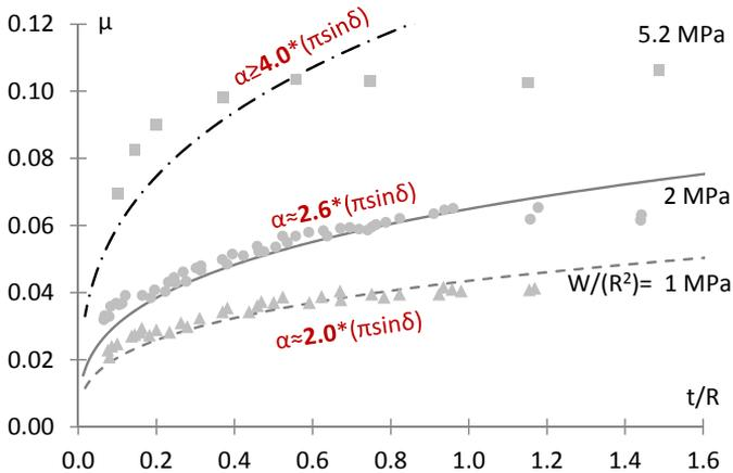
Fig. 3.16 Comparison between the predicted values of  $\mu$  (lines), by theory of Muhr et al. (1997), and the experimental data (dots), reported here through the digitalization of Fig. 3.11.  $\alpha$  value to get the best fitting is reported for each stress level ( $W/R^2$ ) considered.
