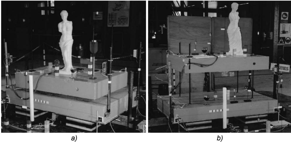
Fig. 4.1 a) View of the two test set-ups used in the ECOEST experimentation: a) Mass Down and b) Mass Up configuration (from Guerreiro et al., 2007).
