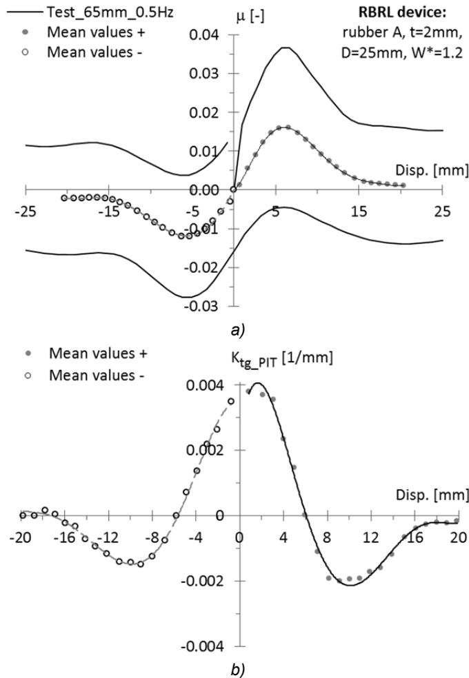
Fig. 6.84 a) Non-linear elastic behaviour for the presence of the initial depression under the ball. b) Tangent stiffness calculated from the non-linear  $\mu$ -disp behaviour of plot a). Results from a sinusoidal test performed at 65 mm amplitude and 0.5 Hz frequency, on the RBRL device assumed as reference (A, t=2mm, D=25mm, W\*=1.2).
