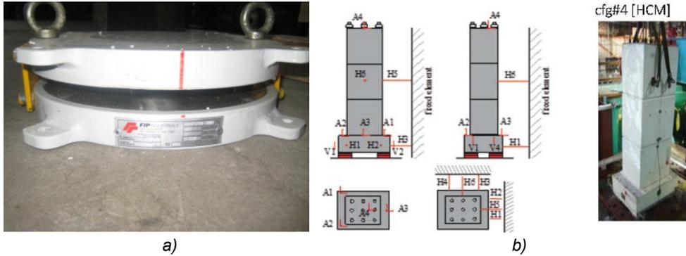
Fig. 2.21 a) DCCSS isolator. b) Setup used for shaking table tests (from Berto et al., 2013).
