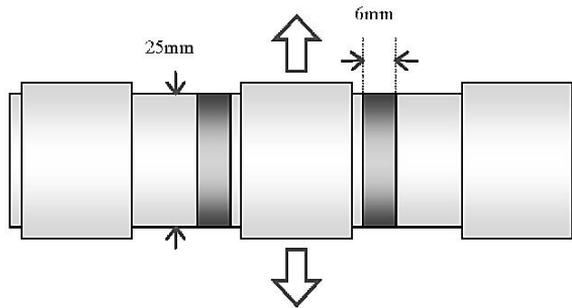
Fig. 5.2 Cylindrical double shear test piece that shows the nominal thickness of the rubber disc (darker colour) sandwiched between three metal pieces (from Ahmadi et al., 2008).
