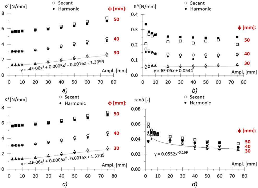
Fig. 5.27 ELVFD parameters from sinusoidal tests at the same frequency, 1 Hz. Comparison between the Harmonic and Secant linearization methods. Values for one spring.
