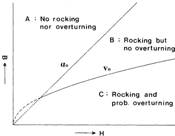
Fig. 2.9 Overturning criteria for rigid bodies (from Ishiyama, 1984).
