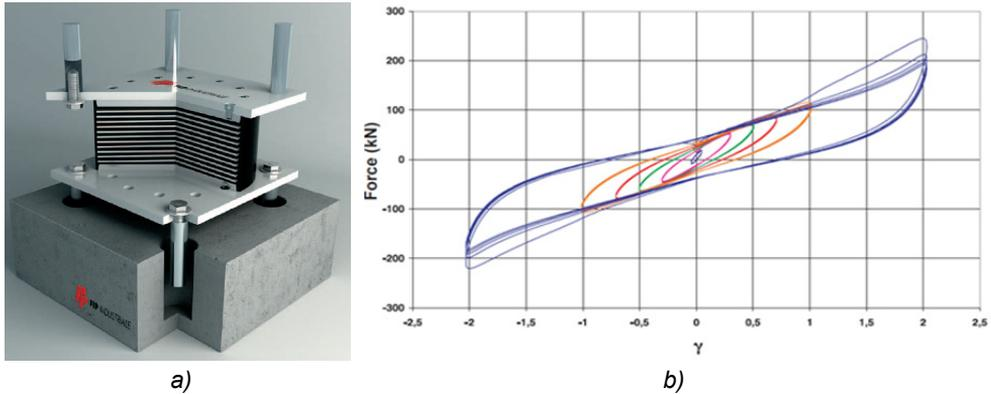
Fig. 2.14 a) Image of a High Damping Rubber Bearing (HDRB). b) Typical hysteresis loops of a HDRB isolator obtained by dynamic tests at increasing shear strain amplitude  $\gamma$  (from FIP Industriale S.p.A., 2015).
