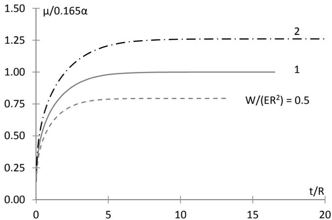
Fig. 3.18 Theoretical plots of rolling friction ratio  $\mu$ , scaled using  $\alpha$ , versus dimensionless ratio of rubber layer thickness to ball radius (Eqs. (3.28), (3.16)), for lubricated condition.  $W/ER^2$  is the stress parameter.
