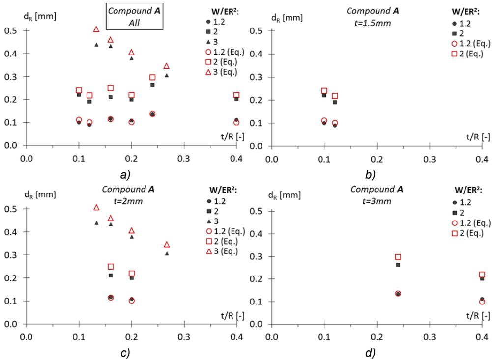
Fig. 6.52 a) Comparisons between test results and values calculated by Eq. (6.12) for the maximum residual indentation, for the case of rubber A and different values of  $t/R$  and  $W/ER^2$ . The same results are reproduced in the figures b), c), d) for the different values of rubber layer thickness analyzed.
