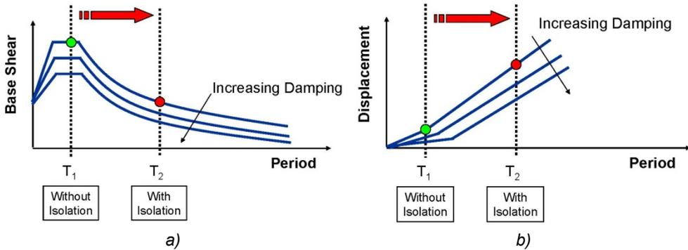
Fig. 2.10 Effects of the seismic isolation in terms of spectral acceleration (a) and displacement (b) (from Symans, 2004).
