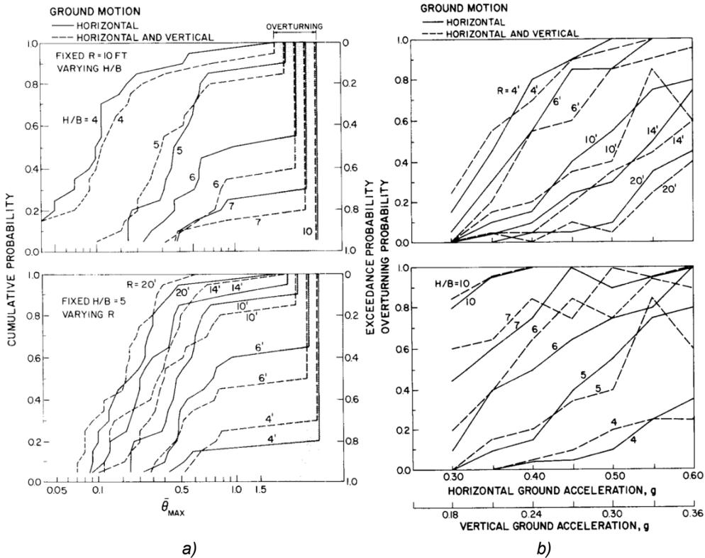
Fig. 2.8 a) Cumulative probability distribution functions for maximum rotation  $\theta_{MAX}$ . b) Overturning probability. Different values of R and H/B investigated, for rigid blocks subjected to an ensemble of horizontal and vertical ground motion. (Yim et al., 1980).
