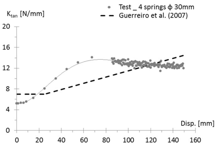
Fig. 5.36 Tangent stiffness calculated by the experimental results, compared with the one proposed in the Guerreiro et al. (2007) Model for the RBRL device, relatively to the recentering springs system used in the ECOEST Project (4 spring, diameter 30 mm).
