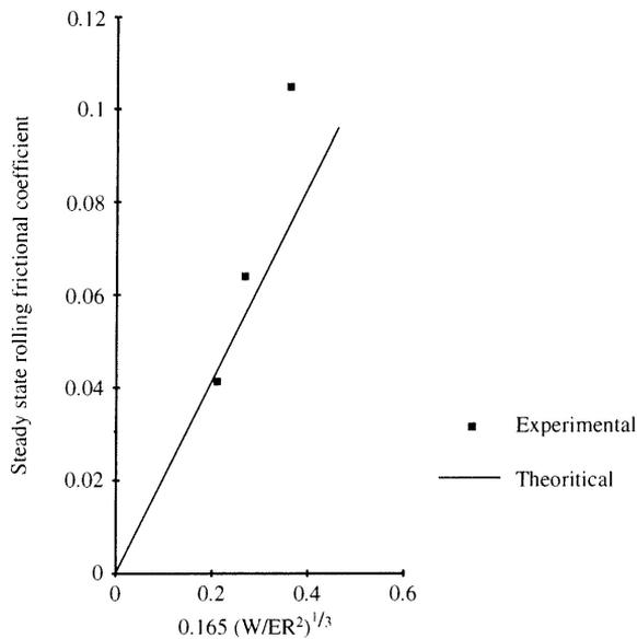
Fig. 3.12 Comparison of theory for the plateau value of  $\mu$  (Eq. (3.16)) with experimental results, for steady-state rolling resistance as a function of load (Muhr et al., 1997).
