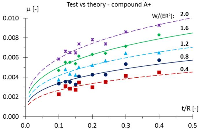
Fig. 5.16 Comparison, for the compound A+, of the rolling friction values ( $\mu$ ) obtained by the tests and the theory, for different thickness/radius ratios ( $t/R$ ) and stress parameters ( $W/ER^2$ ).
