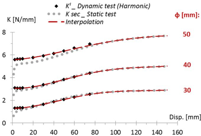
Fig. 5.31 Comparison between the storage stiffness  $K'$ , from dynamic tests, and the secant one  $K_{sec}$ , from quasi-static tests. The stiffness finally considered derives from  $K'$  values until 75 mm, and from  $K_{sec}$  values for higher deflections (as indicated by the dashed lines).
