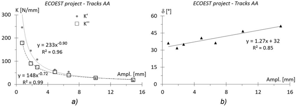
Fig. 4.9 Equivalent linear viscoelastic parameters obtained from ECOEST sinusoidal tests at 5Hz: a)  $K'$   $K''$ , b)  $\delta$ .
