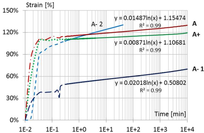
Fig. 5.8 Creep plots for all the specimens tested.
