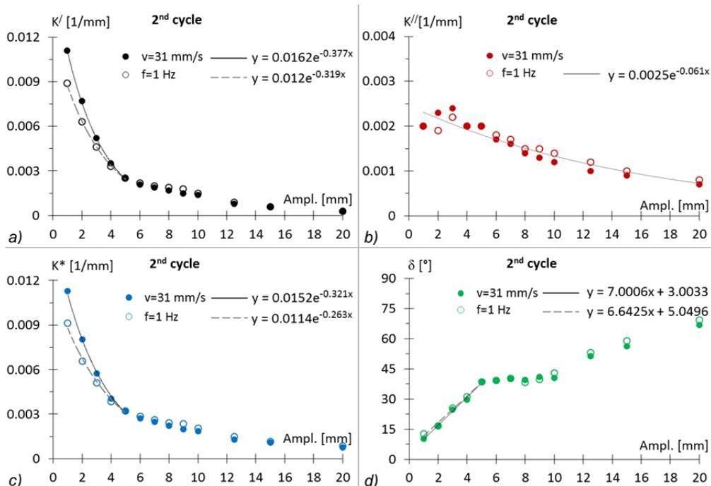
Fig. 6.19  $K'$ ,  $K''$ ,  $K^*$ ,  $\delta$  vs amplitude. Rubber A,  $t=2$ mm,  $D=25$ mm,  $W/ER^2=1.2$ , 2<sup>nd</sup> cycle.
