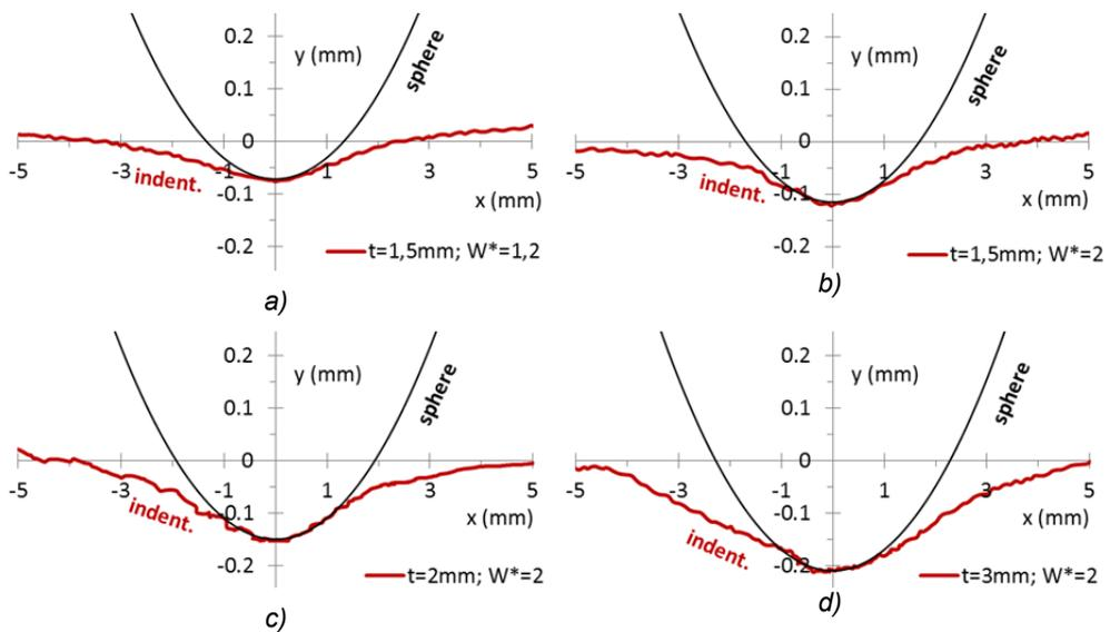
Fig. 6.44 Geometric profiles of Fig. 6.43 with the indication of the relative indenter.
