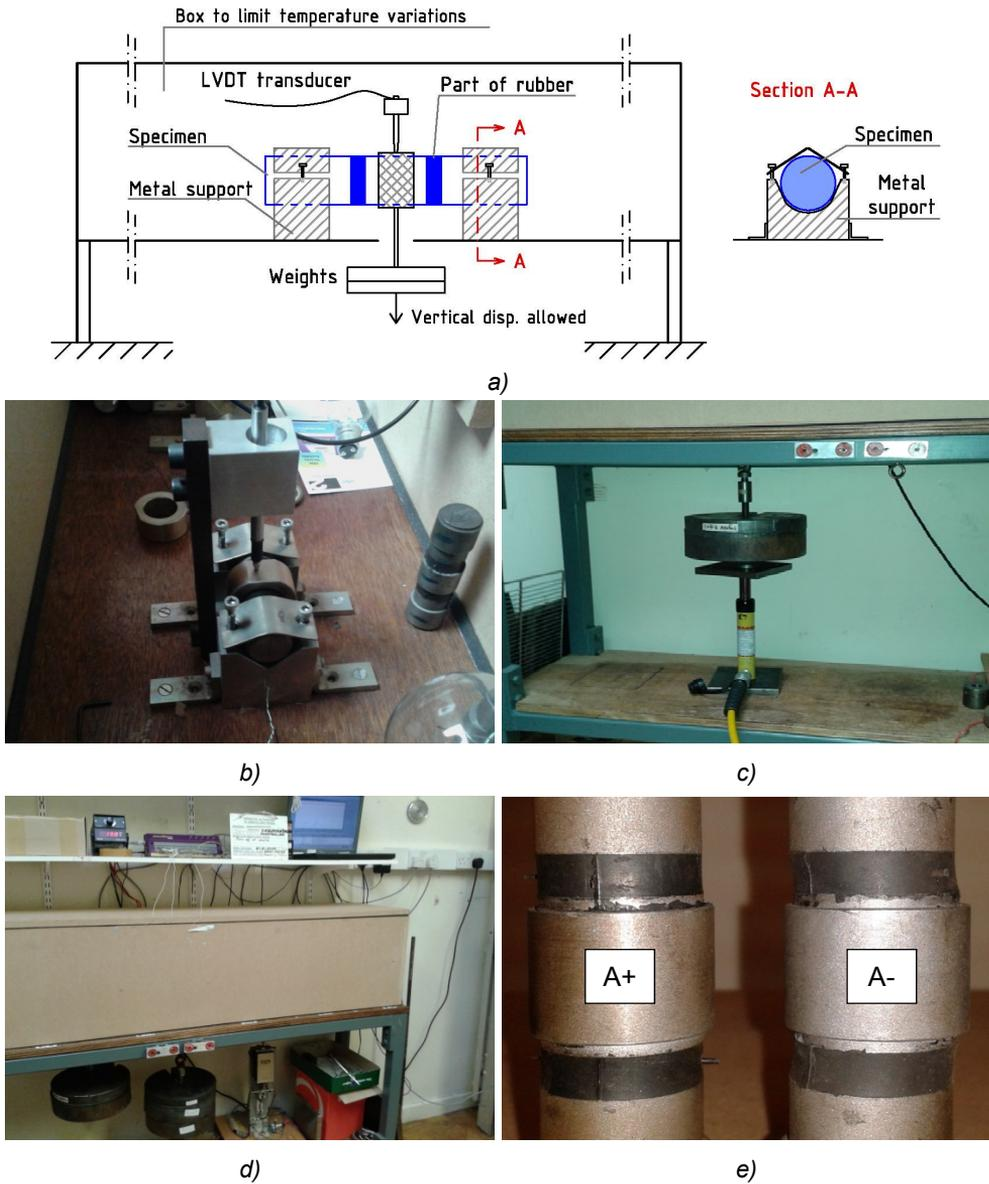
Fig. 5.7 a) Schematic drawing of the creep test setup; b) installation of the test piece (view of the LVDT transducer); c) application of the load through an hydraulic jack minimizing the load oscillations; d) general view of the setup during the creep tests; e) comparison of the residual strain, between specimens A+ and A-, just finished the test.
