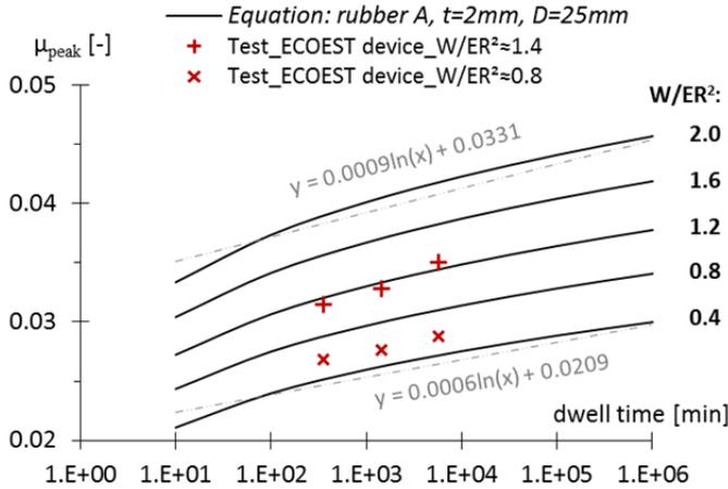
Fig. 6.70 Dependence of the estimated values of  $\mu_{peak}$  on the load dwell time, according to Eq.(6.18), for different stress levels and for the case of rubber A,  $t = 2$  mm and  $D = 25$  mm. Overlap of the  $\mu_{peak}$  values gathered by the sinusoidal tests presented in section 6.4 on the associated ECOEST device (A,  $t = 2$  mm,  $D = 25$  mm).
