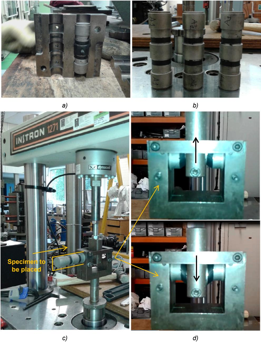
Fig. 5.3 a) Production of the test pieces for the rubber characterization. b) View of the three test pieces used in the double shear tests. c) Test setup using Instron 1271 servo hydraulic test machine (the specimen is not yet placed in the loading rig). d) Images from test execution.
