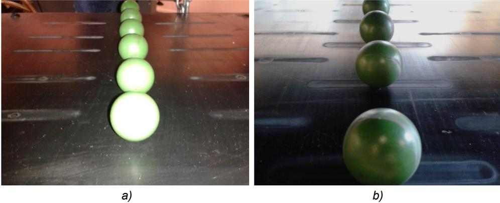
Fig. 6.60 Semi-permanent rolling tracks on the rubber layer B. Case B-B,  $t_{dw}=24$  h,  $W=250$  N: a) before the test (the semi-permanent rolling tracks visible derive from the previous test with  $W=150$  N); b) after the test.
