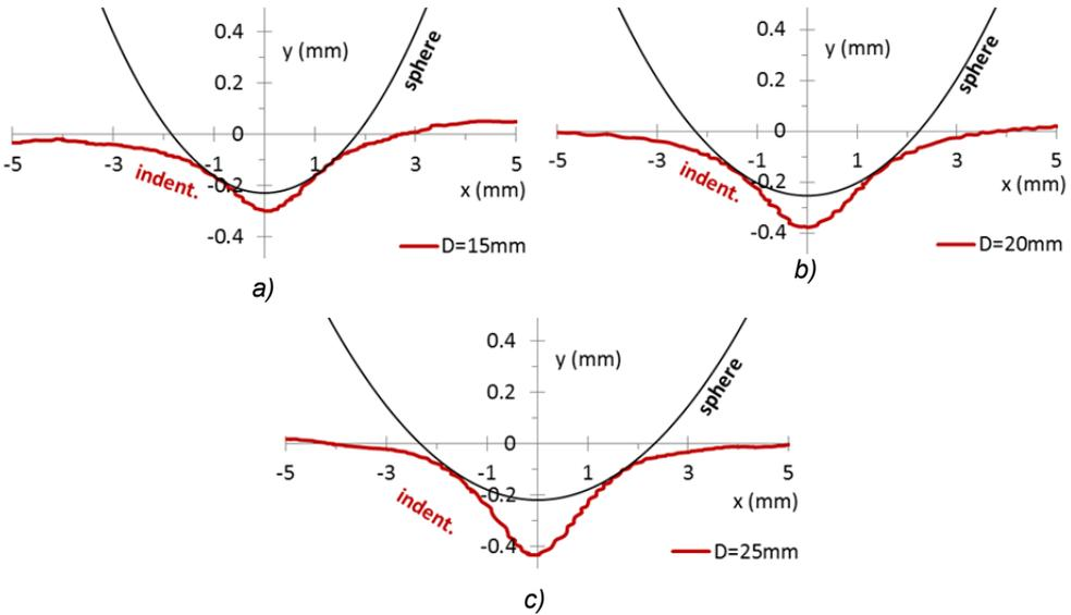
Fig. 6.42 Geometric profiles of Fig. 6.41 with the indication of the relative indenters.
