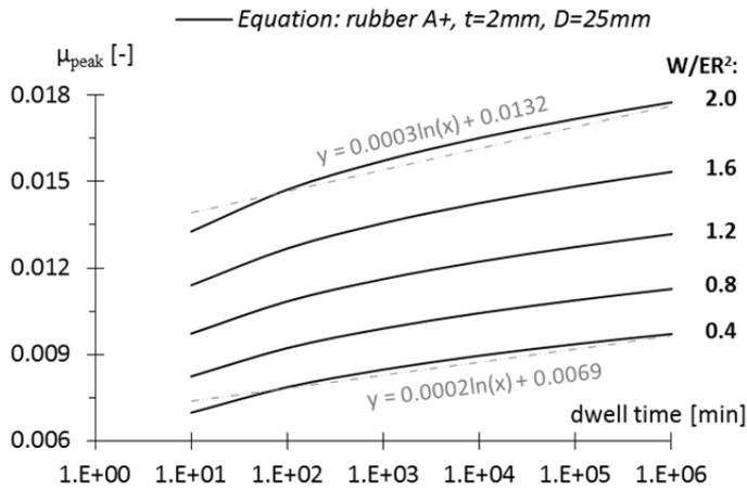
Fig. 6.72 Dependence of the estimated values of  $\mu_{peak}$  on the load dwell time, according to Eq.(6.18), for different stress levels and for the case of rubber A+,  $t = 2$  mm and  $D = 25$  mm.
