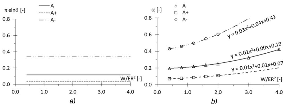
Fig. 5.21 a) Values of the hysteretic parameter  $\alpha$  considering the classic definition:  $\alpha = \pi \sin \delta$ . b)  $\alpha$  values calibrated from tests to have the best fitting with the theory (Eq. (5.5)).
