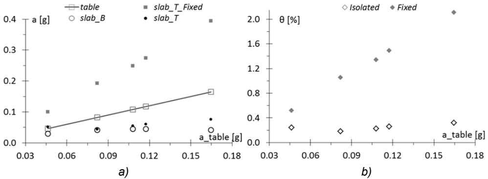
Fig. 4.4 a) Top(“T”)–bottom(“B”) slab accelerations  $a$  [g] and b) drifts  $\theta$  [%] between the two slabs versus peak table acceleration from ECOEST results, for the isolated-base case, compared with the simulated fixed-base case (“Fixed”) ( $\approx$  sliding isolator for small seismic intensity), for Northridge\_PCKC different-scaled earthquakes ( $K = -12, -6, -4, -3, 0$  dB).
