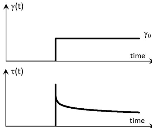
Fig. 3.21 Stress response  $\tau(t)$  to an initial constant strain  $\gamma_0$  for a viscoelastic material.
