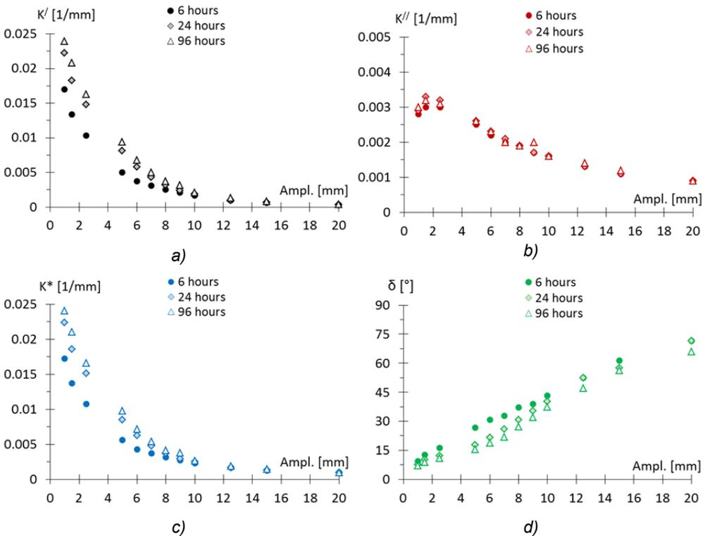
Fig. 6.61 Comparison of  $K'$ ,  $K''$ ,  $K^*$ ,  $\delta$  vs amplitude, for the different dwell times of the load considered: 6, 24 and 96 hours. Case: tracks A-A,  $W = 250$  N, max. vel. = 31 mm/s, 2<sup>nd</sup> cycle.
