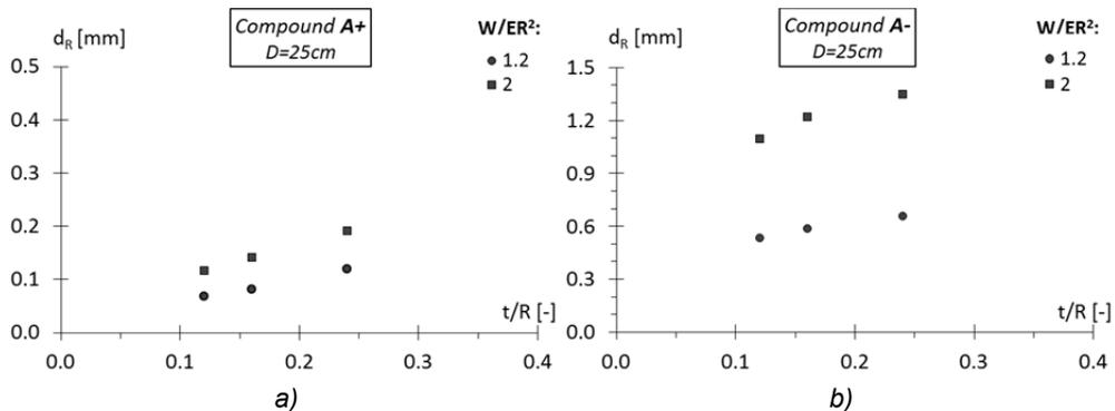
Fig. 6.49 Maximum residual indentations by tests, after a dwell time of the load of 25 hours, for different values of  $t/R$  and  $W/ER^2$ , and for the case of rubber A+ (a) and A- (b).
