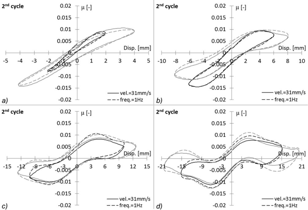
Fig. 6.12 Comparisons of  $\mu$ -disp loops-2<sup>nd</sup> cycle. Rubber A+,  $t=2\text{mm}$ ,  $D=25\text{mm}$ ,  $W/ER^2=1.2$ .
