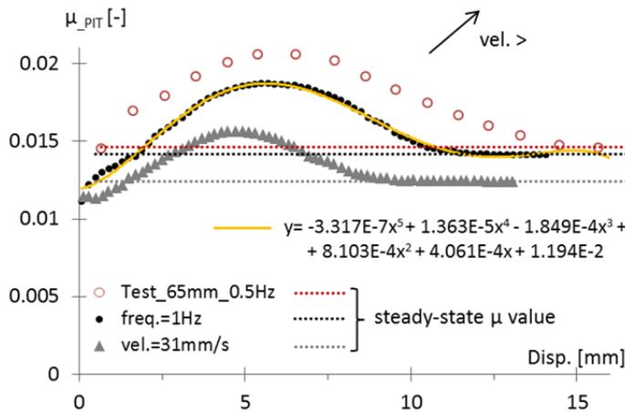
Fig. 6.87 Influence of the pits on the rolling friction resistance for small displacements of the balls. Test at 65 mm and 0.5 Hz, on the reference RBRL device.
