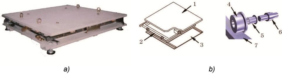
Fig. 2.19 Roller-Type Isolation Device: a) image; b) schematic drawing (from Ueda et al., 2004).
