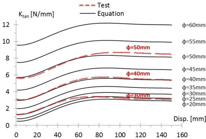
Fig. 5.35 Prediction of the tangent stiffness values  $K_{tan}$ , using Eq. (5.15), and comparison with the experimental values for the diameters 30, 40 and 50 mm.
