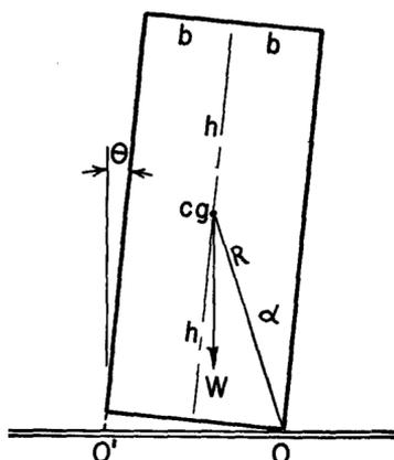
Fig. 2.7 Representation of the rocking phenomena for a slender rigid block (Housner, 1963).
