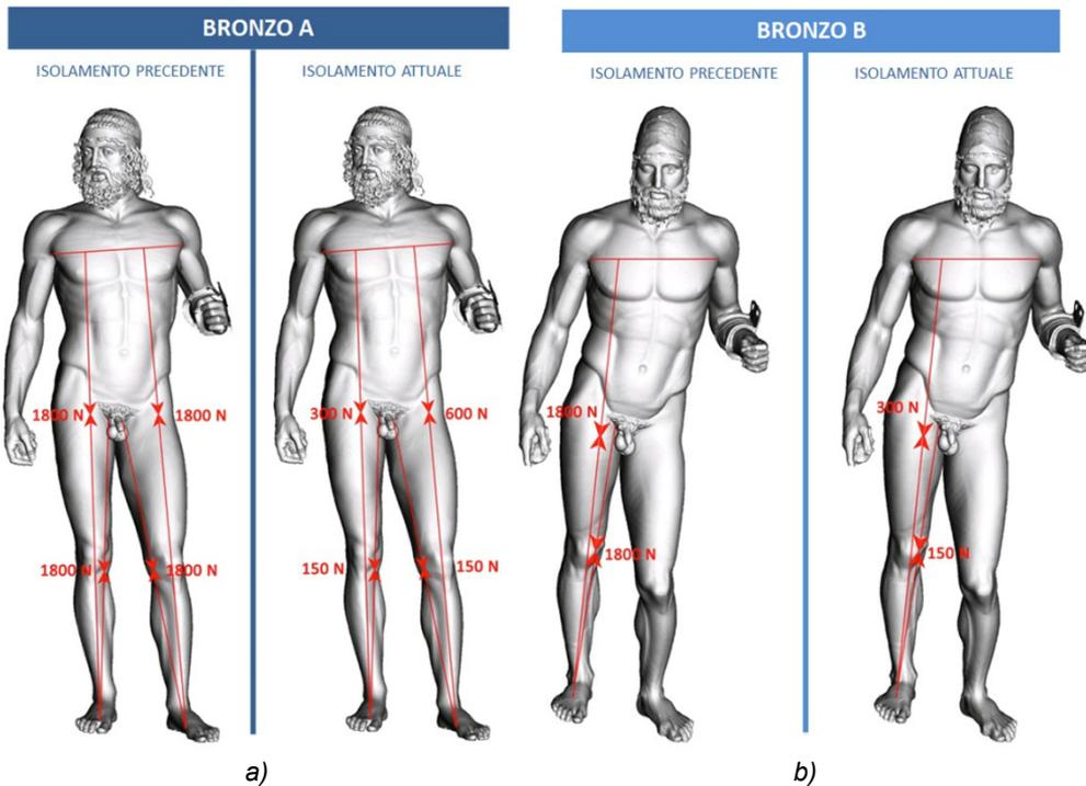
Fig. 2.30 a) Forces acting in the internal anchoring cables, before and after the installation of the new isolation system: a) “Bronzo A”, the “Young”; b) “Bronzo B”, the “Old” (from De Canio & Modena, 2013).
