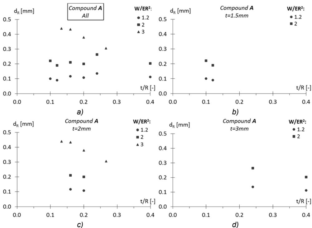
Fig. 6.48 a) Maximum residual indentations by tests, after a dwell time of the load of 25 hours, for the case of rubber A and different values of  $t/R$  and  $W/ER^2$ . The same results are reproduced in the figures b), c), d) for the different values of rubber layer thickness analyzed.
