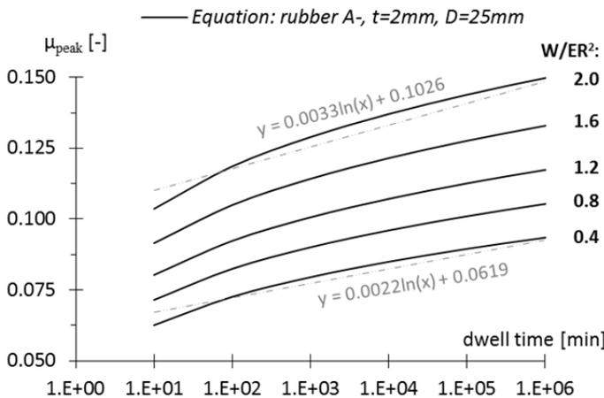
Fig. 6.71 Dependence of the estimated values of  $\mu_{peak}$  on the load dwell time, according to Eq.(6.18), for different stress levels and for the case of rubber A-,  $t = 2$  mm and  $D = 25$  mm.
