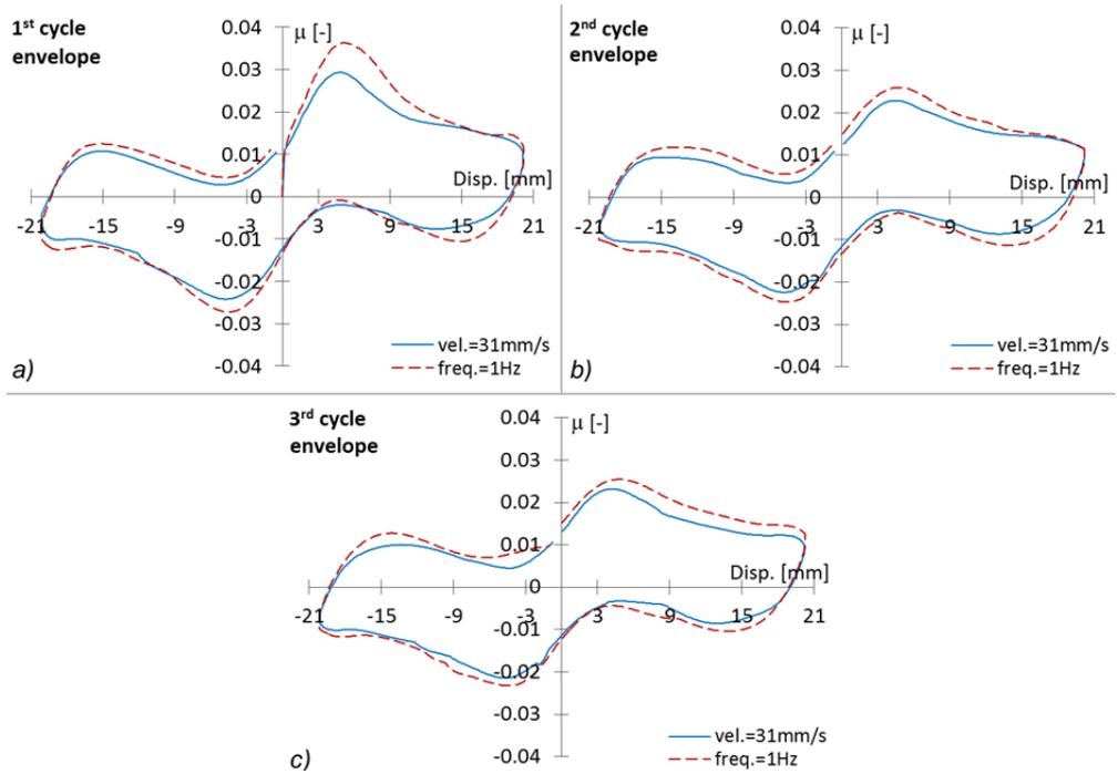
Fig. 6.3 Envelopes of  $\mu$ -disp loops. Rubber A,  $t=2\text{mm}$ ,  $D=25\text{mm}$ ,  $W/ER^2=1.2$ .
