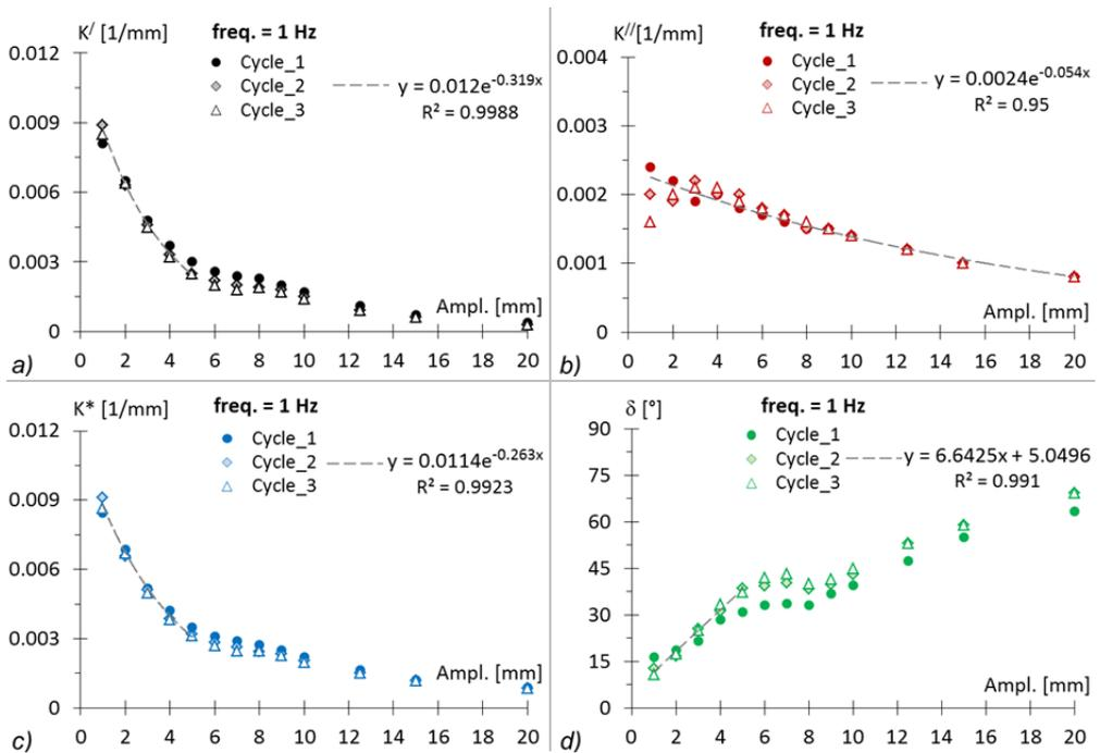
Fig. 6.17  $K'$ ,  $K''$ ,  $K^*$ ,  $\delta$  vs ampl. Rubber A,  $t=2\text{mm}$ ,  $D=25\text{mm}$ ,  $W/ER^2=1.2$ , constant frequency
