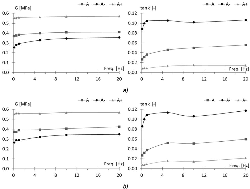
Fig. 5.5 Dynamic shear properties of rubber compounds (A, A+,A-) by Harmonic (a) and Secant (b) linearization method – influence of frequency for a 5% strain.
