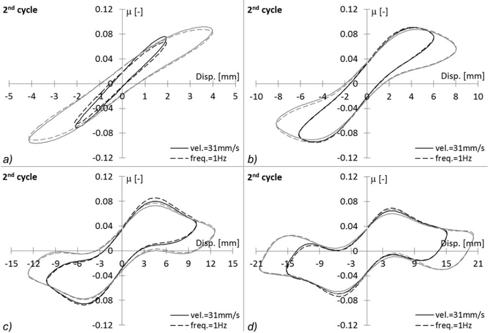
Fig. 6.15 Comparisons of  $\mu$ -disp loops-2<sup>nd</sup> cycle. Rubber A-,  $t=2\text{mm}$ ,  $D=25\text{mm}$ ,  $W/ER^2=1.2$ .
