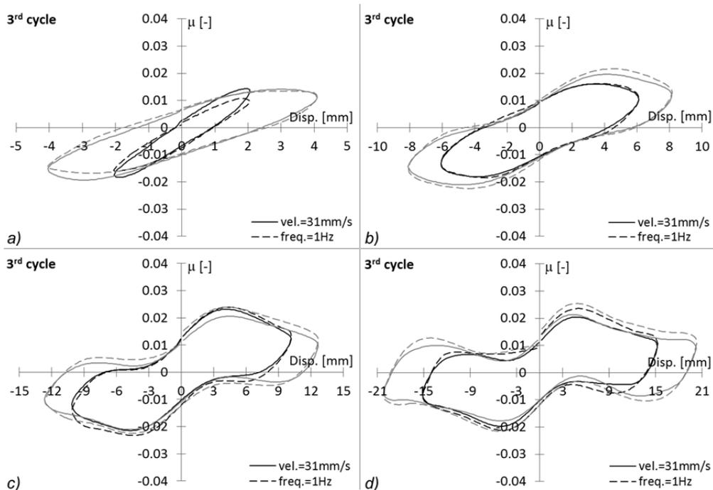
Fig. 6.6 Comparisons of  $\mu$ -disp loops - 3<sup>rd</sup> cycle. Rubber A,  $t=2\text{mm}$ ,  $D=25\text{mm}$ ,  $W/ER^2=1.2$ .
