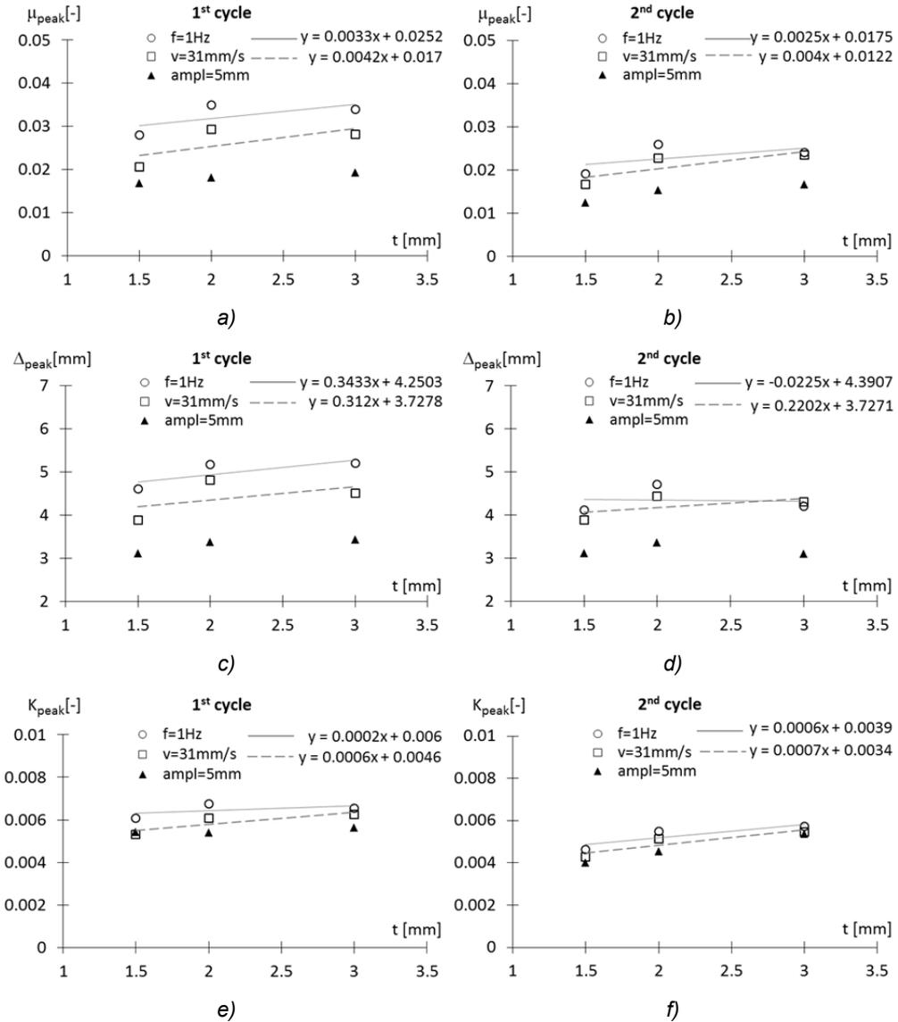
Fig. 6.31  $\mu_{peak}$ , relative displacement  $\Delta_{peak}$  and secant stiffness  $K_{peak}$  plotted versus the thickness  $t$  of the rubber layer. Case: rubber A,  $D=25\text{mm}$ ,  $W/ER^2=1.2$ .
