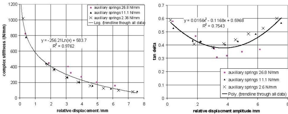
Fig. 3.6 Complex stiffness and loss tangent results, both versus relative displacement amplitude, for the systems used in the sinusoidal shaking table tests carried out at ISMES, Bergamo, 2000 (from Muhr & Bergamo, 2010).
