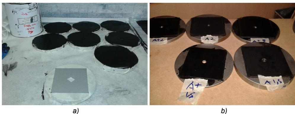
Fig. 6.33 Samples used to measure the geometric profiles of the pits: a) painting with Chemlok\_220 (bonding agent) after sandblasting of the steel plates; b) samples finished.
