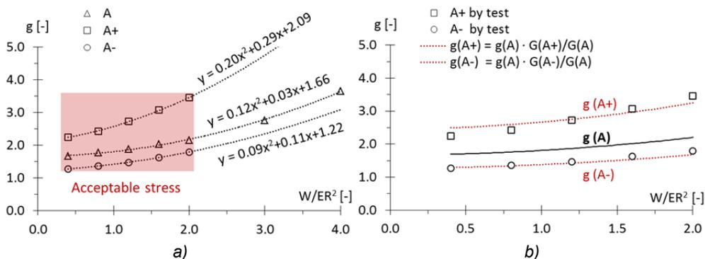
Fig. 5.20 a)  $g$  parameter (see Eq. (5.5)) needed to scale the hysteretic parameter value, calculated as  $\alpha = \pi \cdot \sin \delta$ , to have the best fitting between theory and test results. b) Comparison, for rubber A+ and A-, between the values of the parameter  $g$  obtained by tests and the ones calculated by Eq. (5.6), in which compound A is the reference one.
