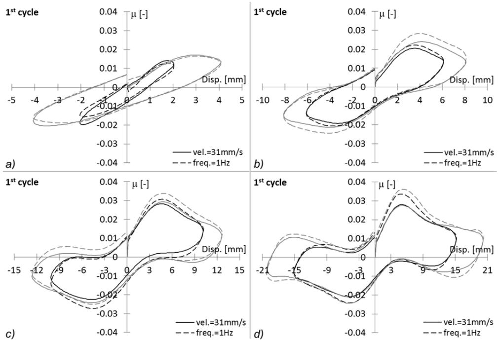
Fig. 6.4 Comparisons of  $\mu$ -disp loops - 1<sup>st</sup> cycle. Rubber A,  $t=2\text{mm}$ ,  $D=25\text{mm}$ ,  $W/ER^2=1.2$ .
