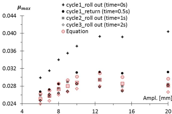
Fig. 6.77 Estimate of the recovery effects of the rubber on  $\mu_{max}$ , according to Eq. (6.20).
