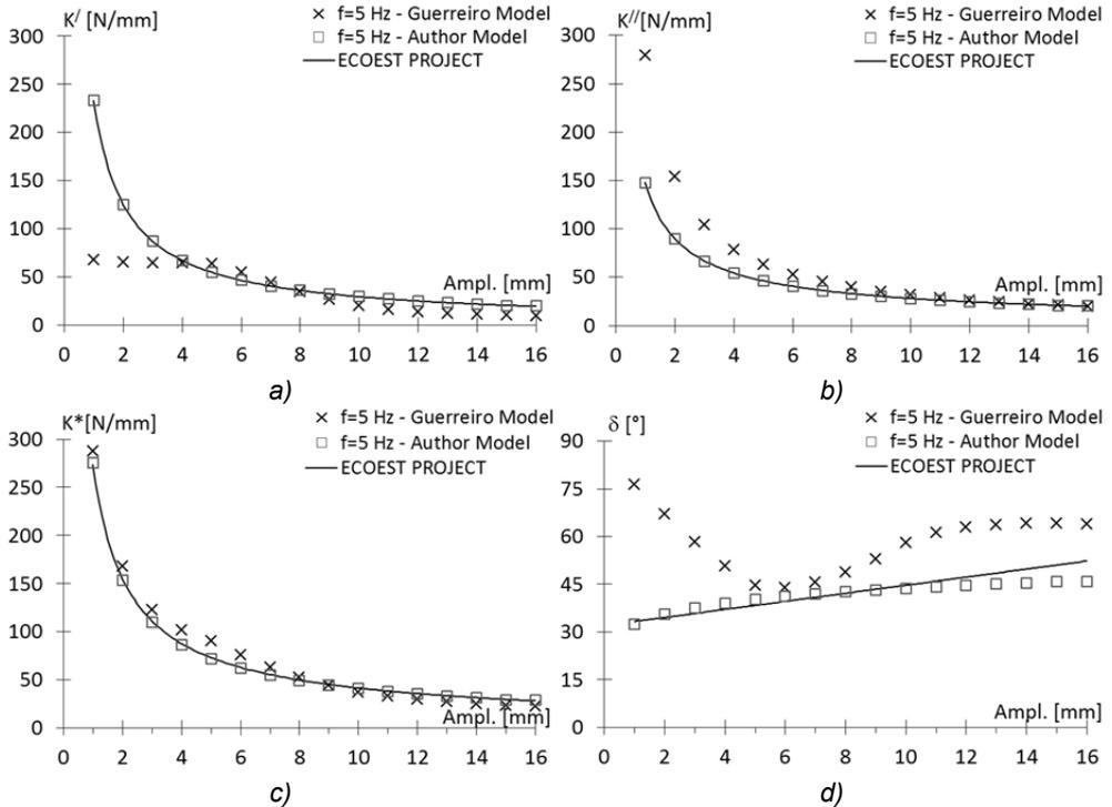
Fig. 4.16 Comparison of the ELVFD parameters, which describe the non-linear dynamic behaviour of the RBRL device, calculated by Guerreiro Model, Author Model and sinusoidal tests of the ECOEST project for different sinusoidal amplitudes: a) storage stiffness  $K'$ ; b) loss stiffness  $K''$ ; c) complex stiffness  $K^*$ ; d) loss angle  $\delta$ .
