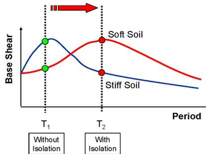
Fig. 2.11 Effects of the seismic isolation with different response spectra (from Symans, 2004).
