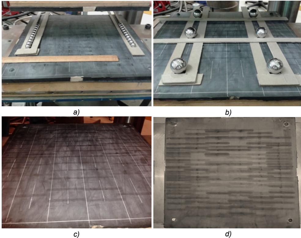
Fig. 5.13 a), b) Images of balls positioning. Images of rubber tracks, lower (c) and upper (d), after running some (c) / all (d) tests associated with that RBRL device.
