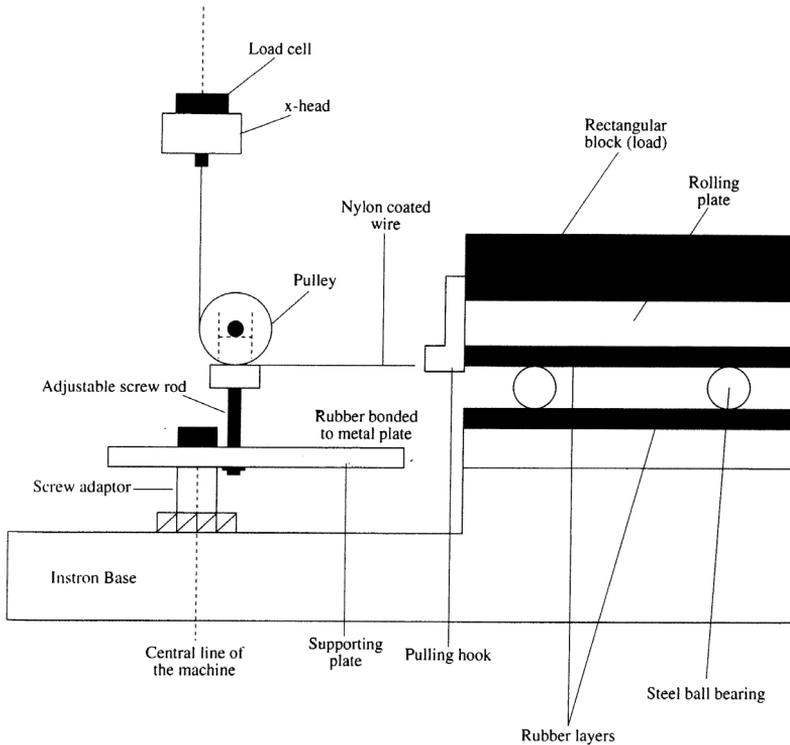
Fig. 3.10 Tests setup for measuring rolling forces (Muhr et al., 1997).
