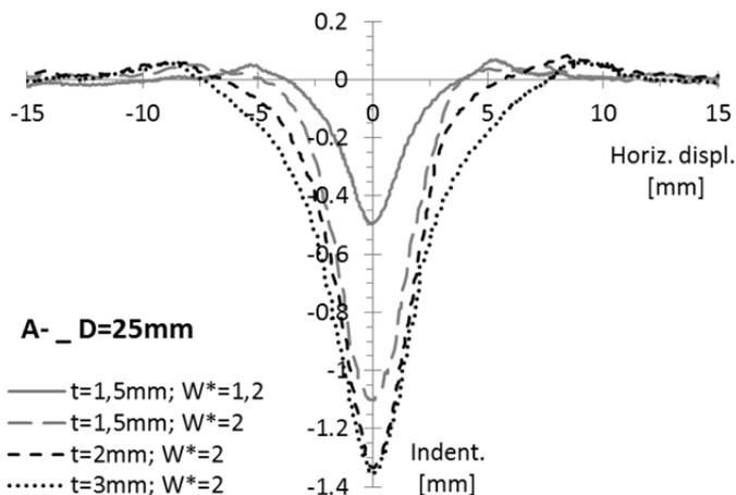
Fig. 6.45 Comparison of the geometric profiles of the residual indentation for the case of rubber A-,  $D=25\text{mm}$ , for different combinations of stress level ( $W^*=1.2, 2$ ) and thickness of rubber layer ( $t=1.5, 2, 3\text{ mm}$ ).
