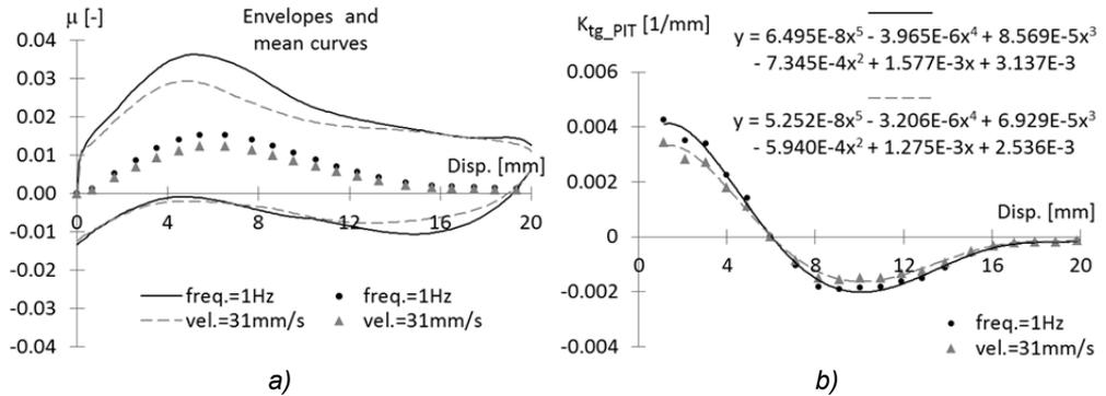
Fig. 6.86 a) Envelopes of the  $\mu$ -disp loops of the tests with constant velocity ( $v=31\text{mm/s}$ ) and constant frequency ( $f=1\text{Hz}$ ), for the reference RBRL device, presented in section 6.2. The points represent the non-linear elastic  $\mu$ -disp behaviour inside the pit, and were obtained by scaling the values of Fig. 6.84 a) by the ratio of the  $\mu_{peak}$  values. b) Related tangent stiffnesses.
