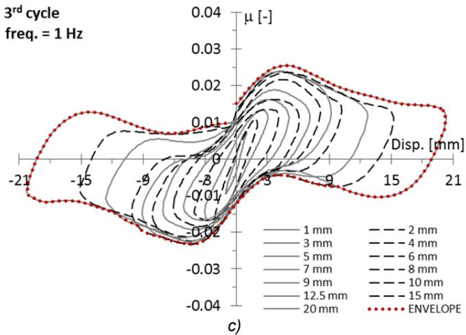
Fig. 6.2  $\mu$ -disp loops. Rubber A,  $t=2\text{mm}$ ,  $D=25\text{mm}$ ,  $W/ER^2=1.2$ , constant frequency.
