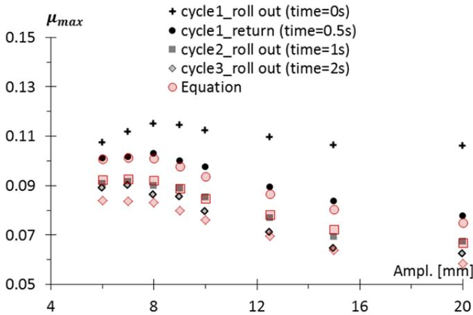
Fig. 6.79 Estimate of the recovery effects of the rubber on  $\mu_{max}$ , according to Eq. (6.20).
