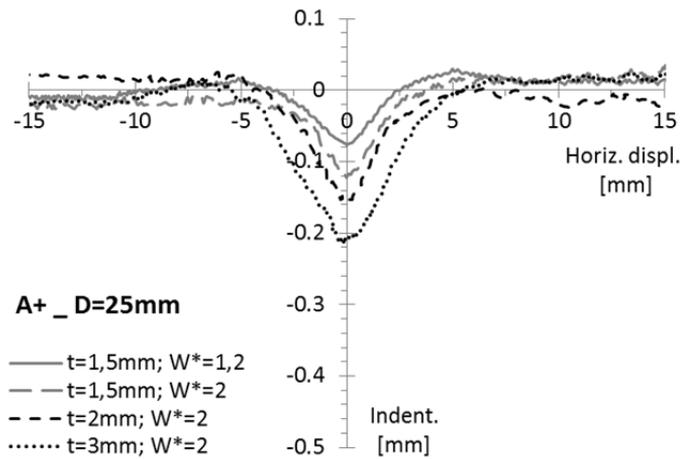
Fig. 6.43 Comparison of the geometric profiles of the residual indentation for the case of rubber A+, D=25mm, for different combinations of stress level ( $W^*=1.2, 2$ ) and thickness of rubber layer ( $t=1.5, 2, 3$  mm).
