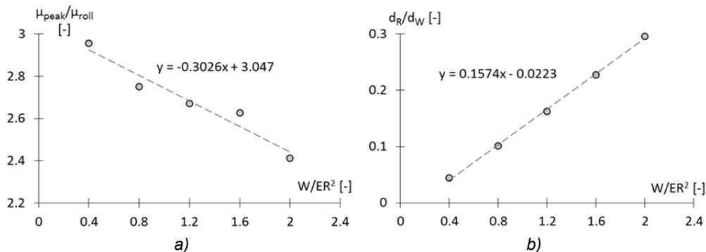
Fig. 6.65 Different dependence of the ratio  $\mu_{peak}/\mu_{roll}$  (a) and  $d_R/d_W$  (b) on the stress parameter  $W/ER^2$ . The values of  $\mu_{peak}$  were obtained by sinusoidal tests performed on the same device with rubber A,  $t = 2$  mm,  $D = 25$  mm, presented in section 6.2.
