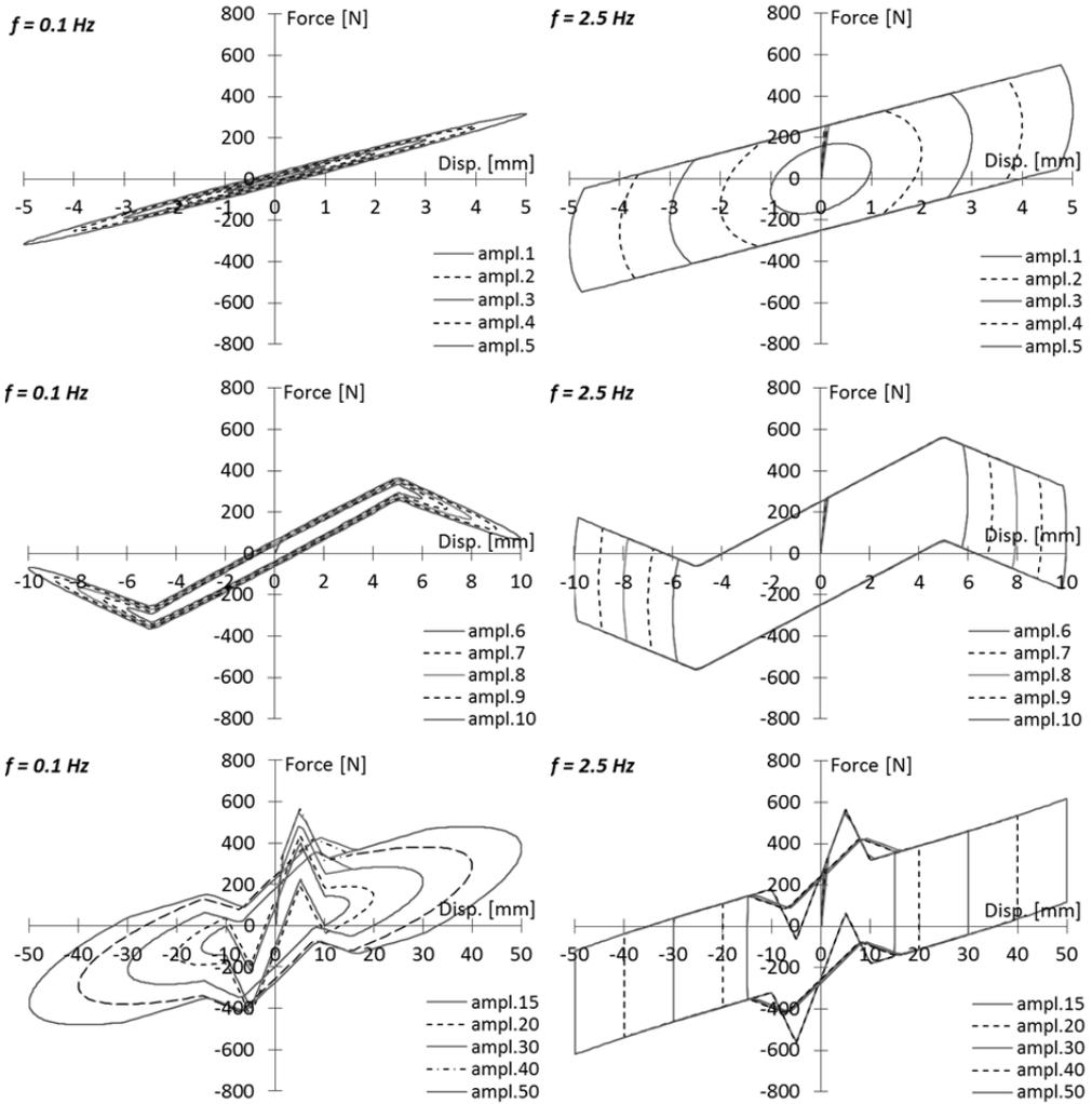
Fig. 4.12 Force-disp. loops from Guerreiro model for selected amplitudes and frequencies.
