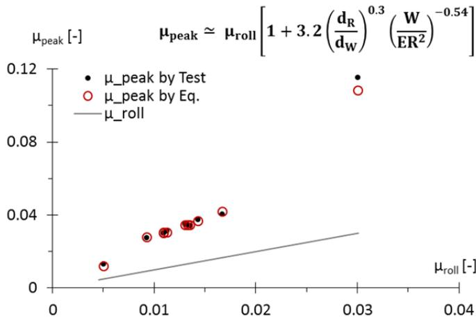
Fig. 6.68 Estimate of  $\mu_{peak}$  according to empirical Eq. (6.18) and comparison of the values with the experimental ones.
