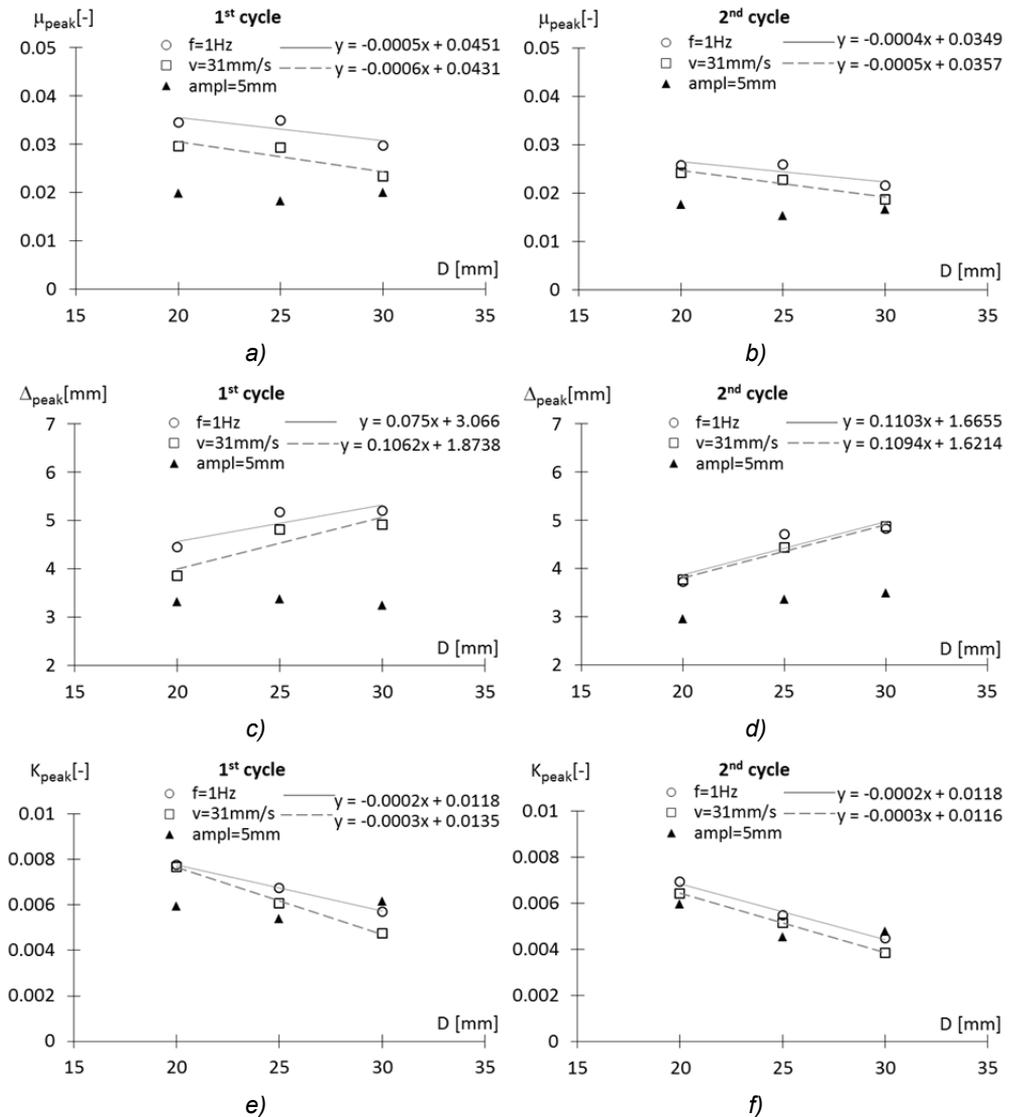
Fig. 6.30  $\mu_{peak}$ , relative displacement  $\Delta_{peak}$  and secant stiffness  $K_{peak}$  plotted versus the diameter  $D$  of the ball. Case: rubber A,  $t=2\text{mm}$ ,  $W/ER^2=1.2$ .
