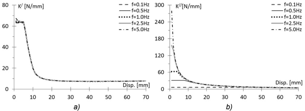
Fig. 4.13 a)  $K'$ , b)  $K''$  from the Guerreiro model for all the amplitudes and frequencies analysed.
