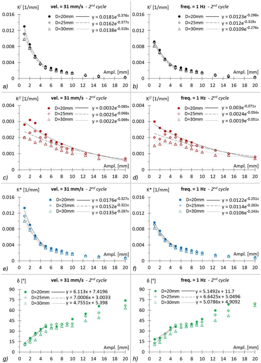
Fig. 6.22 Comparison of  $K'$ ,  $K''$ ,  $K^*$ ,  $\delta$  vs amplitude, for the values of the ball diameter  $D$  analyzed. Case: rubber A,  $t=2\text{mm}$ ,  $W/ER^2=1.2$  - 2<sup>nd</sup> cycle.
