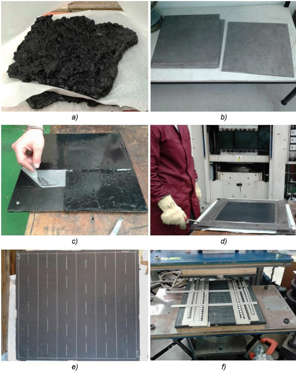
Fig. 5.1 Some images of the principal realization phases of the RBRL devices at TARRC.
