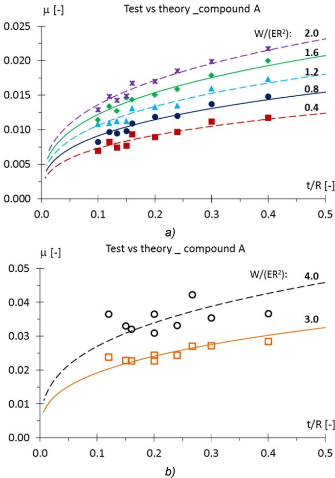
Fig. 5.15 Comparison, for the compound A, of the rolling friction values ( $\mu$ ) obtained by the tests and the theory, for different values of the thickness/radius ratio ( $t/R$ ). (a) Stress parameters ( $W/ER^2$ ) from 0.4 to 2.0 (b) Tests with higher stress parameters: 3.0 and 4.0.
