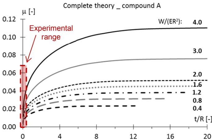
Fig. 5.19 Complete theory in terms of  $(t/R)$ , for rubber A, calibrated from experimentation.
