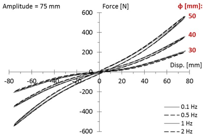
Fig. 6.82 Hysteretic loops from the sinusoidal tests (Ch. 5) with same amplitude, 75 mm, and different frequencies; diameters of the springs tested: 30, 40, 50 mm. Values for one spring.
