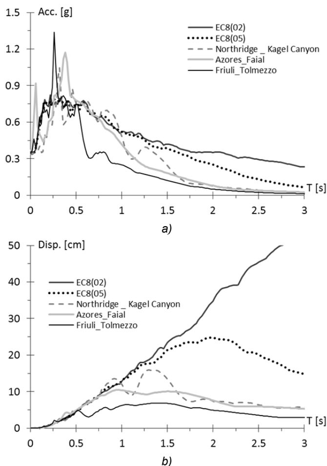
Fig. 4.3 a) Acceleration and b) displacement response spectra of the ground motion selected for the tests with Mass Up configuration, as recorded at the table ( $\zeta = 5\%$ ).
