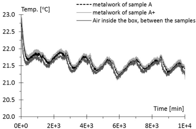
Fig. 5.9 Temperatures measured during the creep tests for the specimens A and A+.
