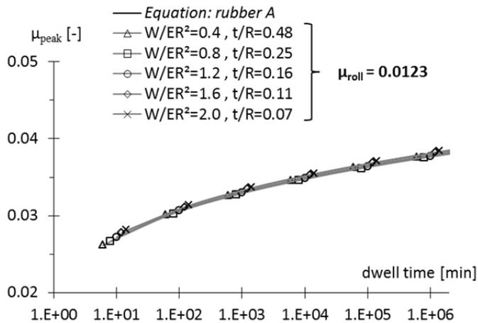
Fig. 6.73 Estimate of  $\mu_{peak}$ , according to Eq.(6.18), for rubber A,  $D = 25$  mm and different combinations of the parameters  $W/ER^2$  and  $t/R$ . Each of these combinations is characterized by the same value of  $\mu_{roll}$  according to the theory of Muhr et al. (1997).
