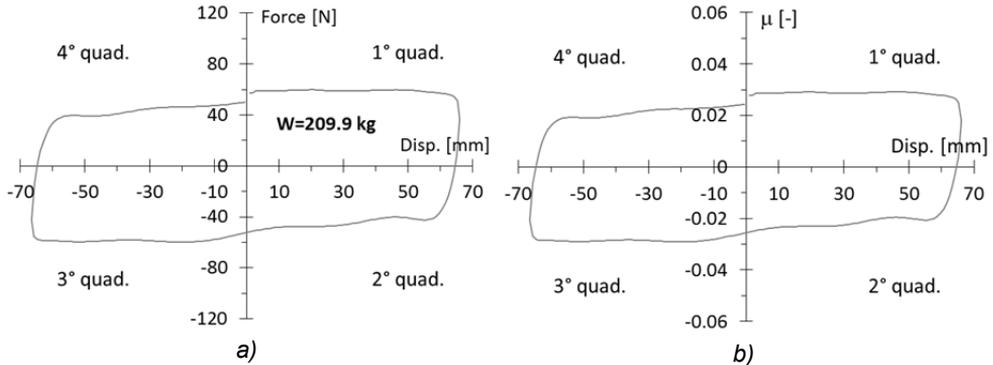
Fig. 5.14 a) Example of force (F)-displacement (D) loop, for the second sinusoidal cycle, for the case:  $A, t=2\text{mm}, D=20\text{mm}, W/ER^2=3$ . b) The same, in terms of friction coefficient  $\mu (=F/Wg)$ . The quadrants are numbered following the rolling of the balls.
