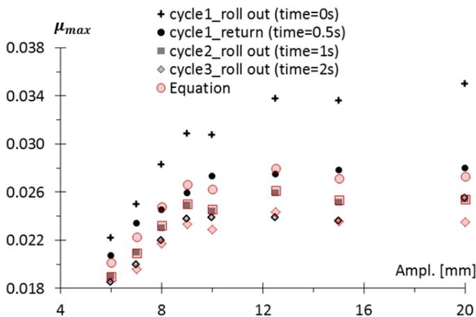
Fig. 6.75 Estimate of the recovery effects of the rubber on  $\mu_{max}$ , according to Eq. (6.20).
