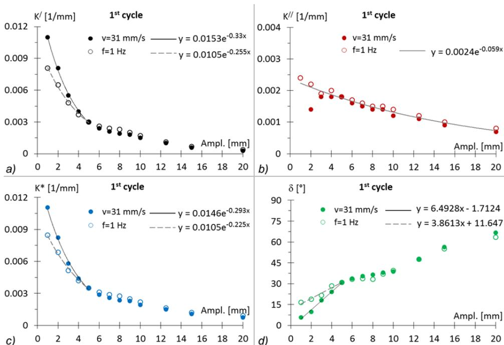
Fig. 6.18  $K'$ ,  $K''$ ,  $K^*$ ,  $\delta$  vs amplitude. Rubber A,  $t=2$ mm,  $D=25$ mm,  $W/ER^2=1.2$ , 1<sup>st</sup> cycle.
