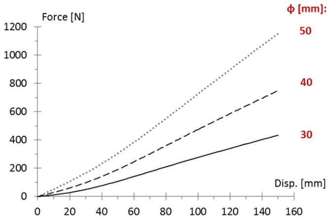
Fig. 5.29 Force-deflection plots from quasi-static tests; diameters of the springs tested: 30, 40, 50 mm. Values for one spring.
