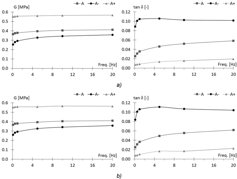
Fig. 5.6 Dynamic shear properties of rubber compounds (A, A+,A-) by Harmonic (a) and Secant (b) linearization method – influence of frequency for a 10% strain.
