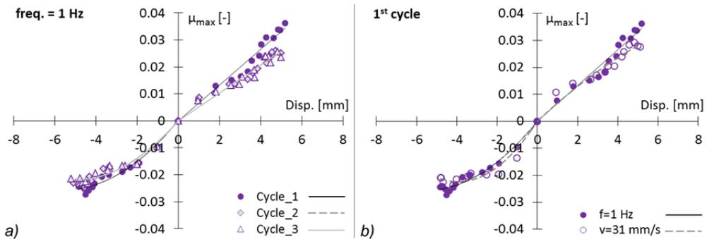
Fig. 6.20  $\mu_{max}$  vs displacement. Rubber A,  $t=2\text{mm}$ ,  $D=25\text{mm}$ ,  $W/ER^2=1.2$ . a) Different cycles, all at 1 Hz; b) comparison of constant frequency (1 Hz) and velocity (31 mm/s) results for first cycles.
