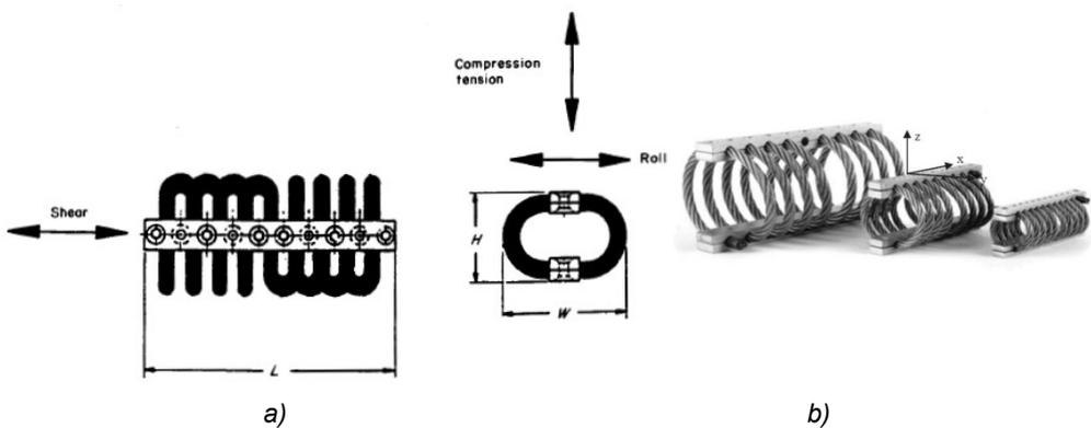
Fig. 2.31 “Wire-Rope” or “Steel Cable Dampers” device. Images from: a) Demetriades et al., 1993 and b) Alessandri et al., 2014.
