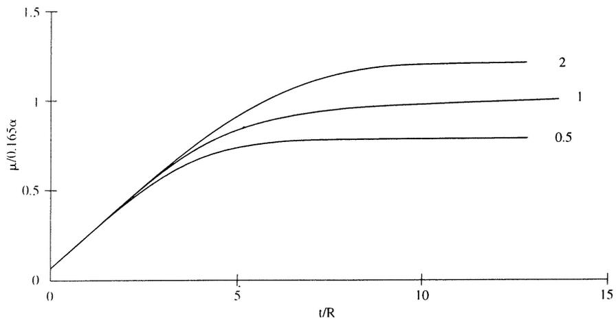
Fig. 3.9 Parametric schematic plots of rolling friction ratio  $\mu$ , scaled using  $\alpha$ , versus dimensionless ratio of rubber layer thickness to ball radius (Eqs.(3.28),(3.16)).  $W/ER^2$  is the stress parameter (Muhr et al., 1997).
