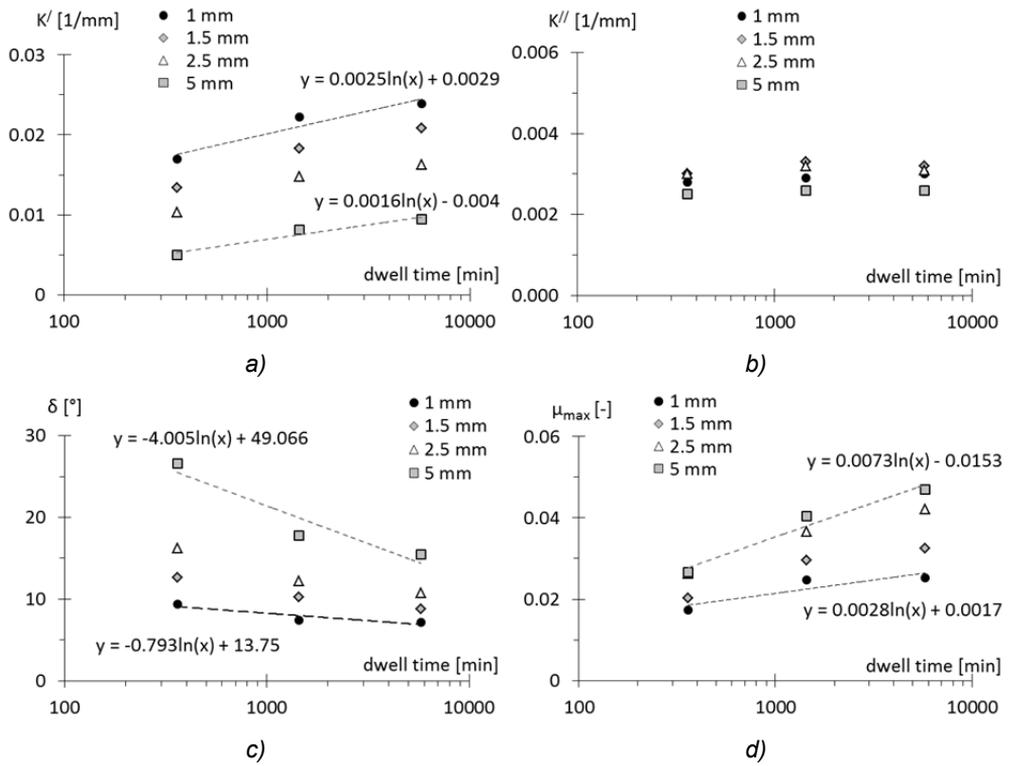
Fig. 6.62 Dependence of  $K'$ ,  $K''$ ,  $\delta$  and  $\mu_{max}$  on the logarithm of the dwell time, for amplitudes up to 5 mm (balls inside pits). Case: tracks A-A,  $W = 250$  N, max. vel. = 31 mm/s, 2<sup>nd</sup> cycle.
