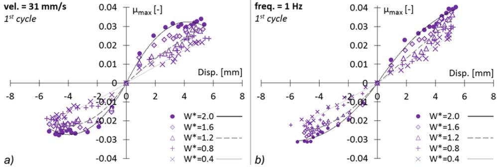
Fig. 6.25 Comparison of  $\mu_{max}$  vs displacement, for the values of the stress parameter  $W^*$  analyzed. Case: rubber A,  $t=2\text{mm}$ ,  $D=25\text{mm}$  \_ 1<sup>st</sup> cycle.
