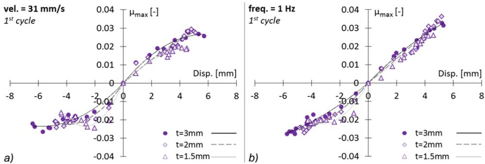
Fig. 6.27 Comparison of  $\mu_{max}$  vs displacement, for the values of the rubber thickness  $t$  analyzed. Case: rubber A,  $D=25\text{mm}$ ,  $W/ER^2=1.2$  \_ 1<sup>st</sup> cycle.
