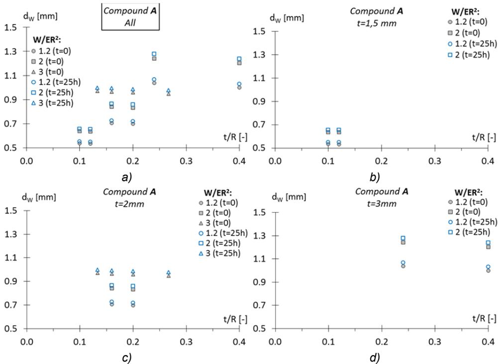
Fig. 6.50 a) Maximum indentations under load given by Waters' equations (Eqs. (6.6) and (6.7)), considering the Young's modulus ( $t=0$ ) and the one relaxed after 25 hours ( $t=25h$ ), for the case of rubber A and different values of  $t/R$  and  $W/ER^2$ . The same results are reproduced in the figures b), c), d) for the different values of rubber layer thickness analyzed.
