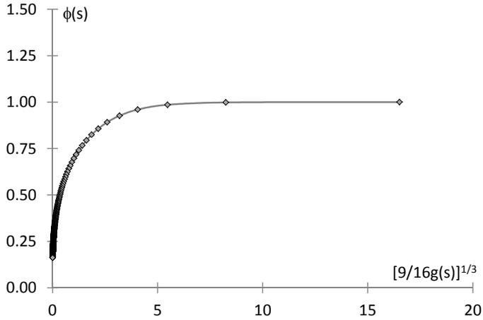
Fig. 3.17 Theoretical plot of reduced friction ratio versus reduced rubber thickness (Eq. (3.28)), for lubricated condition.
