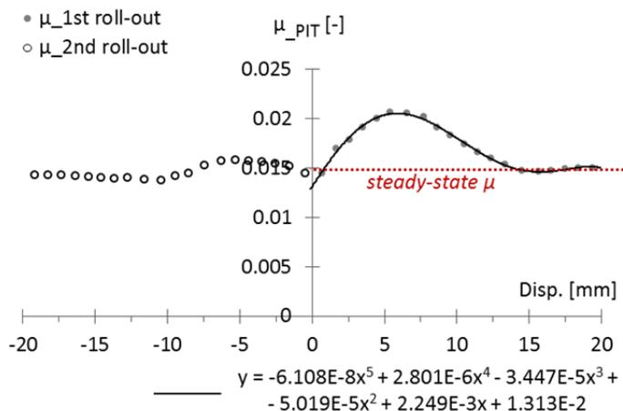
Fig. 6.85 Influence of the pits on the rolling friction resistance for small displacements of the balls. Test at 65 mm and 0.5 Hz, on the reference RBRL device.
