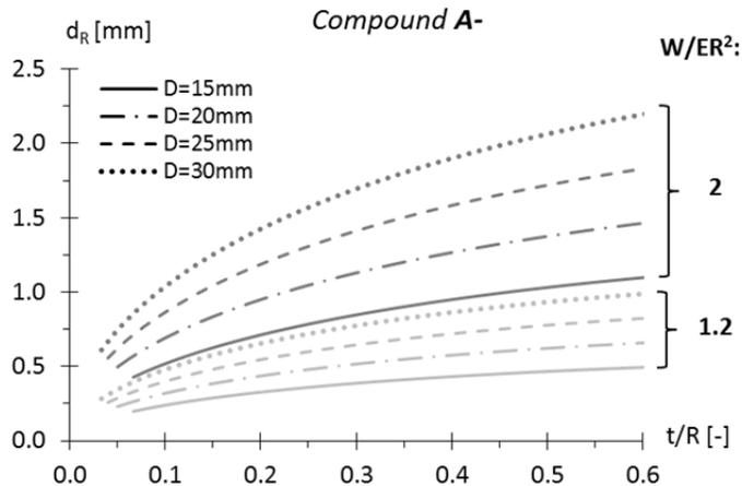
Fig. 6.56 Estimate of the maximum residual indentation  $d_R$  through the Eq. (6.12), after a dwell time of the load of 25 hours, for the rubber A- and for a certain range of  $t/R$  and  $W/ER^2$ .
