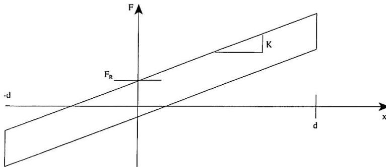
Fig. 3.3 Schematic hysteresis loop for isolation system comprising rolling-ball dissipative-layer isolators and springs (from Cook et al., 1997).
