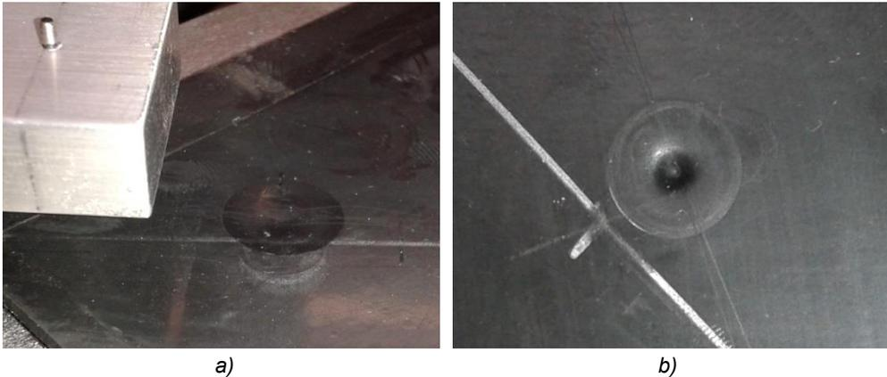
Fig. 6.47 Different shape of the profile of the residual indentation: a) recovery of the rubber at the same velocity (typical for rubber A+, and A with  $W^* < 2$ ); b) recovery of the rubber with different velocities inside the pit, slower in the central part (typical for rubber A-).
