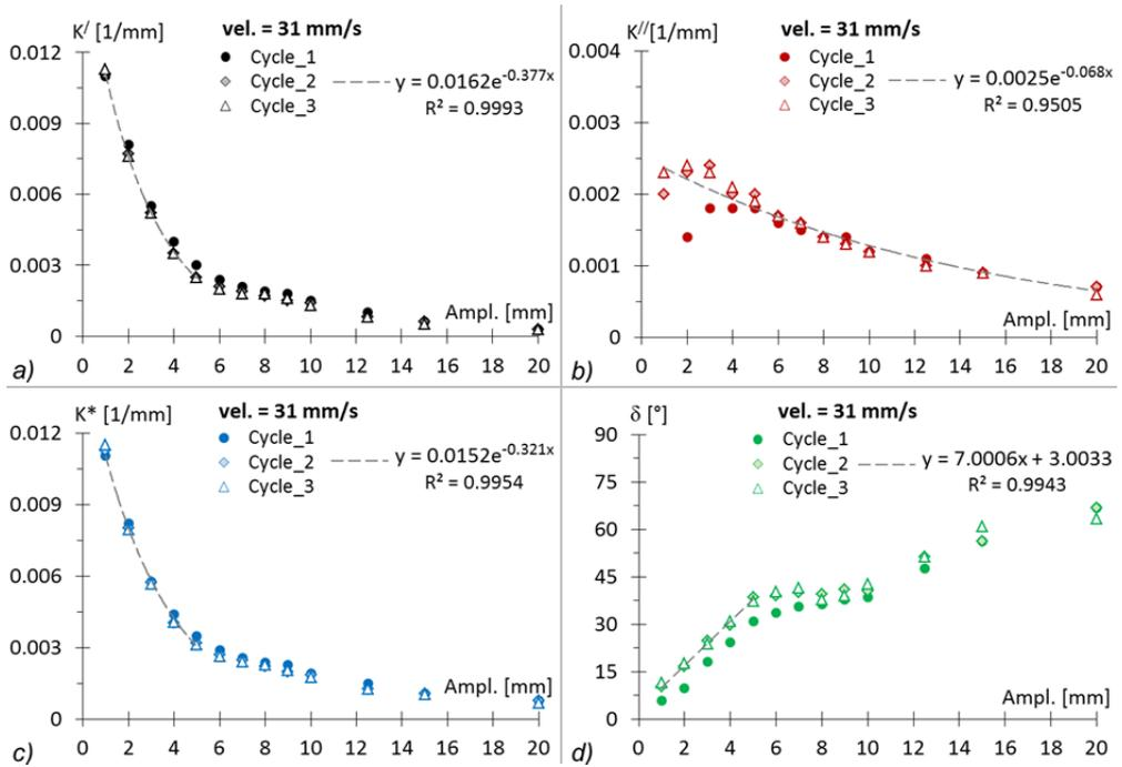
Fig. 6.16  $K'$ ,  $K''$ ,  $K^*$ ,  $\delta$  vs ampl. Rubber A,  $t=2\text{mm}$ ,  $D=25\text{mm}$ ,  $W/ER^2=1.2$ , constant velocity.
