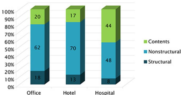
Fig. 1.5 Typical cost breakdown in building construction, according to Taghavi & Miranda (2003), for three different occupancies (image from FEMA E-74, 2011).
