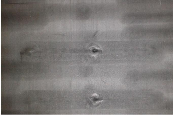
Fig. 5.18 Semi-permanent rolling tracks after a test with rubber A and stress parameter 4.
