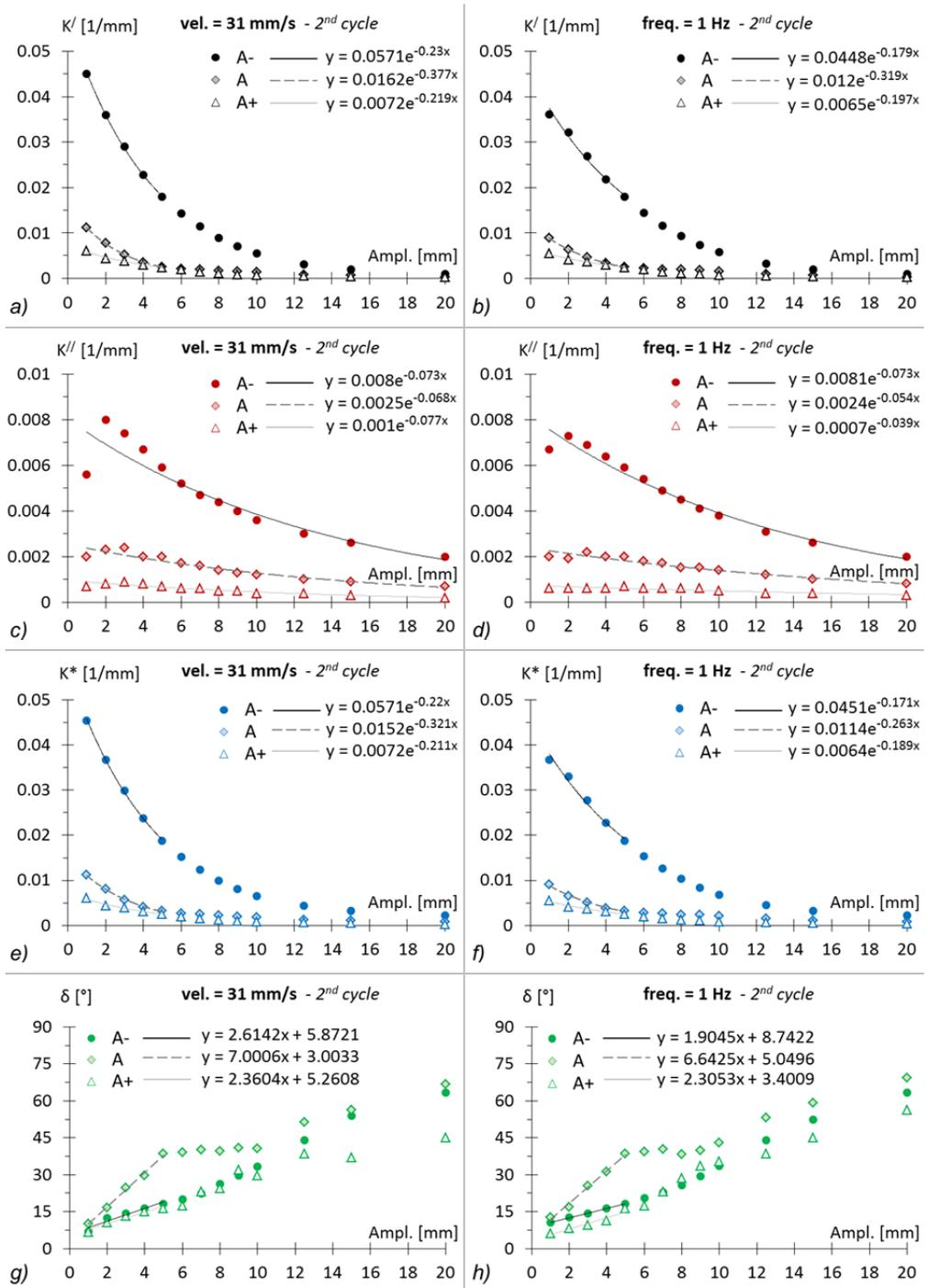
Fig. 6.24 Comparison of  $K'$ ,  $K''$ ,  $K^*$ ,  $\delta$  vs amplitude, for the different rubbers (A-, A, A+) analyzed. Case:  $t=2\text{mm}$ ,  $D=25\text{mm}$ ,  $W/ER^2=1.2$  - 2<sup>nd</sup> cycle.
