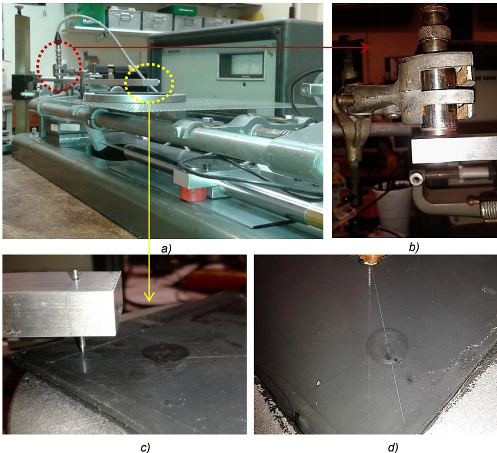
Fig. 6.36 Details of the setup (a) for the measurement of the pit profiles: b) non-contacting capacitance probe and c) needle probe at the two ends of the aluminium alloy bar. d) View of a pit after some measures (the lines shown the measurement directions).
