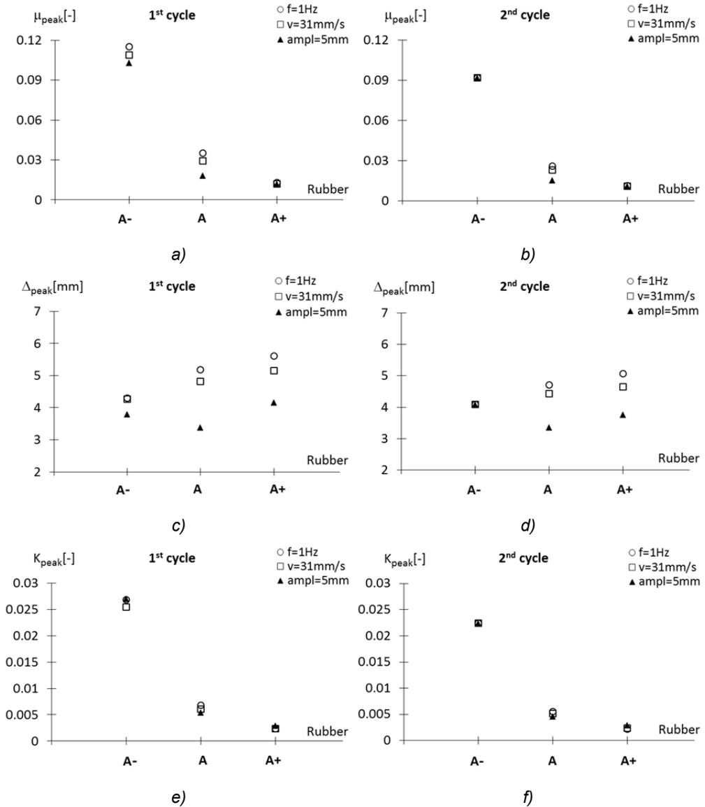
Fig. 6.32  $\mu_{peak}$ , relative displacement  $\Delta_{peak}$  and secant stiffness  $K_{peak}$  plotted versus the type of the rubber. Case:  $t=2\text{mm}$ ,  $D=25\text{mm}$ ,  $W/ER^2=1.2$ .
