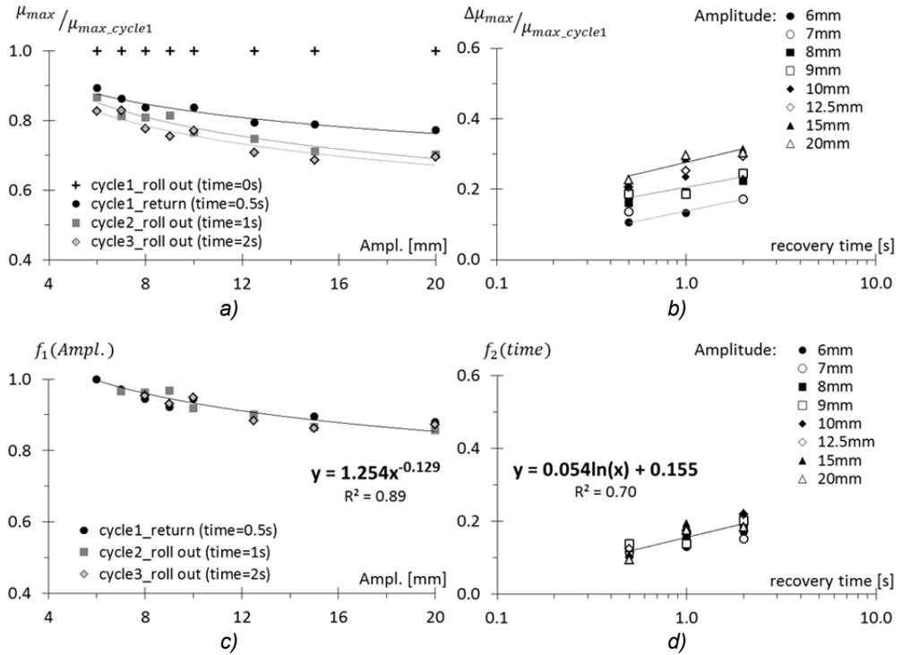
Fig. 6.76 a), b) Effects of the recovery of the rubber on the maximum rolling friction  $\mu_{max}$  due to the roll-out of the balls from their pits. c), d) Interpolating equations for the functions  $f_1(\text{Ampl.})$  and  $f_2(\text{time})$  necessary to apply the equation Eq. (6.20).
