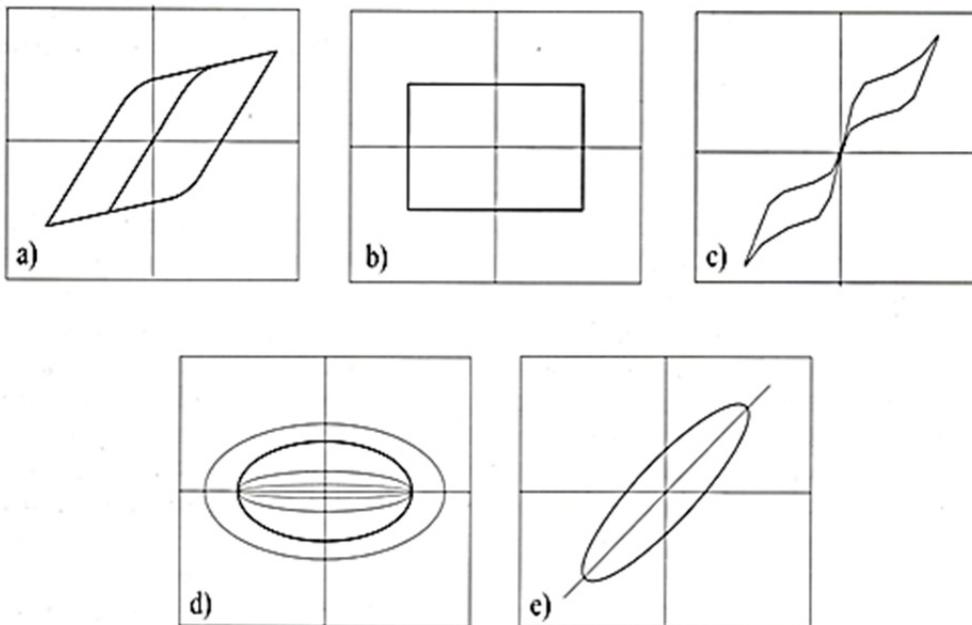
Fig. 2.13 Ideal force-displacement loops of auxiliary devices based on: a) hysteresis of some metals; b) friction; c) superelastic properties of shape memory materials; d) viscous behaviour; e) quasi-linear or viscoelastic behaviour (from Dolce et al., 2010).
