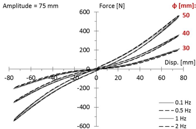
Fig. 5.26 Hysteretic loops from the sinusoidal tests with same amplitude, 75 mm, and different frequencies; diameters of the springs tested: 30, 40, 50 mm. Values for one spring.
