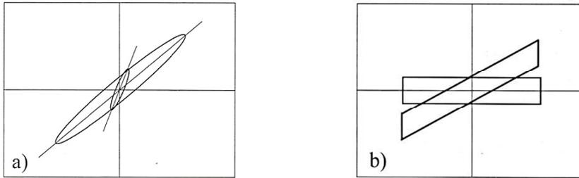
Fig. 2.12 Ideal force-displacement loops of: a) isolators made of elastomeric material and steel; b) sliding isolators (from Dolce et al., 2010).
