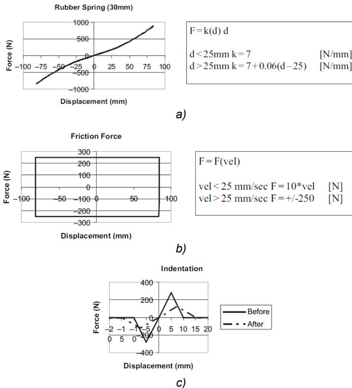
Fig. 3.4 a) Rubber spring analytical model, b) track surface friction model, c) analytical model of the indentation effects, by Guerreiro et al. (2007).
