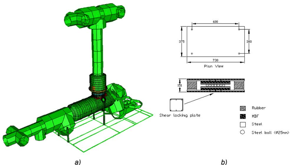
Fig. 2.33 a) GIS 3-Dimensional Finite Element model. b) RBRL isolation device (see next Chapter for more details about this device, in particular Tab. 3.1).
