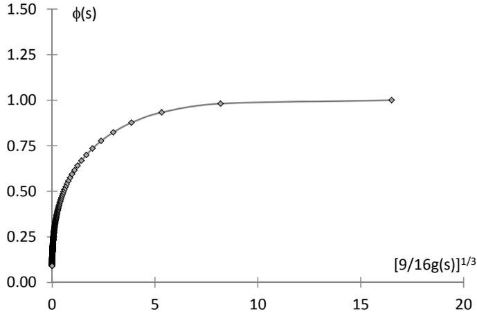
Fig. 3.13 New calculation of the theoretical plot of reduced friction ratio versus reduced rubber thickness (Eq. (3.28)).
