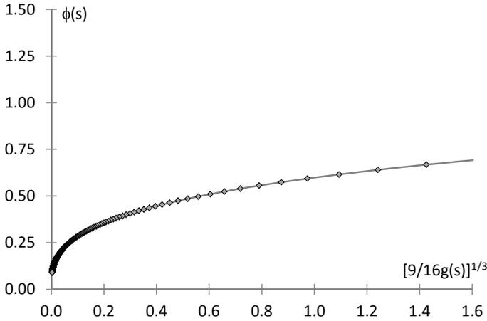
Fig. 3.15 New calculation of the theoretical plot of reduced friction ratio versus reduced rubber thickness (Fig. 3.13), represented for a smaller range of abscissa values, compatible with the experimentation.
