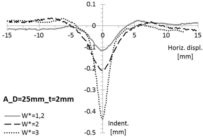
Fig. 6.37 Comparison of the geometric profiles of the residual indentation for the case of rubber A,  $D=25\text{mm}$ ,  $t=2\text{mm}$ , for different values of the stress level ( $W^*=1.2, 2, 3$ ).
