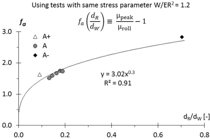
Fig. 6.66 Interpolating function  $f_a$  according to Eq. (6.16).
