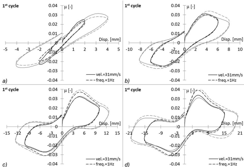
Fig. 6.8 Comparisons of  $\mu$ -disp loops – 1<sup>st</sup> cycle. Rubber A,  $t=2\text{mm}$ ,  $D=25\text{mm}$ ,  $W/ER^2=2$ .
