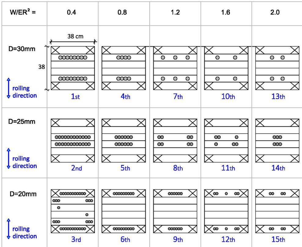
Fig. 5.12 Planning of the tests execution order and balls position: rubber A, layer thickness 1.5 mm
