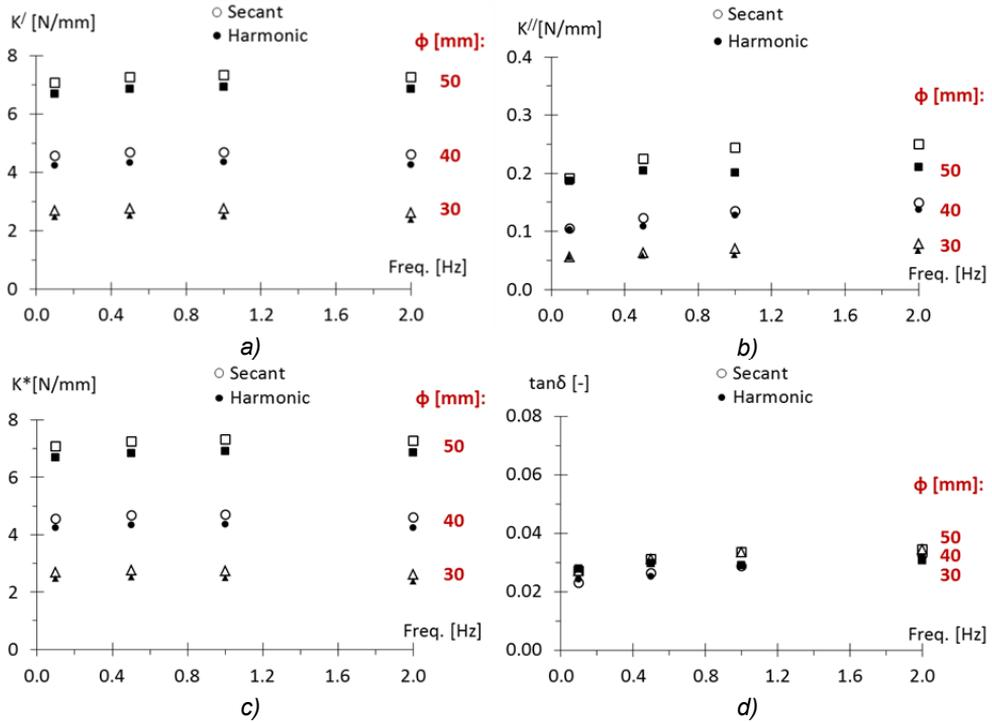
Fig. 5.28 ELVFD parameters from sinusoidal tests at the same amplitude, 75 mm. Comparison between the Harmonic and Secant linearization methods. Values for one spring.
