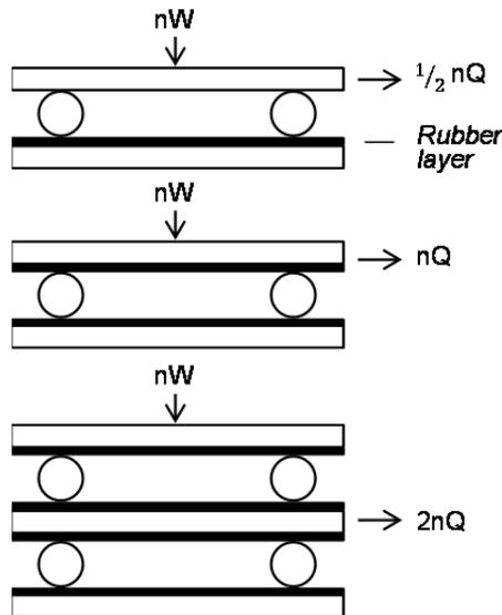
Fig. 3.7 Possible schemes, with the position of balls and rubber layers, for experimental determination of rolling resistance;  $n$  indicates the number of balls in one layer.
