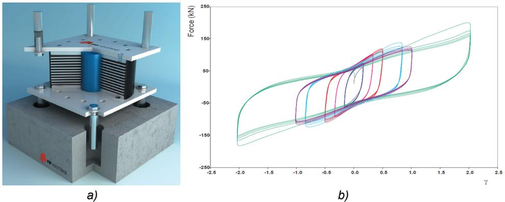
Fig. 2.15 a) Image of the Lead Rubber Bearing (LRB). b) Typical hysteresis loops of a LRB isolator obtained by dynamic tests at increasing shear strain amplitude  $\gamma$  (from FIP Industriale S.p.A., 2015).
