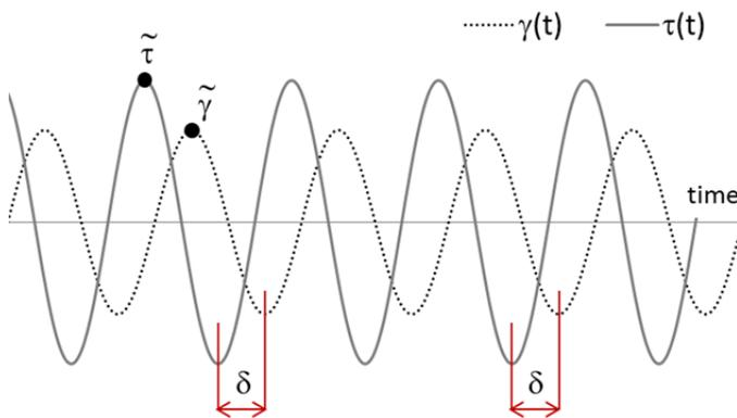
Fig. 3.20 Sinusoidal stress response  $\tau(t)$  to an imposed sinusoidal shear strain  $\gamma(t)$  for a viscoelastic material.
