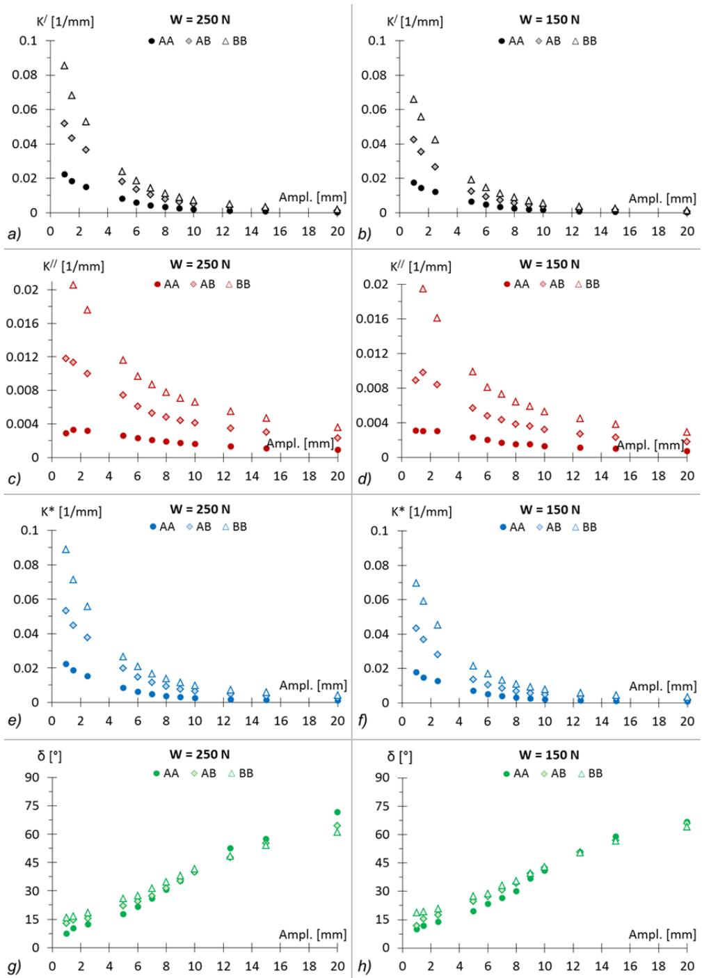
Fig. 6.59 Comparison of  $K'$ ,  $K''$ ,  $K^*$ ,  $\delta$  vs amplitude, for the different rubber tracks considered: A-A, A-B and B-B. Case:  $t_{dw} = 24$  hours, max. vel. = 31 mm/s,  $2^{nd}$  cycle.
