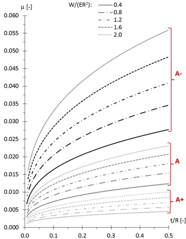
Fig. 6.81 Theoretical  $\mu$  values, calibrated through the experimentation (Ch. 5), for each compound (A+, A, A-) and stress parameter ( $W/ER^2$ ) analyzed, for an adequate range of  $t/R$ .
