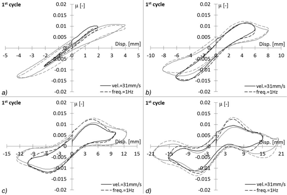
Fig. 6.11 Comparisons of  $\mu$ -disp loops-1<sup>st</sup> cycle. Rubber A+,  $t=2\text{mm}$ ,  $D=25\text{mm}$ ,  $W/ER^2=1.2$ .
