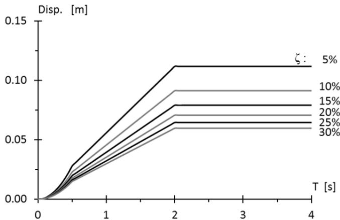
Fig. 5.38 Design displacement response spectra from EC8 (2004), assuming a spectrum of “type 1”, a ground of “type B” and a bedrock acceleration of 0.15 [g].
