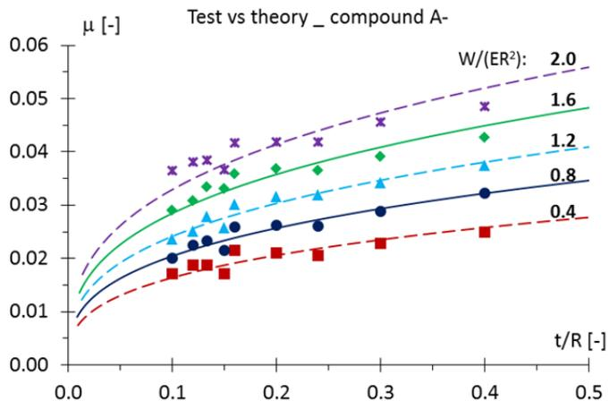
Fig. 5.17 Comparison, for the compound A-, of the rolling friction values ( $\mu$ ) obtained by the tests and the theory, for different thickness/radius ratios ( $t/R$ ) and stress parameters ( $W/ER^2$ ).
