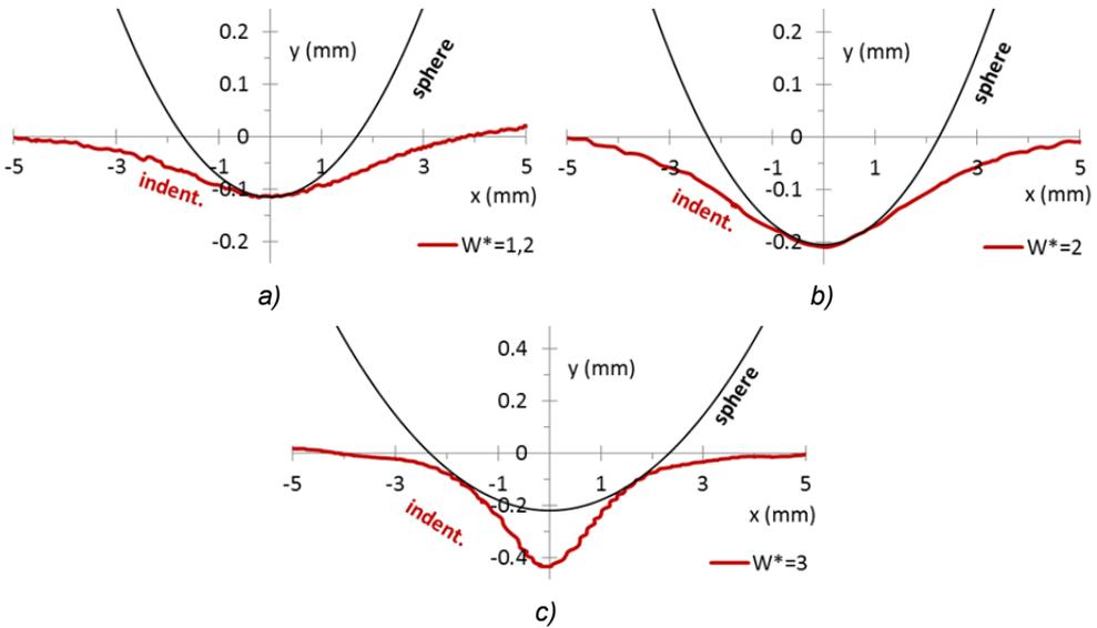
Fig. 6.38 Geometric profiles of Fig. 6.37 with the indication of the relative indenter.
