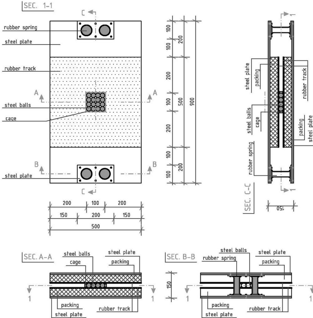
Fig. 3.1 Combined package of RBRL bearing and recentering springs as used for REEDS and ECOEST projects, by Donà et al. (2014).
