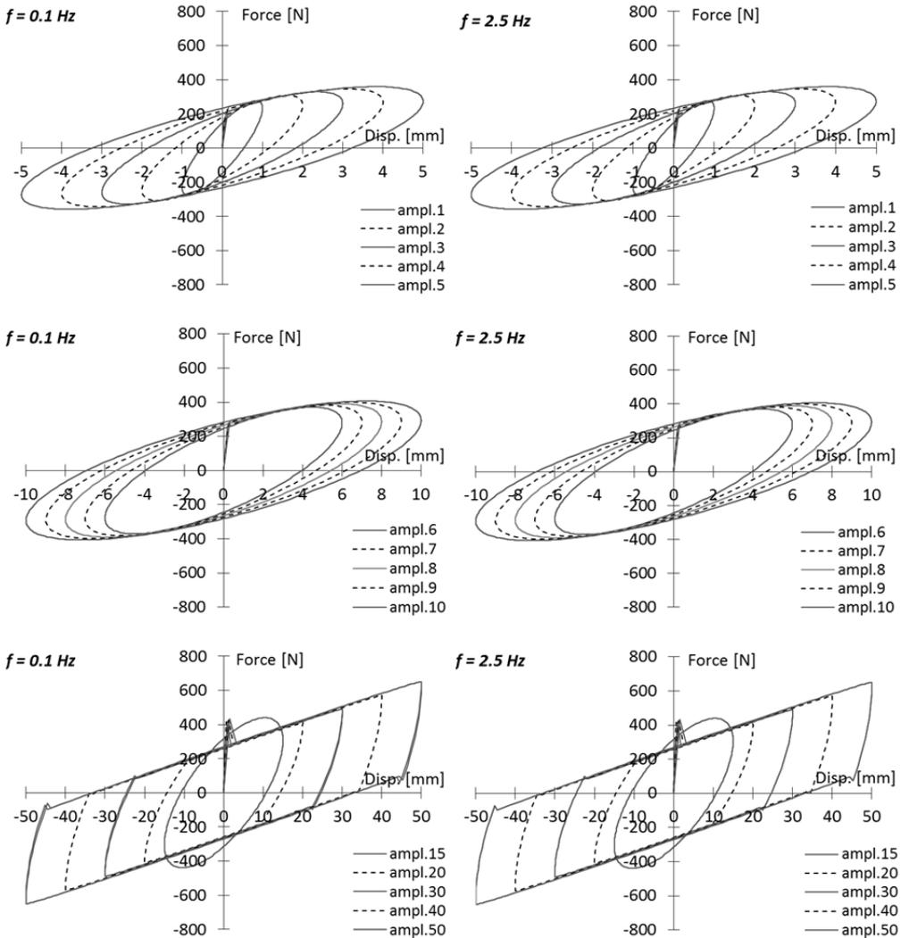
Fig. 4.15 Force-disp. loops from author model for selected amplitudes and frequencies.
