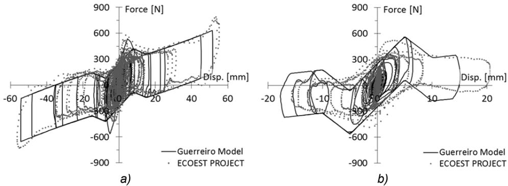
Fig. 4.11 Comparison of directly measured and modelled force-displacement plots for NorthridgePCKC: a) 0 dB; b) -12 dB.
