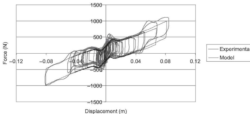
Fig. 3.5 Force-displacement response results comparison using the Guerreiro Model and for the seismic input of Northridge Kagel Canyon - monoaxial (+3dB), by Guerreiro et al. (2007).
