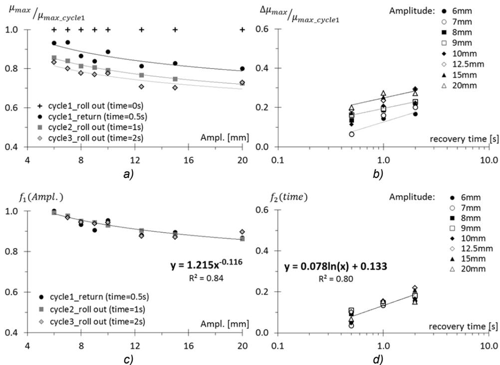
Fig. 6.74 a), b) Effects of the recovery of the rubber on the maximum rolling friction  $\mu_{max}$  due to the roll-out of the balls from their pits. c), d) Interpolating equations for the functions  $f_1(\text{Ampl.})$  and  $f_2(\text{time})$  necessary to apply the equation Eq. (6.20).
