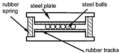
Fig. 3.2 Simplified representation of the RBRL system (from Guerreiro et al. 2007).
