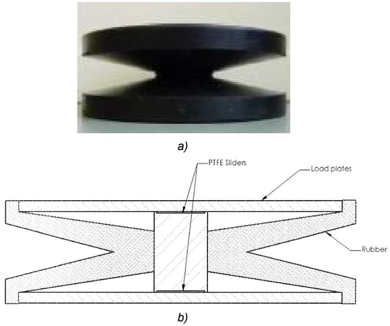
Fig. 2.35 RoGlider seismic isolator: a) image (from <http://www.robinsonseismic.com>) and b) section (from Robinson et al., 2006).
