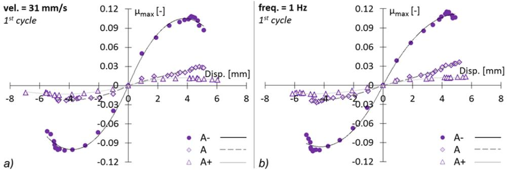
Fig. 6.28 Comparison of  $\mu_{\max}$  vs displacement, for the different rubbers (A-, A, A+) analyzed. Case:  $t=2\text{mm}$ ,  $D=25\text{mm}$ ,  $W/ER^2=1.2$  \_ 1<sup>st</sup> cycle.
