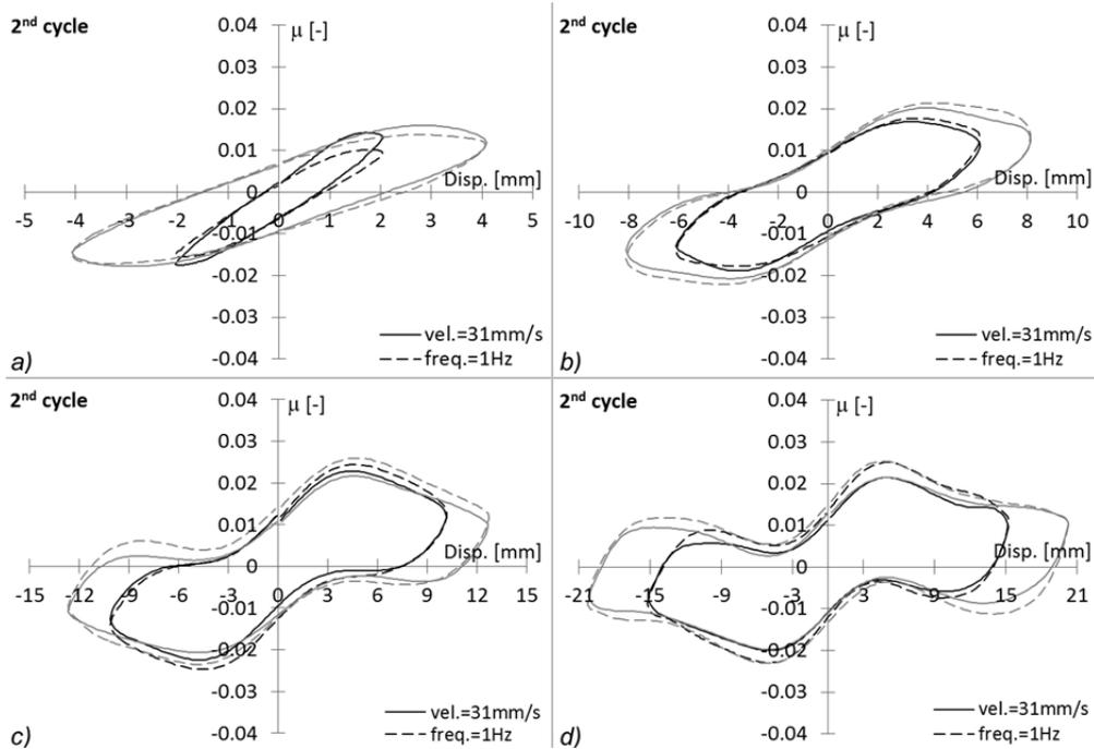
Fig. 6.5 Comparisons of  $\mu$ -disp loops - 2<sup>nd</sup> cycle. Rubber A,  $t=2\text{mm}$ ,  $D=25\text{mm}$ ,  $W/ER^2=1.2$ .
