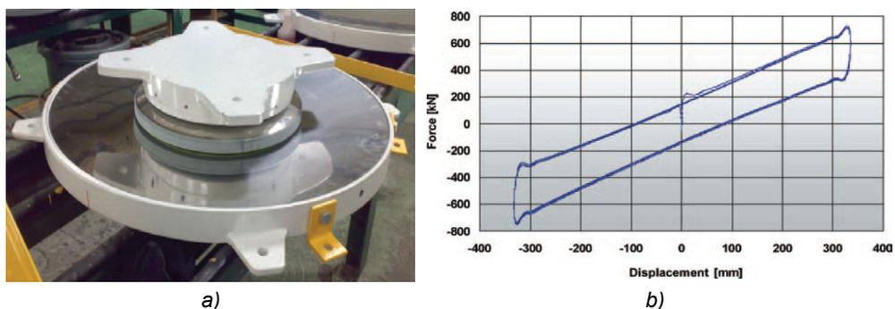
Fig. 2.16 a) Image of a curved surface slider or friction pendulum system (FPS) device. b) Relative hysteresis loop (from FIP Industriale S.p.A., 2015).
