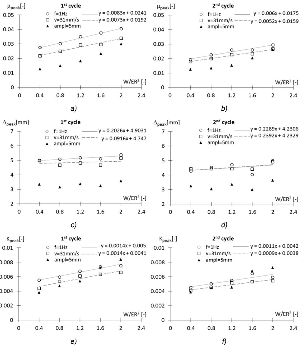
Fig. 6.29  $\mu_{peak}$ , relative displacement  $\Delta_{peak}$  and secant stiffness  $K_{peak}$  plotted versus the stress parameter  $W/ER^2$ . Case: rubber A,  $t=2\text{mm}$ ,  $D=25\text{mm}$ .
