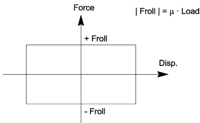
Fig. 6.80 Modelling of the steady-state rolling resistance.
