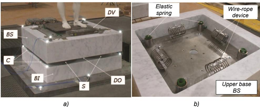
Fig. 2.29 Principal parts of the isolation system. a) Global view of the device. b) Internal view of the upper base (from De Canio, 2012).
