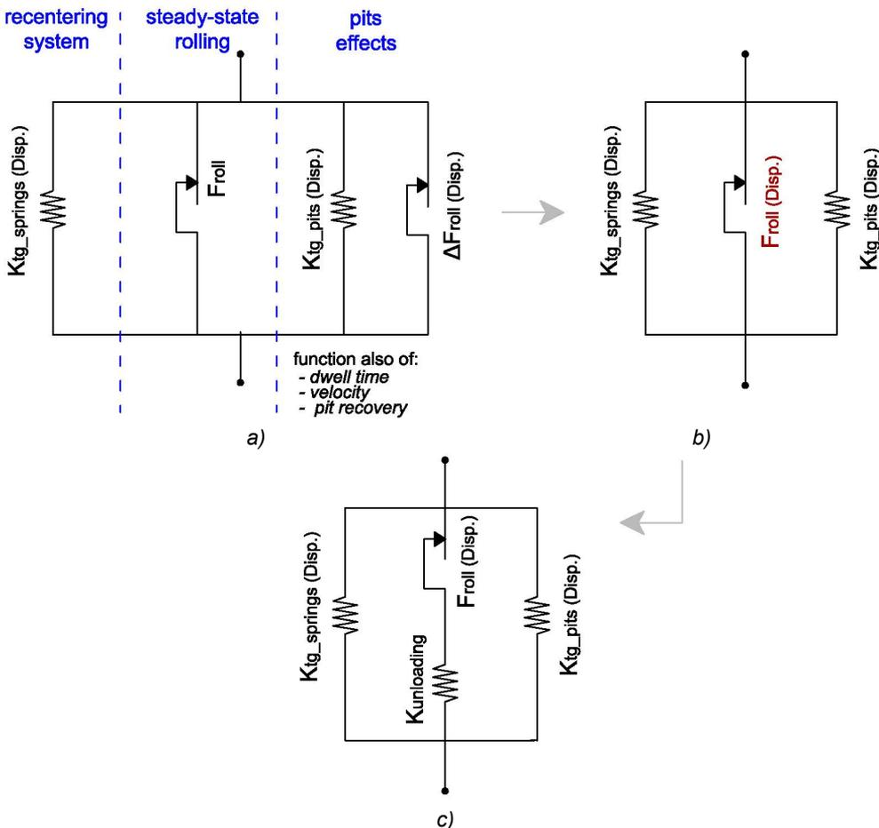
Fig. 6.88 Proposal of a time-domain model for the RBRL isolation system.
