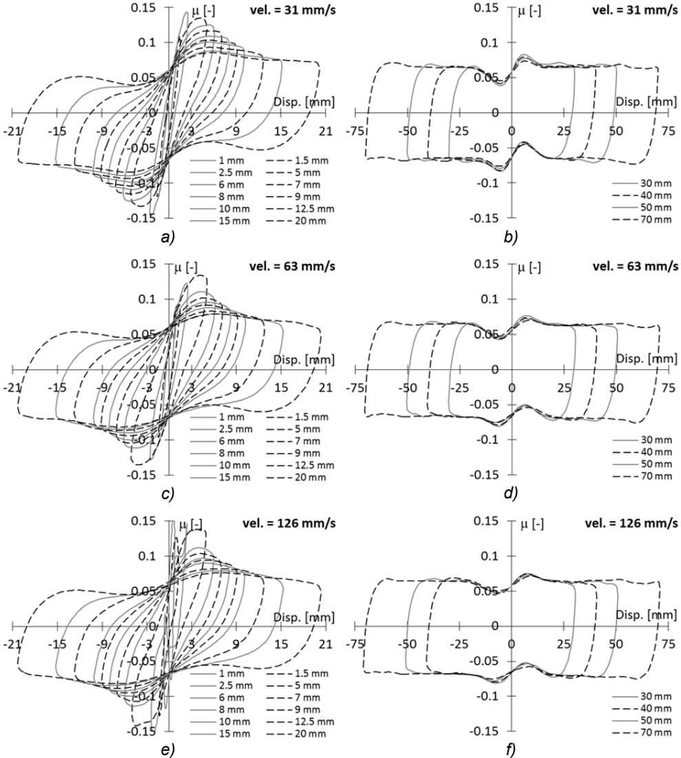
Fig. 6.58  $\mu$ -disp loops. Case: rubber tracks B-B,  $W = 250$  N,  $t_{dw} = 24$  h, 2<sup>nd</sup> cycle.
