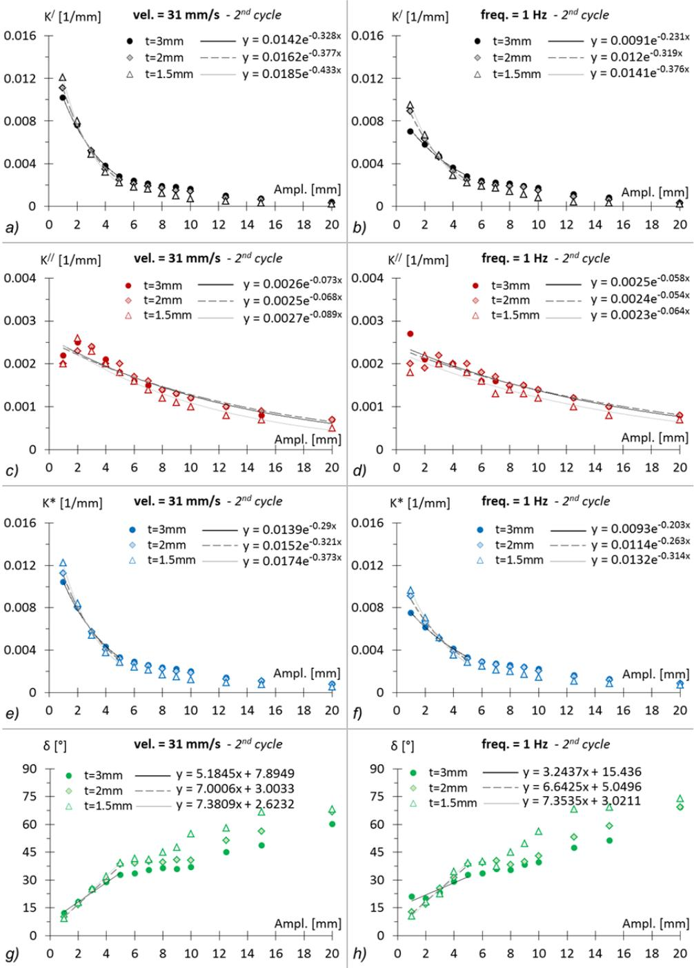
Fig. 6.23 Comparison of  $K'$ ,  $K''$ ,  $K^*$ ,  $\delta$  vs amplitude, for the values of the rubber thickness  $t$  analyzed. Case: rubber A,  $D=25\text{mm}$ ,  $W/ER^2=1.2$  - 2<sup>nd</sup> cycle.
