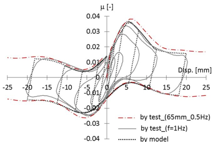
Fig. 6.89 Comparison of the real  $\mu$ -disp loops (no recentering springs) with those predicted by the model.
