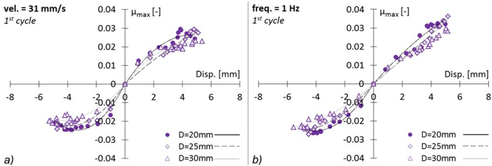
Fig. 6.26 Comparison of  $\mu_{max}$  vs displacement, for the values of the ball diameter  $D$  analyzed. Case: rubber A,  $t=2\text{mm}$ ,  $W/ER^2=1.2$  \_ 1<sup>st</sup> cycle.
