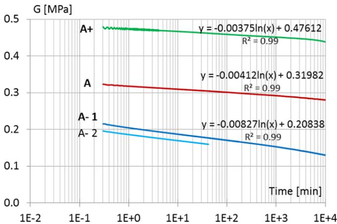
Fig. 5.10 Relaxation moduli for all the compounds tested, calculated by the creep test results of Fig. 5.8.
