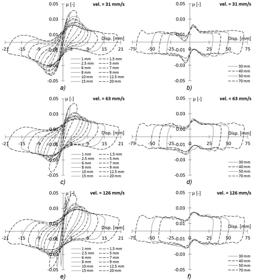
Fig. 6.57  $\mu$ -disp loops. Case: rubber tracks A-A,  $W = 250\text{ N}$ ,  $t_{dw} = 24\text{ h}$ ,  $2^{nd}$  cycle.
