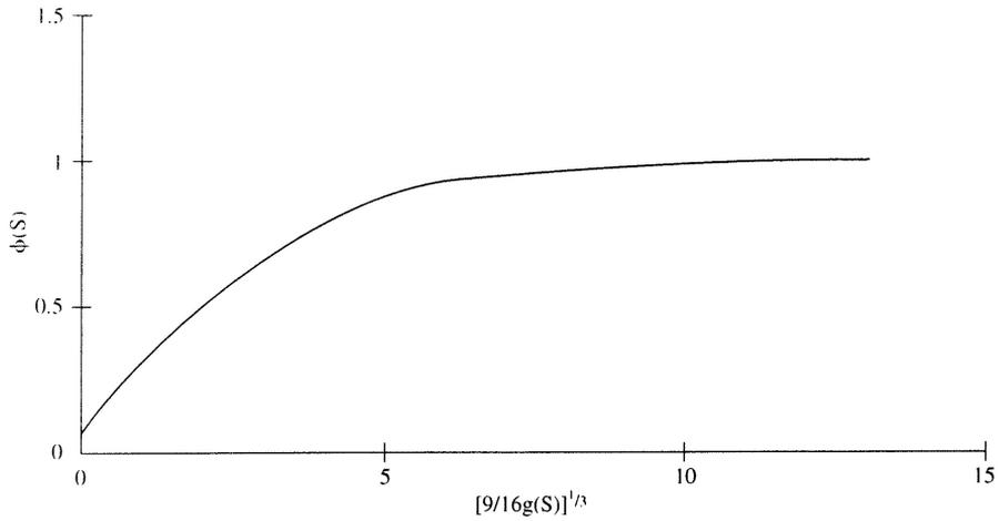
Fig. 3.8 Schematic plot of reduced friction ratio versus reduced rubber thickness (Eq.(3.28), Muhr et al., 1997).
