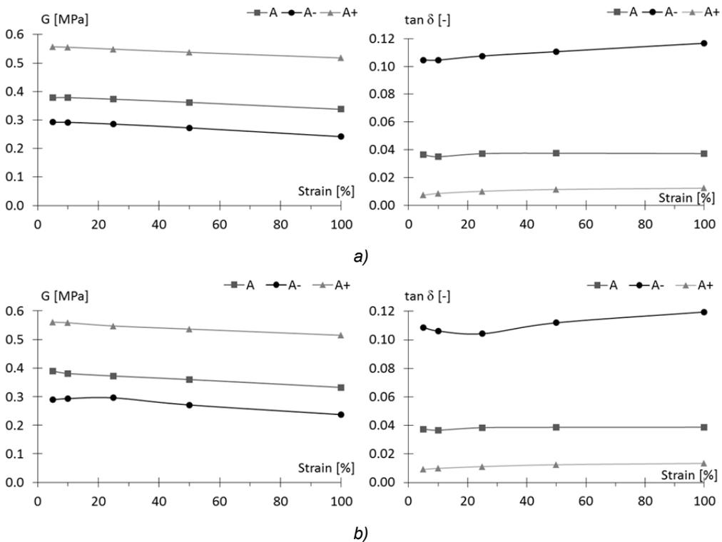
Fig. 5.4 Dynamic shear properties of rubber compounds (A, A+,A-) by Harmonic (a) and Secant (b) linearization method – influence of strain level at 1 Hz frequency.
