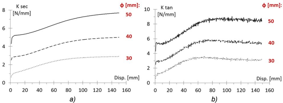
Fig. 5.30 a) Secant stiffness and b) tangent stiffness plots calculated from the results of the quasi-static tests (Fig. 5.29). Values for one spring.
