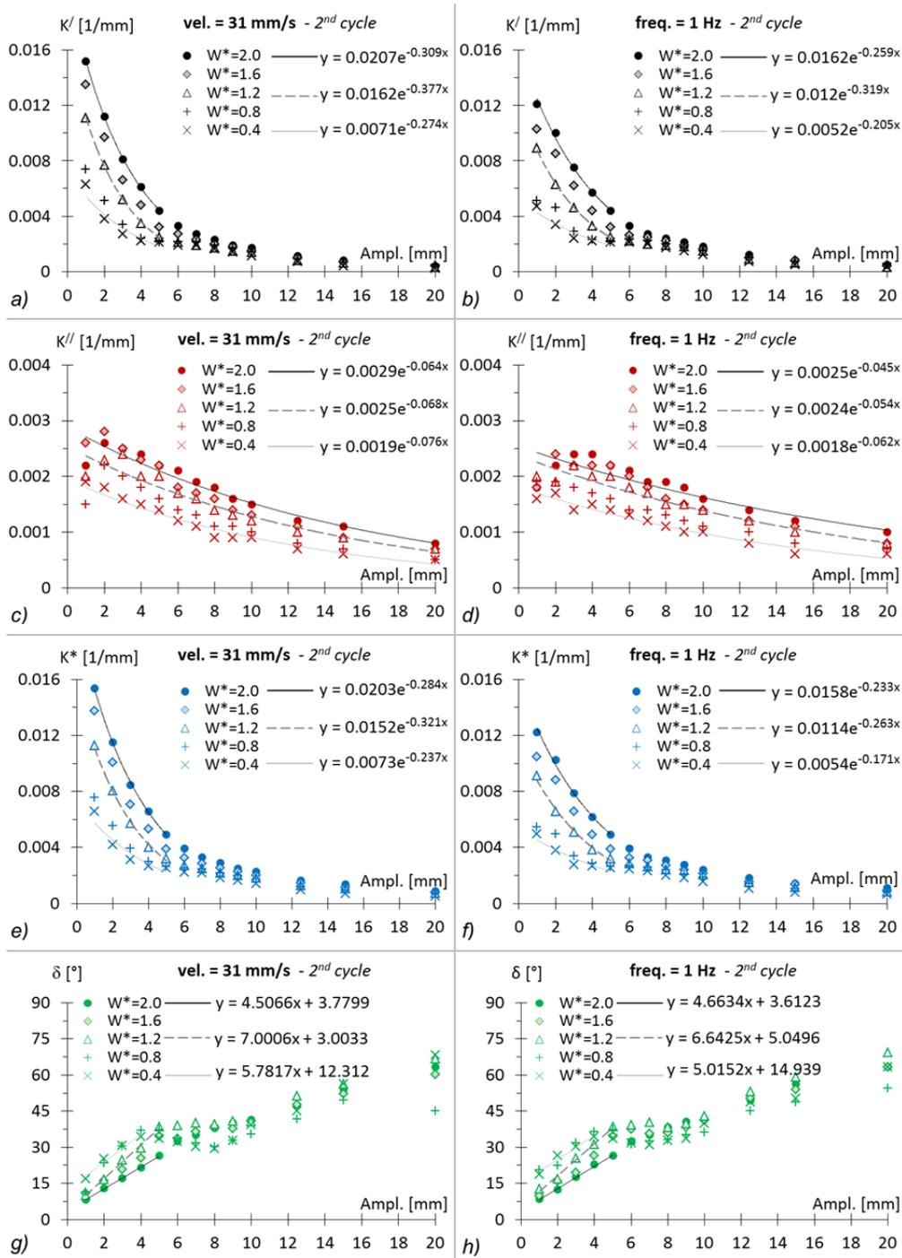
Fig. 6.21 Comparison of  $K'$ ,  $K''$ ,  $K^*$ ,  $\delta$  vs amplitude, for the values of the stress parameter  $W^*$  analyzed. Case: rubber A,  $t=2\text{mm}$ ,  $D=25\text{mm}$  -  $2^{\text{nd}}$  cycle.
