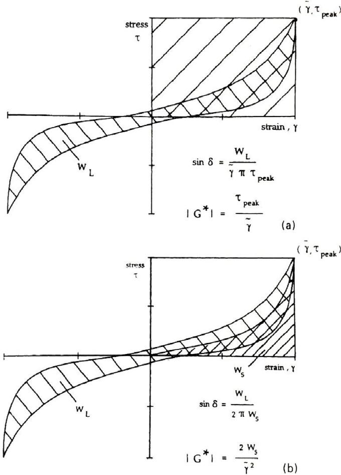
Fig. 3.23 Hysteresis loops showing non-linear behaviour typical of filled rubber at high strain and illustrating: a) Secant method; b) Skeleton curve method (from Ahmadi & Muhr, 1997).
