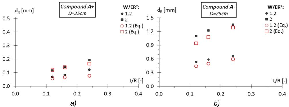
Fig. 6.53 Comparisons between test results and values calculated by Eq. (6.12) for the maximum residual indentation, for different values of  $t/R$  and  $W/ER^2$ , and for the case of rubber A+ (a) and A- (b).
