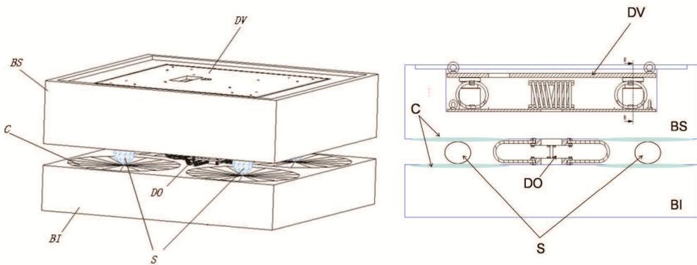
Fig. 2.28 Scheme of the Rolling Double Pendulum device (from De Canio, 2012).
