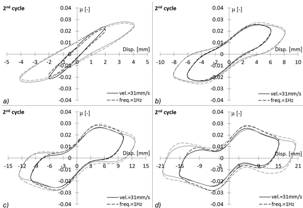
Fig. 6.9 Comparisons of  $\mu$ -disp loops – 2<sup>nd</sup> cycle. Rubber A,  $t=2\text{mm}$ ,  $D=25\text{mm}$ ,  $W/ER^2=2$ .
