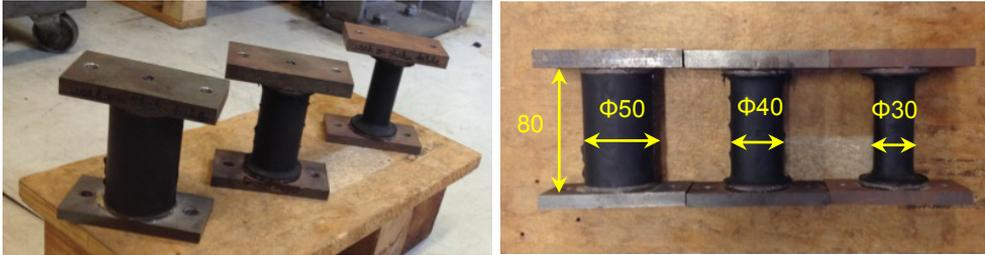
Fig. 5.24 Tested recentering rubber springs; diameter ( $\phi$ ), from left to right: 50, 40, 30 mm.
