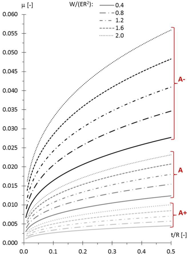
Fig. 5.22 Theoretical  $\mu$  values, calibrated through the experimentation, for each compound (A+, A, A-) and stress parameter ( $W/ER^2$ ) analyzed, on an adequate range of  $t/R$  ratios.
