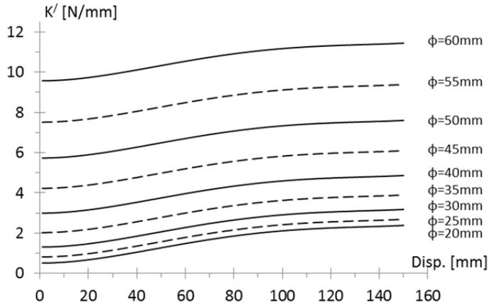
Fig. 5.37 Prediction of the storage stiffness values  $K'$ , using Eq. (5.13).
