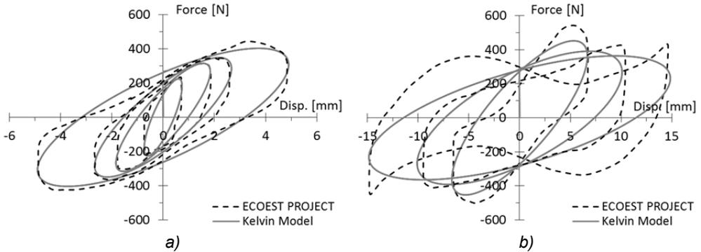
Fig. 4.10 Force-displacement loops obtained for AA tracks during the ECOEST project and compared with equivalent linear viscoelastic representations a) amplitudes up to 5 mm b) amplitudes up to 15 mm.
