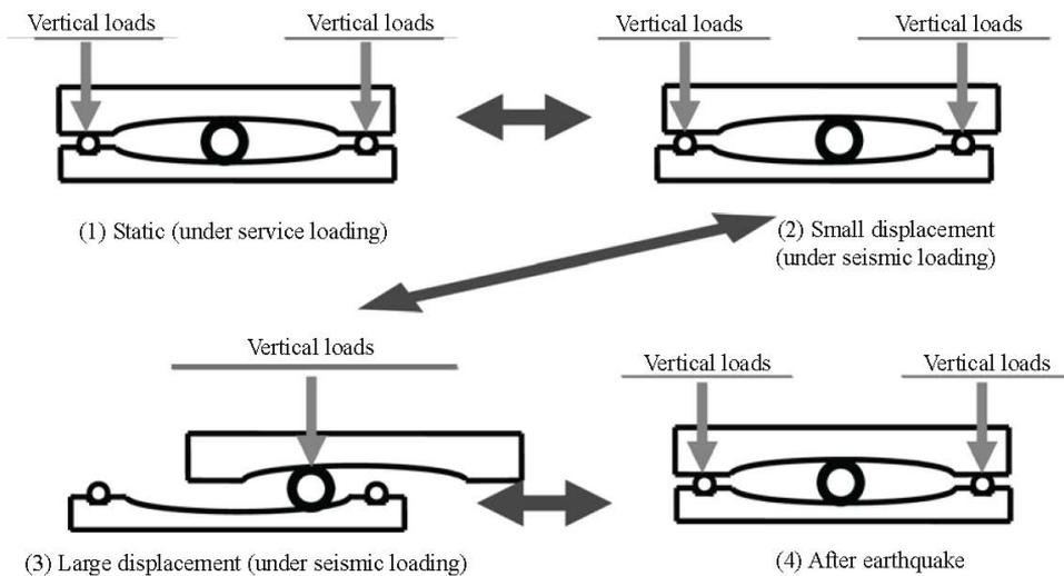
Fig. 2.27 Movements of a SDI-BPS device under service and seismic loadings (from Tsai et al., 2010).
