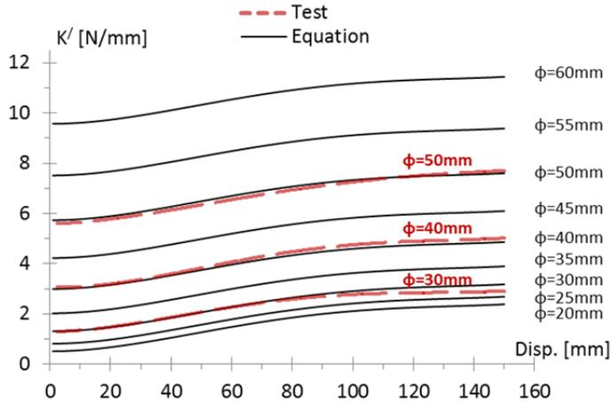
Fig. 5.33 Prediction of the storage stiffness values  $K'$ , using Eq. (5.13), and comparison with the experimental values for the diameters 30, 40 and 50 mm.
