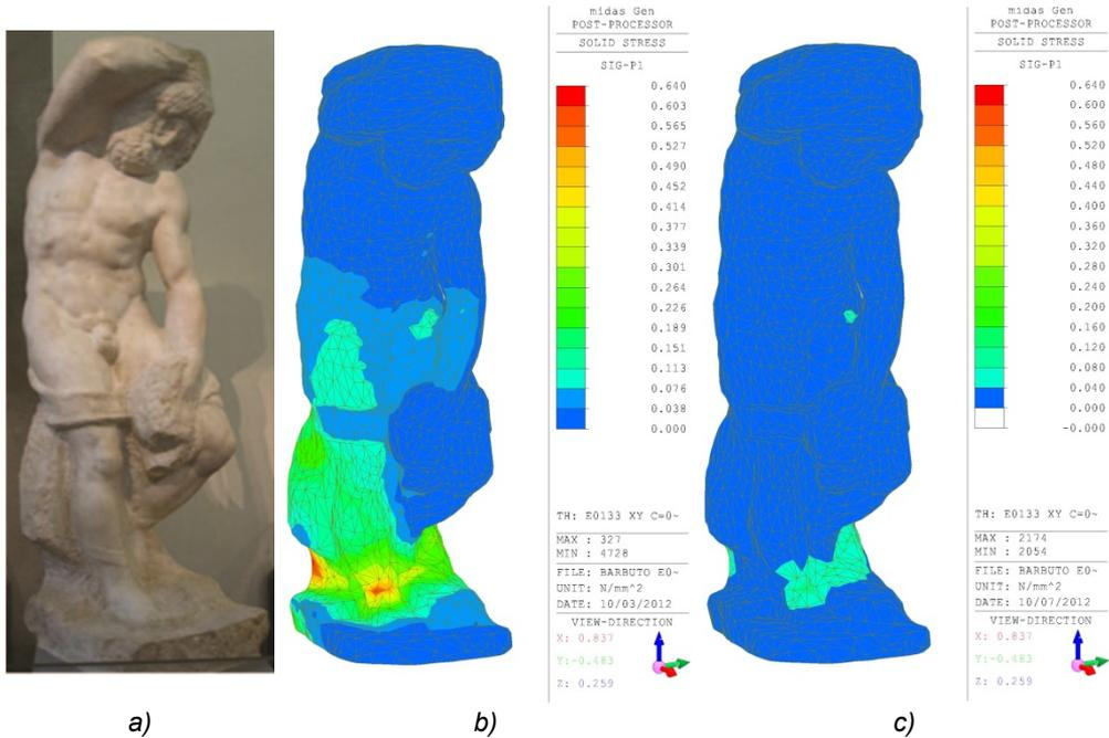
Fig. 2.22 a) Statue “Prigione Barbuto” by Michelangelo. b),c) Finite Element Model of the statue, with the stress field, for the case without b) and with c) seismic isolation (from Baggio et al., 2013).
