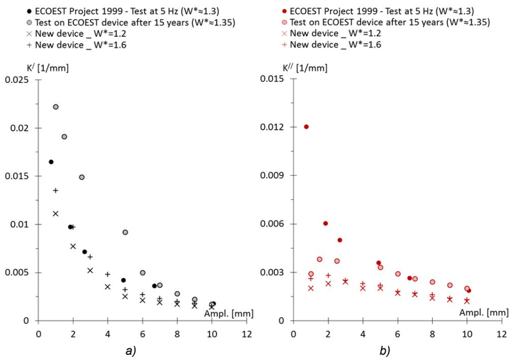
Fig. 6.63 Comparisons of  $K'$  and  $K''$  of the RBRL device with rubber A,  $t = 2\text{mm}$ ,  $D = 25\text{mm}$  between the cases of: sinusoidal shaking-table test performed at 5 Hz during ECOEST project ( $W^* \approx 1.3$ ), new sinusoidal test on the same ECOEST device and with similar  $W^*$  (after 15 years from its production), new sinusoidal tests on a new RBRL device (produced at TARRC for this PhD Project) with values of  $W^*$  of 1.2 and 1.6.
