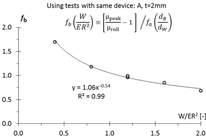
Fig. 6.67 Interpolating function  $f_b$  according to Eq. (6.17).
