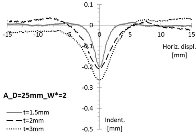
Fig. 6.39 Comparison of the geometric profiles of the residual indentation for the case of rubber A,  $D=25\text{ mm}$ ,  $W^*=2$ , for different thicknesses of the rubber layer ( $t=1.5, 2, 3\text{ mm}$ ).
