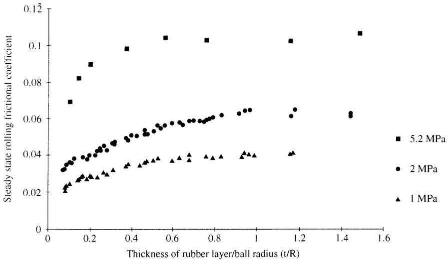
Fig. 3.11 Experimental results for steady-state rolling friction coefficient, versus ratio of rubber layer thickness to ball radius, for three different values of  $W/R^2$  (Muhr et al., 1997).
