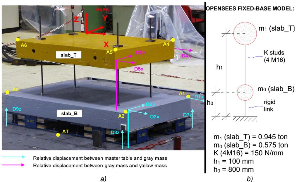
Fig. 4.2 a) Mass Up configuration with indication of the transducers (A = accelerations; D = displacements). b) Relative fixed-base model analyzed in OpenSees for comparisons.
