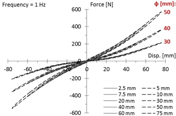
Fig. 5.25 Hysteretic loops from the sinusoidal tests with same frequency, 1 Hz, and different amplitudes; diameters of the springs tested: 30, 40, 50 mm. Values for one spring.
