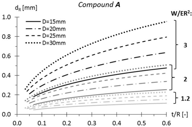
Fig. 6.54 Estimate of the maximum residual indentation  $d_R$  through the Eq. (6.12), after a dwell time of the load of 25 hours, for the rubber A and for a certain range of  $t/R$  and  $W/ER^2$ .
