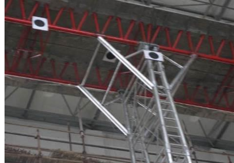
d) Displacement measured point on the column
