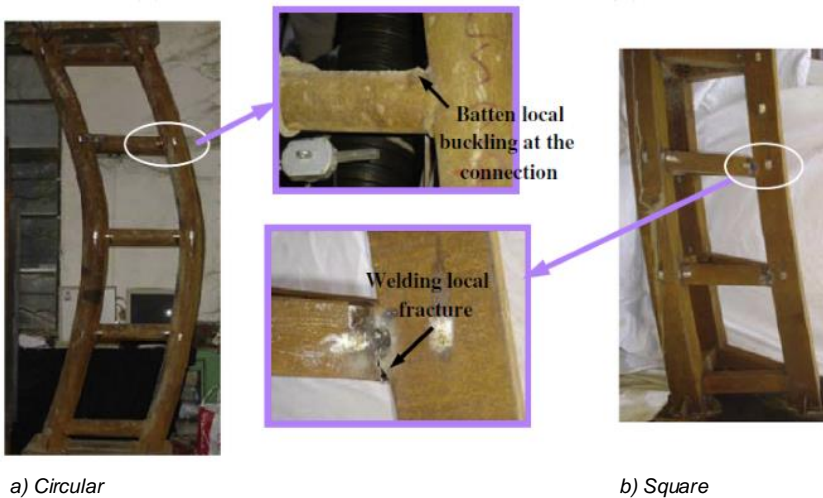
Fig. 19 Failure modes of tested battened specimens (Han et al., 2012)
