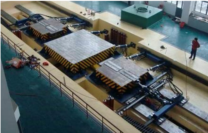
Fig. 114 Panorama of the three bi-axial shaking table array system
