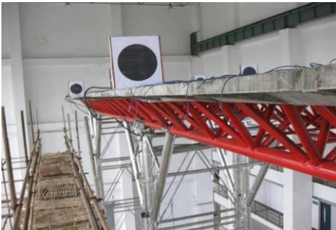
c) Displacement measured point on the deck
