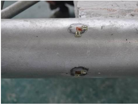
g) Strain gauges on the top of RC web Fig. 122 Details of instruments
