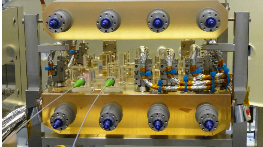
Figure 13: LISA Pathfinder optical bench during integration, courtesy of University of Glasgow.
