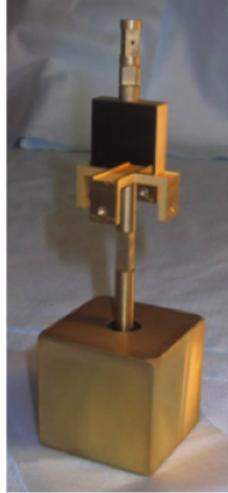
FIGURE 3.2: The real test mass suspended in the torsion pendulum facility.
