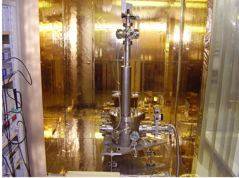
FIGURE 3.4: Torsion pendulum vacuum chamber and the thermal box that surround it.
