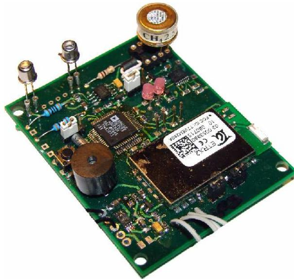
Figure 6.2: Gas sensor module.
