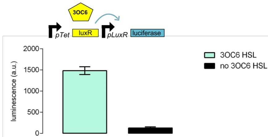
Fig. 4.42 Artificial cells sense 3OC6 HSL.
