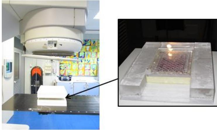
**Figure 16.** Experimental set up used for the irradiation of cell cultures. In the box, the plexiglas phantom used to ensure the electronic equilibrium in cell cultures during the irradiation.
