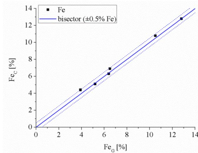
Figure A.6. Average iron concentration calculated with the chemical method vs. average iron concentration calculated with the geometrical method.
