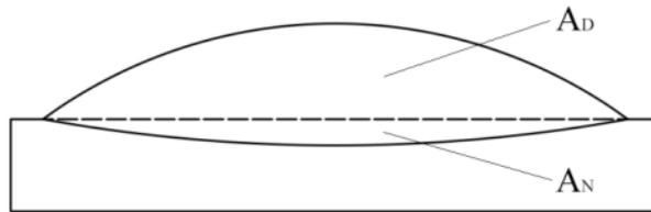
Figure A.4. Schematic representation of  $A_N$  (part of the cross-sectional area emerging from the original surface of the plate) and  $A_D$  (submerged part of the cross-sectional area).
