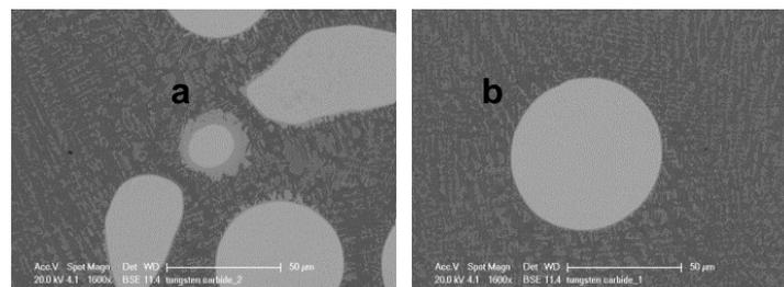
Figure A.2. Classifications of the carbides according to the presence of the interface constituent: tungsten carbide with (a) and without (b) interface constituent.
