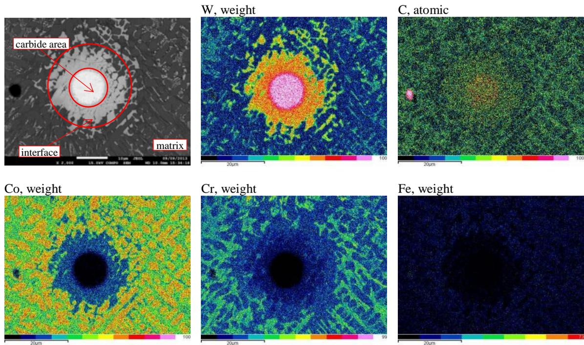
Figure 3.68. EDXS maps for the different elements present into the material.
