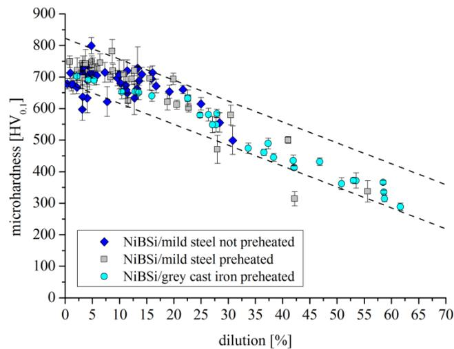
Figure 3.67. Microhardness of the NiBSi clads as a function of dilution.
