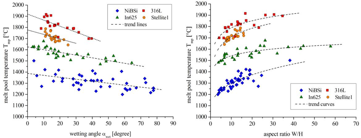
Figure A.14. Estimated melt pool temperature as a function of the wetting angle and the aspect ratio respectively.
