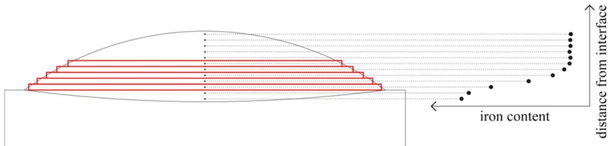
Figure A.3. Schematic representation of the cross-sectional areas used to define the chemical dilution.
