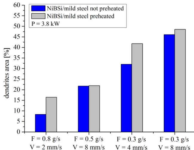
Figure 3.62. Percentage of the dendritic region for clads produced in different conditions.
