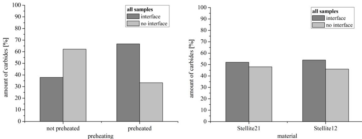
Figure 3.72. Percentage of carbides with and without the interfacial microstructural constituent according to their preheating conditions (left) and to the different base materials (right) for all the samples measured.
