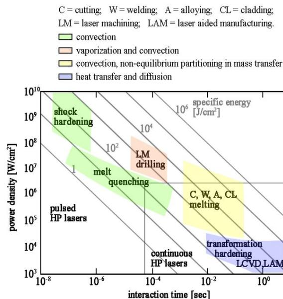
Figure 1.4. Process map for various laser applications in materials processing [50].
