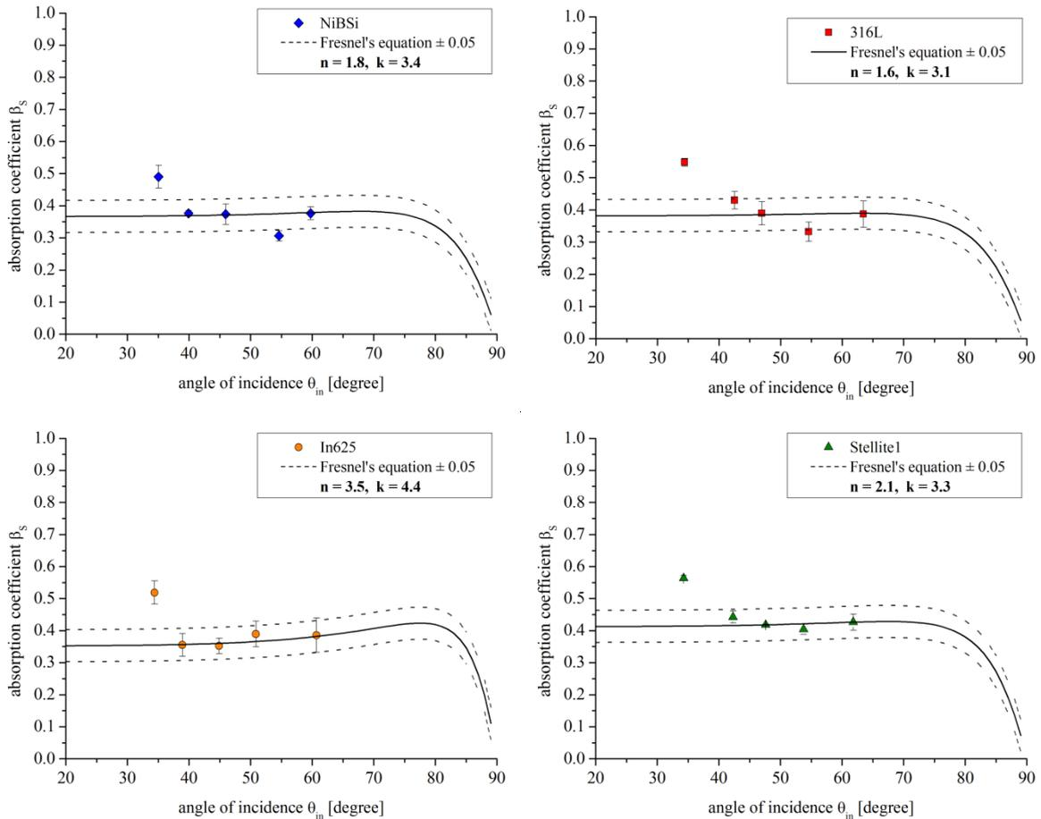
Figure A.11. Measured values of absorption  $\beta_s$  for the four materials together with the estimated Fresnel's curves.
