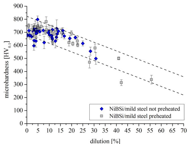
Figure 3.64. Microhardness of the clads produced on the mild steel as a function of dilution.
