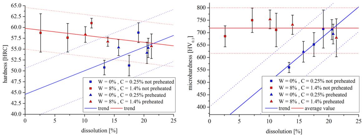
Figure 3.74. Rockwell C Hardness (left) and matrix  $HV_{0.1}$  microhardness (right) as a function of carbides dissolution.
