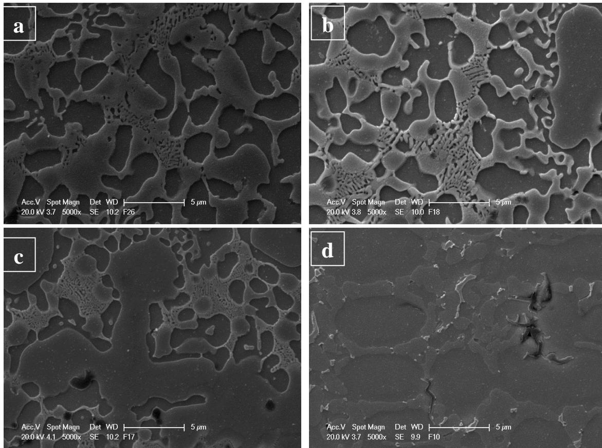
Figure 3.65. Microstructures of the clads produced on the preheated grey cast iron for different values of dilution: (a)  $D = 2.1\%$ , (b)  $D = 16.0\%$ , (c)  $D = 27.7\%$  and (d)  $D = 58.7\%$ .
