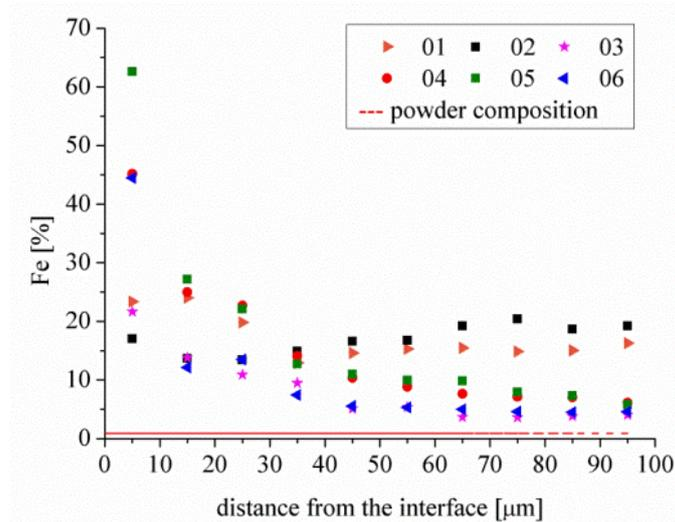
Figure A.5. EDXS iron concentration profiles of six clad investigated in different processing conditions: laser power ranging from 3 to 4 kW, scan speed ranging from 3 to 4 mm/s, feeding rate ranging from 0.5 to 0.6 g/s.
