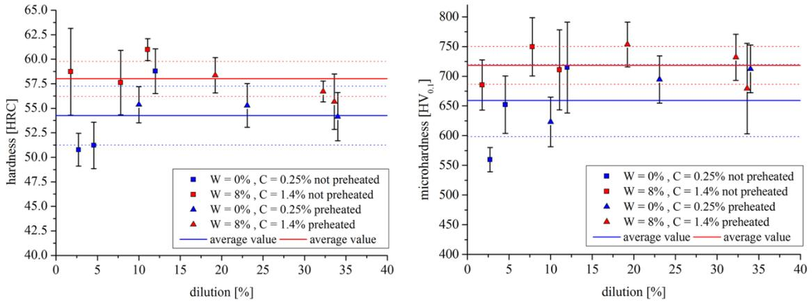
Figure 3.73. Rockwell C Hardness (left) and matrix  $HV_{0.1}$  microhardness (right) as a function of dilution.
