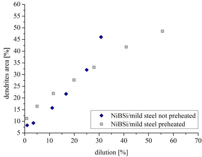
Figure 3.61. Percentage of the dendritic region as a function of clad dilution.
