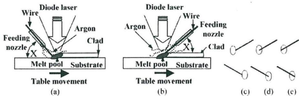
Figure 1.15. Possibilities of wire feed angles and positions: (a) leading wire, (b) trailing wire, (c) wire tip not crossing the melt pool (d) wire tip in central position (e) wire tip crossing the melt pool [74].
