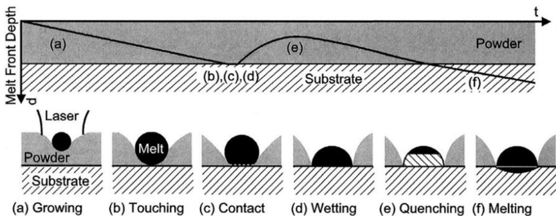
Figure 1.9. Contact history between melt, powder and substrate [61].
