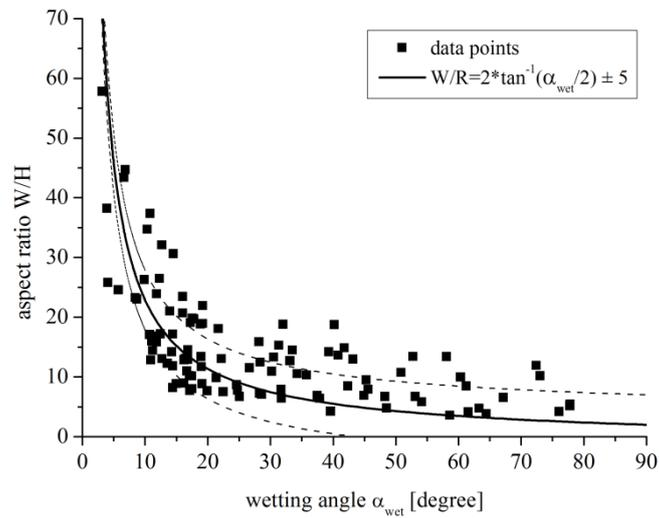
Figure A.15. Aspect ratio values as a function of the wetting angle plotted together with equation (A.19).
