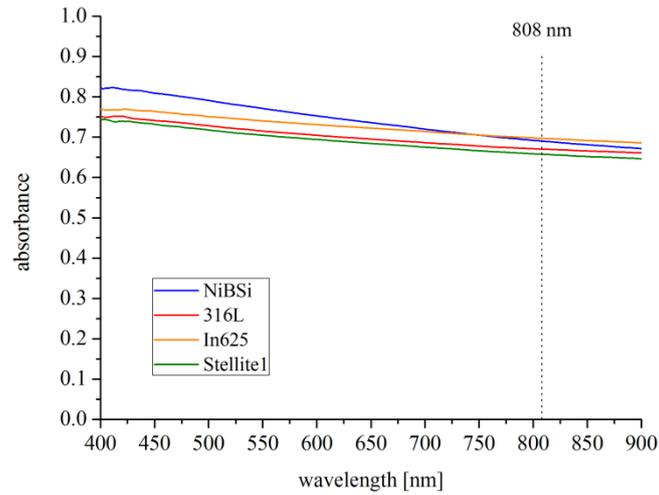
Figure A.13. Spectral absorbance in the visible region for the different powders.
