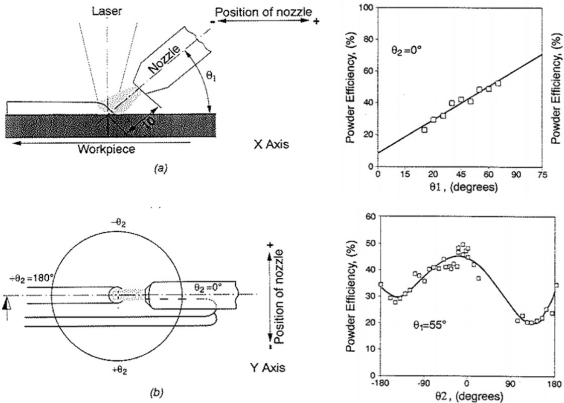
Figure 1.12. Schematic of blown powder laser cladding showing (a) the longitudinal section with the inclination  $\theta_1$  and its influence on the powder efficiency and (b) a plan view of the clad surface with the orientation  $\theta_2$  and its influence on the powder efficiency [67].
