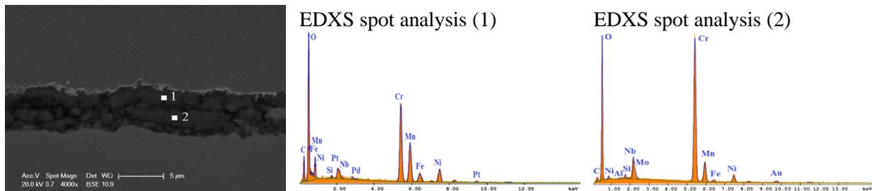
Figure 3.56. Oxide scale formed at  $1100^\circ\text{C}$  and respective EDXS analysis.
