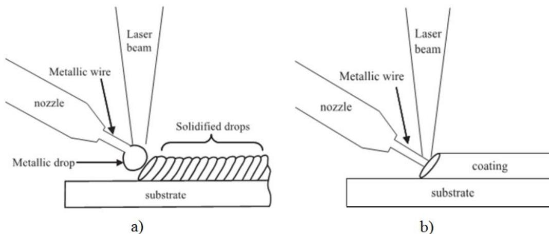
*Figure 1.13. Schematic of laser cladding with wire/strip feeding in (a) drop by drop configuration and (b) classical configuration [73].*
