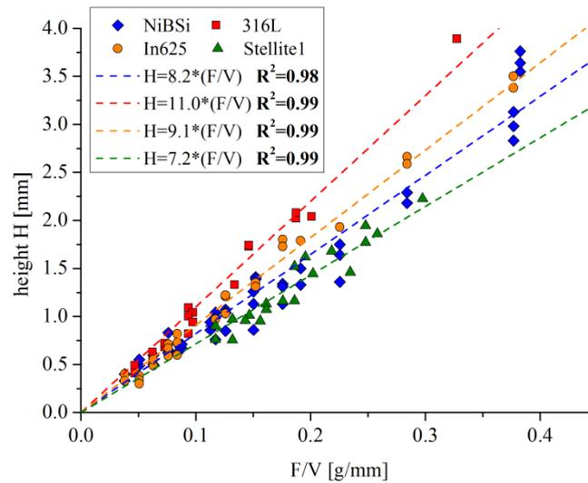
Figure 3.2. Correlations between clad height and  $F/V$  for different powders.
