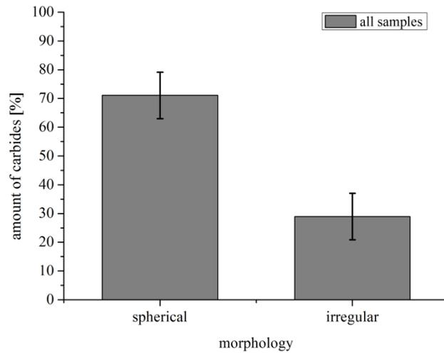
Figure 3.70. Average percentage of spherical and irregular carbides according to their morphology for all the samples measured.
