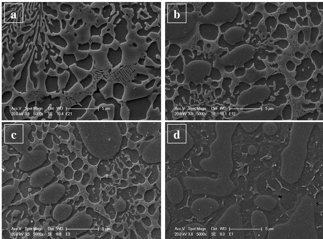
Figure 3.58. Microstructures of the clads produced on the preheated mild steel for different values of dilution: (a)  $D = 0.8\%$ , (b)  $D = 19.9\%$ , (c)  $D = 28.0\%$  and (d)  $D = 55.6\%$ .
