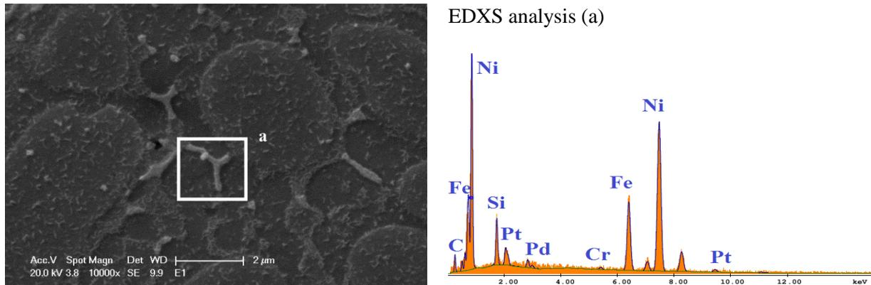
Figure 3.63. Morphology and EDXS analysis of the silicon-rich eutectic formed when dilution is high.
