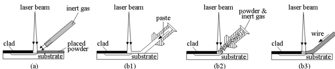
Figure 1.8. Different methods of laser cladding: (a) two-step laser cladding, (b) one-step laser cladding with (b1) paste, (b2) powder injection and (b3) wire feeding [11].
