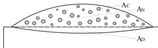
Figure A.1. Schematic drawing of the clad cross-sectional area: emerging cross-sectional area ( $A_N$ ), submerged cross-sectional area ( $A_D$ ) and area of the carbides in the cross-sectional area ( $A_C$ ).
