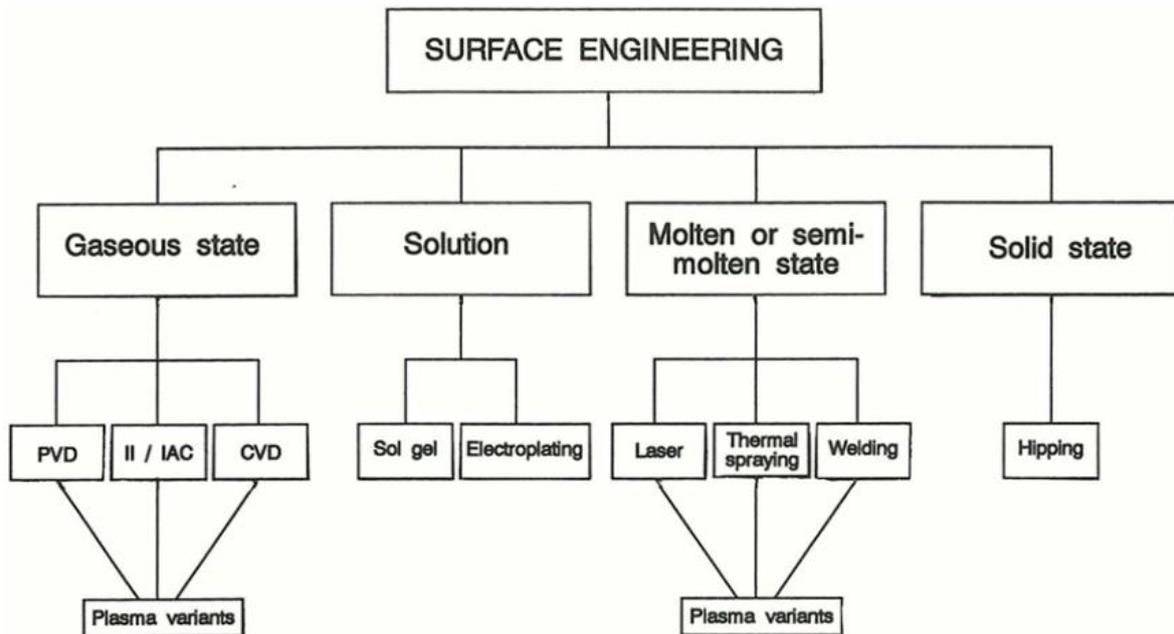
Figure 1.1. Classification of surface engineering techniques depending on the state of the depositing phase [5].
