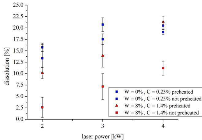
Figure 3.69. Carbides dissolution as a function of the laser power for the different materials, preheated and not.
