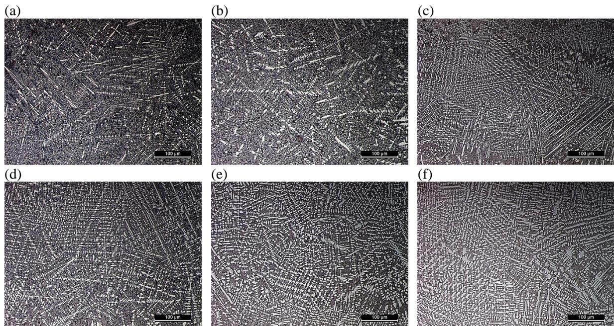
Figure 3.60. Microstructures of the clads produced on the preheated mild steel with different dilution: (a)  $D = 0.8\%$ , (b)  $D = 5.0\%$ , (c)  $D = 11.6\%$ , (d)  $D = 19.9\%$ , (e)  $D = 28.0\%$  and (f)  $D = 41.0\%$ .
