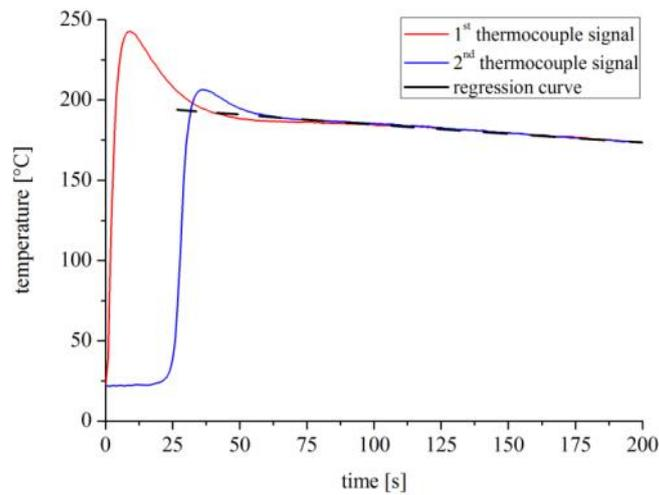
Figure A.9. Temperatures recorded by the two thermocouples in one of the run and regression curve.
