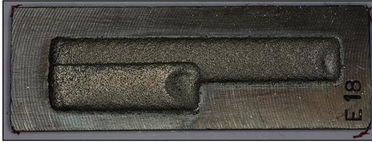
Figure 2.2. Typical sample produced showing the selected cladding strategy
