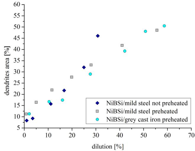
Figure 3.66. Percentage of the dendritic region as a function of clad dilution.
