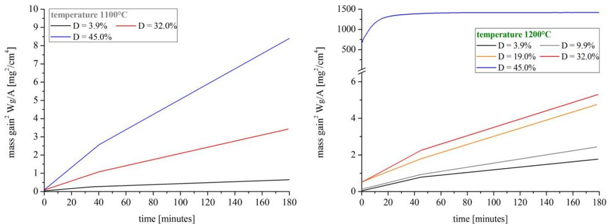
Figure 3.50. Thermogravimetric curves at 1100°C (left) and 1200°C (right) for different values of clad dilution.
