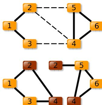
Figure 9.1: Example of vertex and edge partitioning: on the top figure, vertices are partitioned and a few *cut edges* connect vertices belonging to different partitions. On the bottom figure, edges are partitioned and a few *frontier vertices* appear in more than one partition
