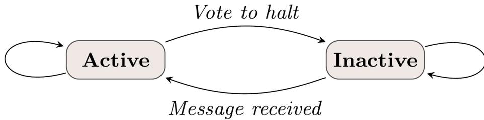
Figure 8.1: Vertex's state machine in PREGEL (from [70])
