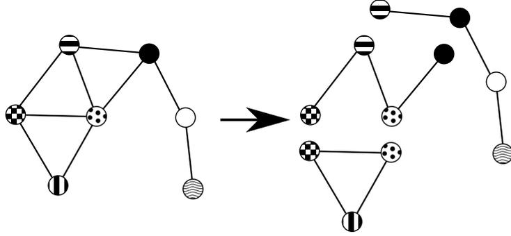
Figure 6.3: Edge partitioning example: each edge appears in only one partition, while frontier vertices may appear in more than one partition
