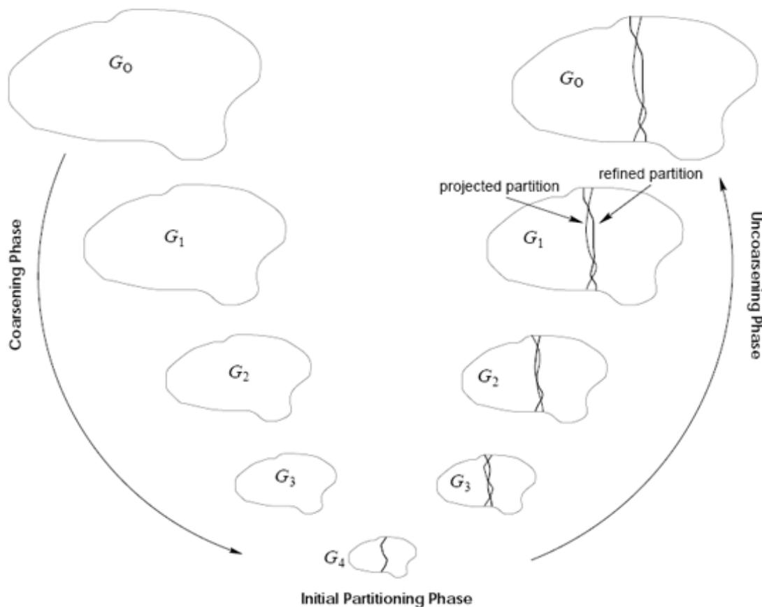
Figure 6.5: Illustrative scheme of multilevel partitioning algorithms, from <http://masters.donntu.org/2006/fvti/shepel/diss/indexe.htm>
