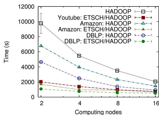
Figure 9.3: Running time of single source shortest path algorithm in HADOOP comparing a standard baseline algorithm and ETSCHE, with `m3.large` machines on EC2.
