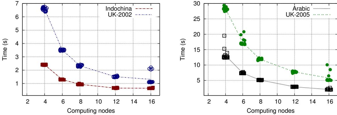
Figure 9.5: Scalability of ETSCH/AKKA on the larger datasets, using `m3.large` machines on EC2. For each experiment we measure the average time for a complete iteration of PageRank
