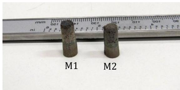
**Figure 7.1.1:** Brake pad pins from the two different friction materials, M1 & M2.
