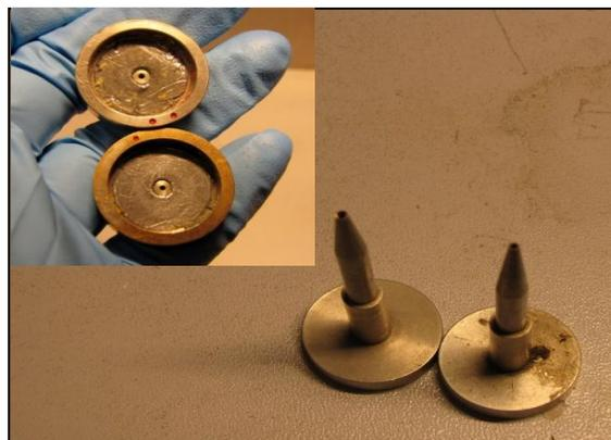
**Figure 7.4.5:** Different size of incoming X-Ray beam collimators.
