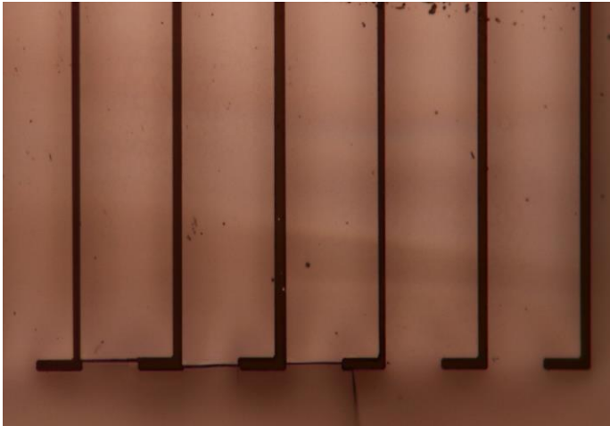
Figure. 4.13. Optical micrograph of the under-etched Si microwires before transferring to secondary substrate by a PDMS stamp.
