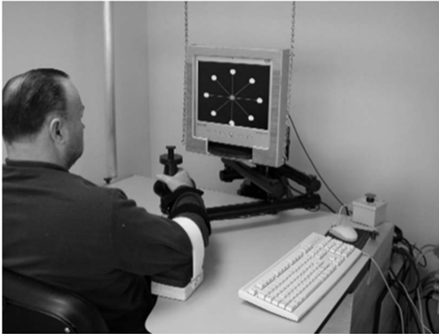
Figure 1: InMotion2 robot: a subject is shown performing robot-aided exercises. A cursor on the display corresponds to the position of the hand, and each target is highlighted sequentially as a goal for the subject to reach toward.
