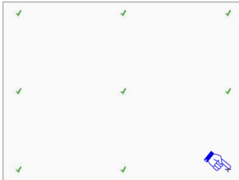
Figure 27: Calibration targets appear on the screen. Apply and hold a touch in the centre of each displayed target in the sequence they are displayed on the screen
