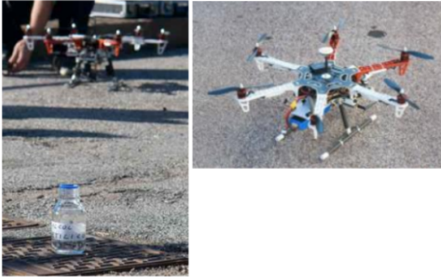
Figure 5.7: Pictures of the UAV carrier (hexacopter with 80 cm diameter) and gas source taken during tests on the field.
