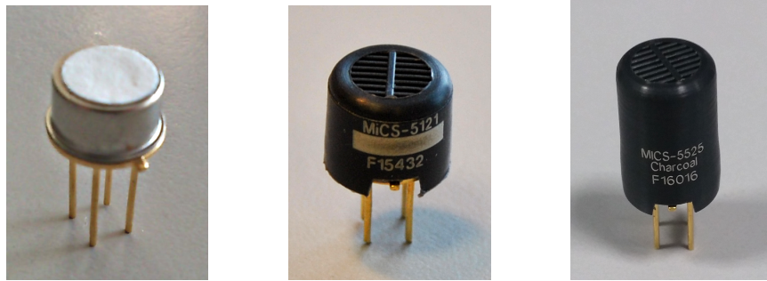
Figure 3.1: AS-MLK Natural Gas sensor [8] (left), MICS-5121 CO/VOC sensor [2] (center) and MICS-5525 CO/VOC sensor [3] (right).
