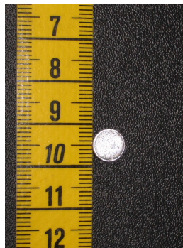
Figure 5.17: Marker used to monitor head position.
