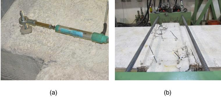
**Figure 9.3:** Visual damage observations corresponding to (a) DS3, and (b) DS4, respectively
