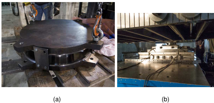
Figure 4.16: View of the CSB: a) CSB during positioning phase; b) CSB positioned under the BTS.
