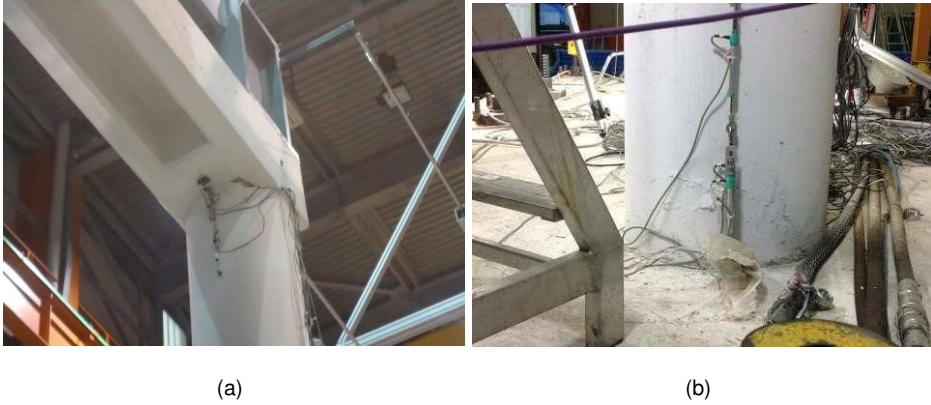
Figure 3.33: Cracks opening at the top and bottom of Pier #11 after test k09.
