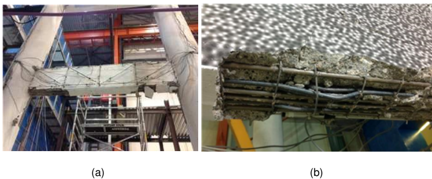
Figure 3.36: Damage in the Pier #11 after k12 test: a) transverse beam damage on Pier #11; b) blow up of the transverse beam.
