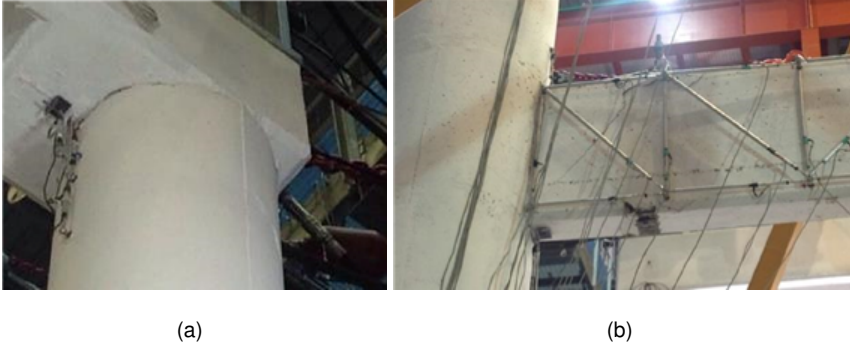
Figure 3.37: Damage after k12 test: a) cracks opening at the top of a column in Pier #11; b) cracks pattern in the first transverse beam in Pier #9.
