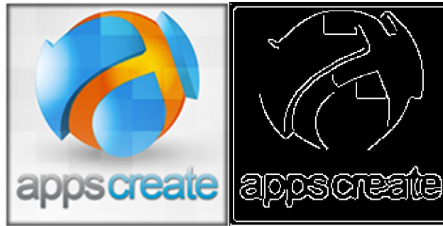
Figure 31. Icon contour detection. Contour pixels are counted and taken as an estimate of amount of detail.
