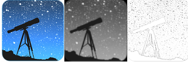
Figure 35. Frequency filtering. The central image is processed with a low-pass filter; the right image - with a high-pass filter.
