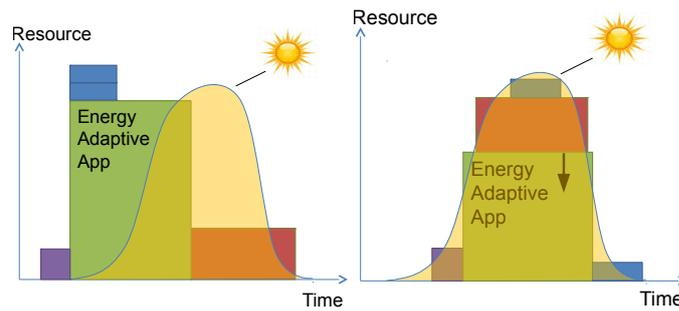
Figure 1.1: Adapting applications for a better usage of renewable energies
