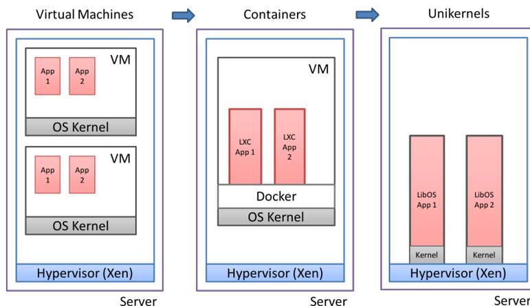
Figure 7.1: Evolution of virtualization vehicles: VMs, containers, Unikernels
