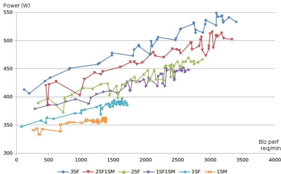
Figure 5.6: Business Performance (Req/min) versus power consumption (W) for each working mode
