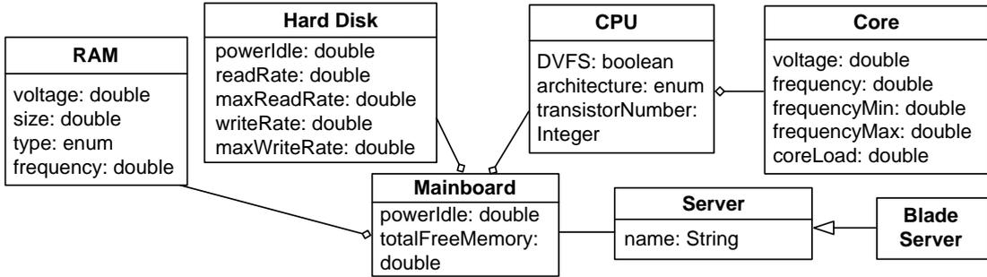
Figure 4.3: Server UML class diagram
