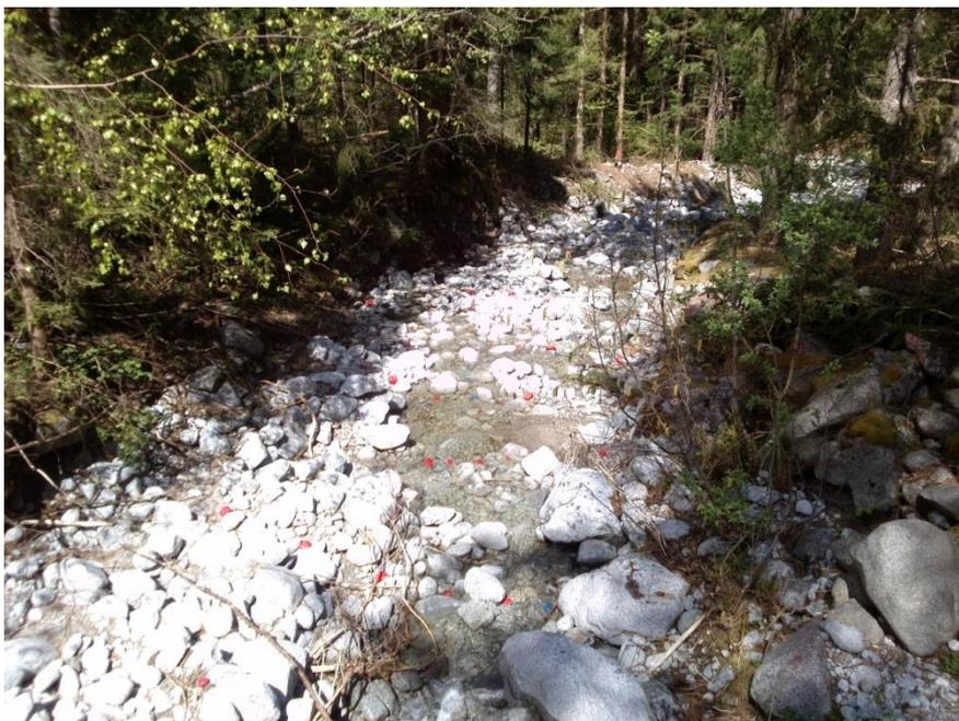
Figure 3.13. Release of tracers at Ussaia site: ribs are spaced 2 m apart and each row spans across the entire section.
