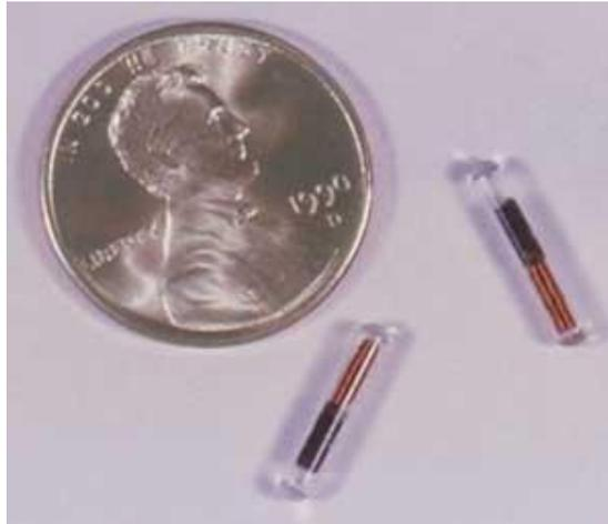
Figure 3.12. Passive Integrated Transponders consisting of a glass-encapsulated copper coil, inserted into drilled stones to allow detection after floods.
