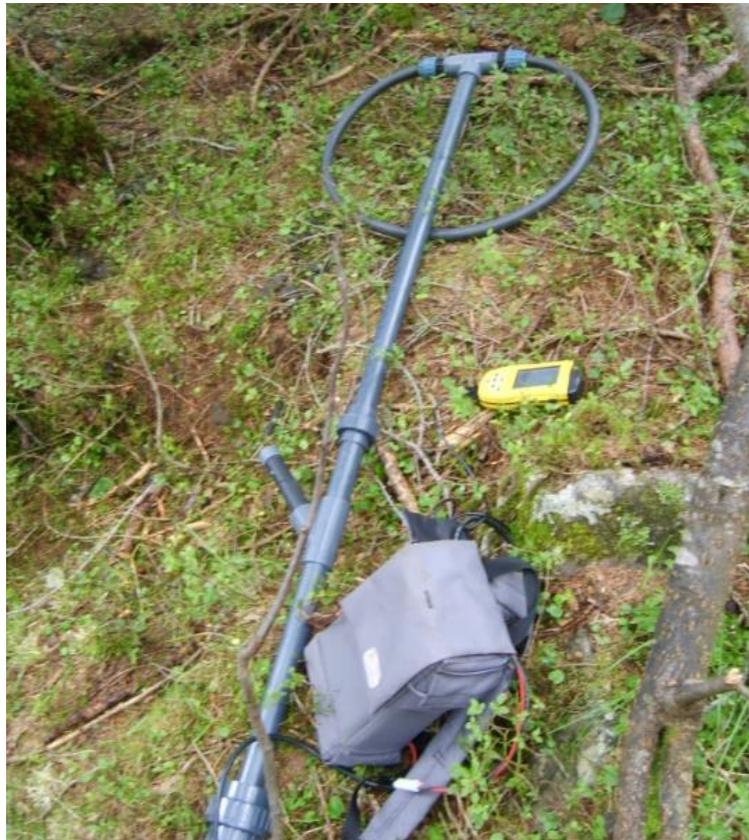
Figure 3.14. Mobile antenna manufactured by Oregon RFID by means of which bedload monitoring surveys have been conducted. In the picture is visible the palmtop where clasts ID are displayed (yellow device), and the grey backpack, where the portable reader/datalogger is located.
