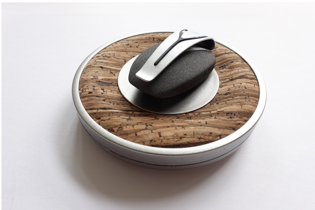
Figure 4.5: Final version of the sensor on the wireless charging pad.
