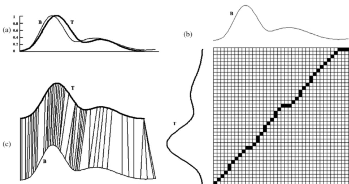
Figure 2.4: An example of the DTW algorithm. Taken from [104].
