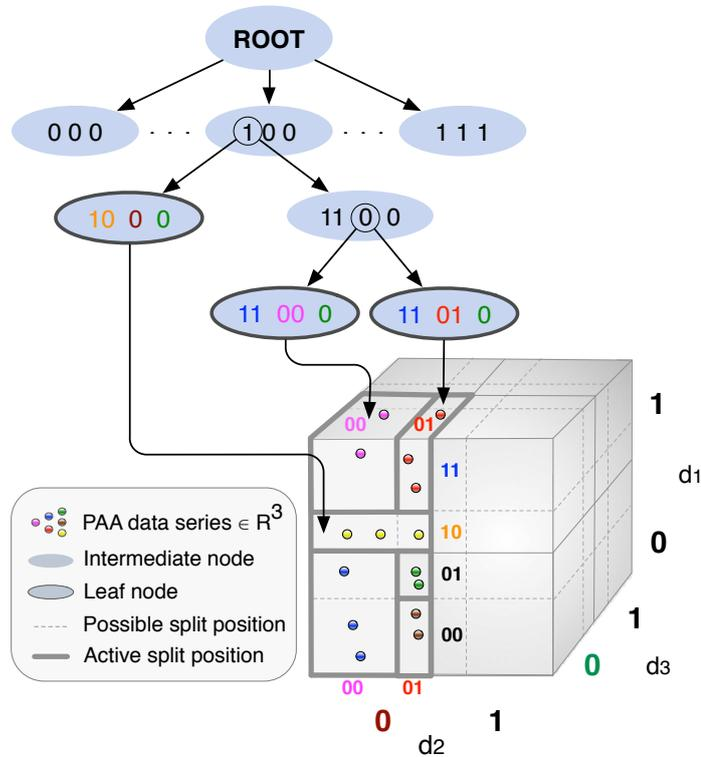
Figure 2.6: An example of iSAX and its space partitioning.
