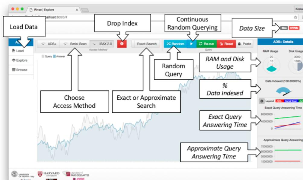
Figure 5.3: RINSE interface components explanation.
