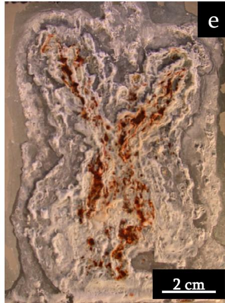
**Figure 2.36** Scratched samples after: Silane HT120+PW (a), Silane HT180+PW (b), untreated galvanized steel+PW (c), Commercial silane+PW (d), ZTF+PW (e).
