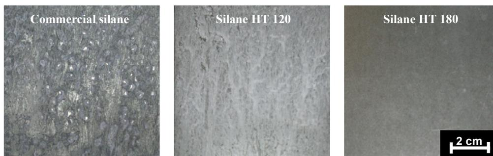
**Figure 2.27** Appearance of the samples after 24 hours of exposure in the salt spray chamber
