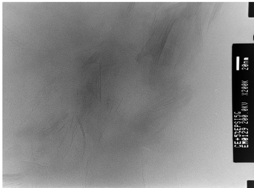
**Figure 3.35** TEM images of the exfoliated structure of sample CL2\_10
