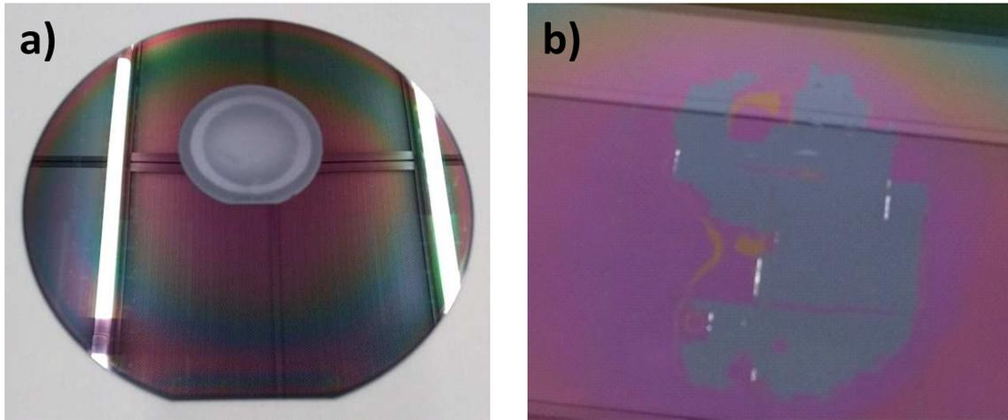
**Figure 1.40:** a) InP wafer bonded on the patterned SOI wafer and b) III-V layer after the substrate removal. The III-V device layer was partially detached during the substrate etching, but left large intact areas.
