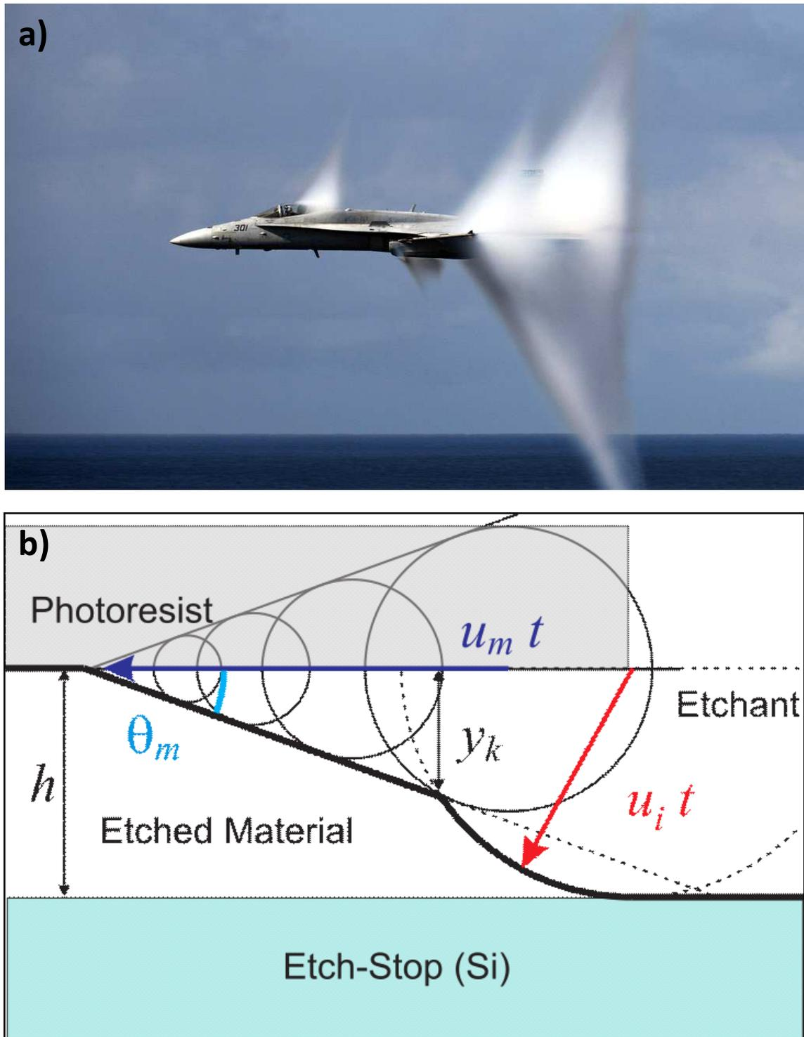
**Figure 5.2:** a) An F/A-18C Hornet breaks the sound barrier, forming a wavefront with the characteristic Mach angle [176]. b) Sketch of the Mach-angle profile formation in the general case when the etching begins isotropically with  $u_i$  and has a wedge asymptote. The relevant quantities  $u_i$ ,  $u_m$ ,  $\theta_m$  are highlighted in colors.
