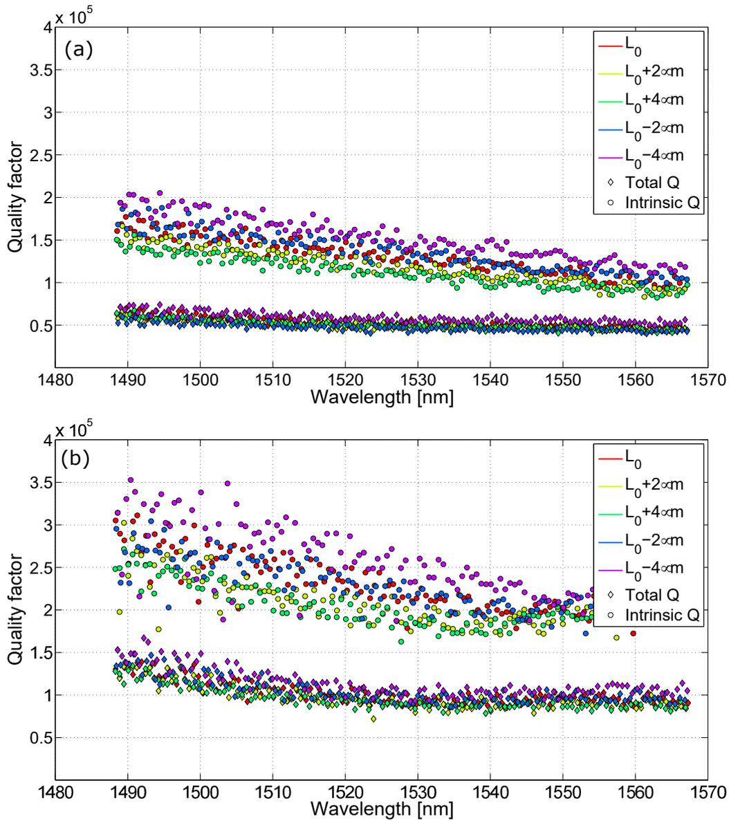
**Figure 2.25:** Quality factor estimations obtained by fitting the resonances of a (a) TEOS sample and a (b) PECVD sample. The measure refers to series of five racetrack resonators with  $l_w = 2400 \text{ nm}$ ,  $R = 350 \mu\text{m}$  and  $2\mu\text{m}$  step variations around the designed critical coupling length designed for IR.
