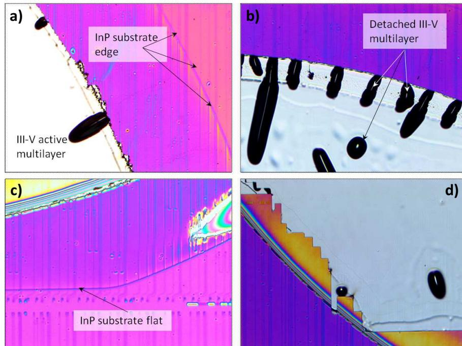
**Figure 1.36:** Optical images of the bonded III-V substrate. Panel a) show footprint of the substrate in the BCB. The same footprint is also present in panel c) where the flat of the III-V wafer is aligned to the structures of the SOI wafer. b) the active layer is partially detached near the borders or c) partially etched.
