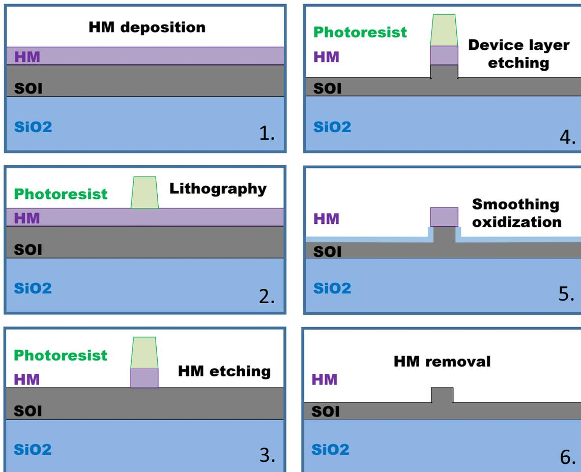
**Figure 1.10:** Process flow for the realization of the devices. The SOI layer is covered with a HM layer and then with photoresist, that is patterned using stepper lithography. The pattern is transferred from the photoresist to the HM using RIE, and then again from the HM to the SOI using RIE. After the pattern definition, the photoresist is removed and the structures are smoothed using wet chemical oxidization. The oxide layer and the HM are then removed, leaving bare the smoothed structures.
