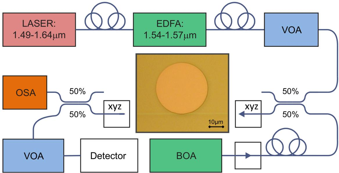
**Figure 3.11:** Experimental setup for the non-linear experiment. A Tunable laser, amplified with an Erbium Doped fiber Amplifier (EDFA), is mixed with the broadband signal of a Boosted Optical Amplifier (BOA) and shined into the sample with a taper fiber. The output is also collected with a taper fiber, split and fed to an Optical Spectrum Analyzer (OSA) and a broadband germanium detector to measure the probe and the pump spectra respectively.
