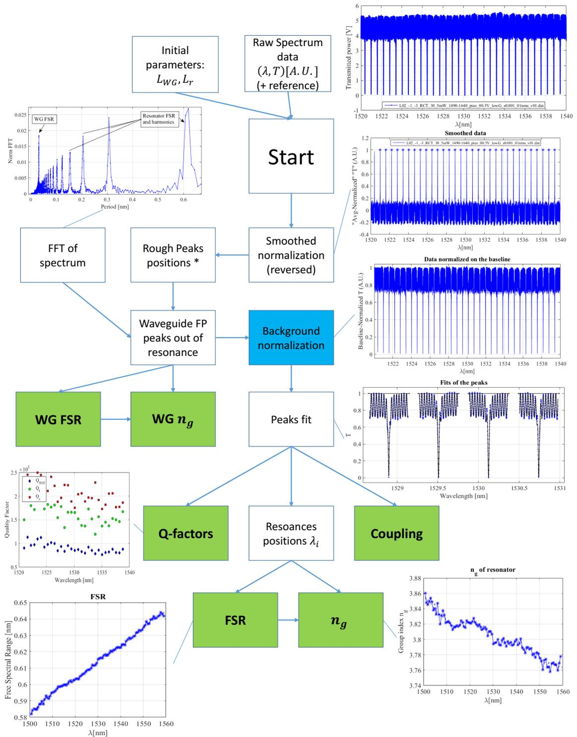
**Figure 13:** Flowchart of the "TrovaPicchi" resonator transmission analysis routine that was developed during this thesis work. This routine, with slight variations, has been used in Chapters 1, 2 and 4 to analyze the response of single-mode ring resonators.
