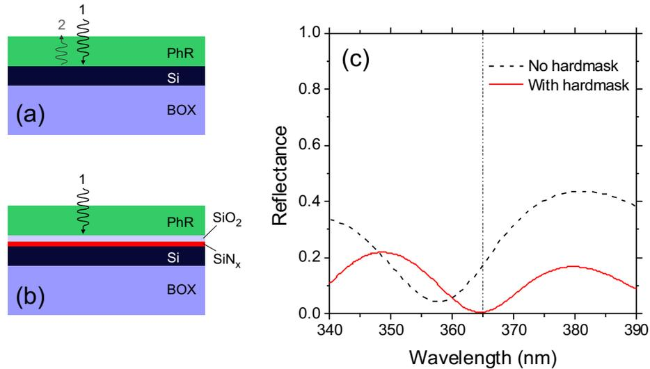
**Figure 1.19:** (a) the UV light of the lithography patterning is partially reflected at the material interfaces between the layers, modifying the light pattern inside the photoresist. (b) a HM with a sufficient number of layers may be used to realize an anti-reflection coating. (c) making use of transfer-matrix simulations, the reflectance of the anti-reflection HM may be brought to 0.
