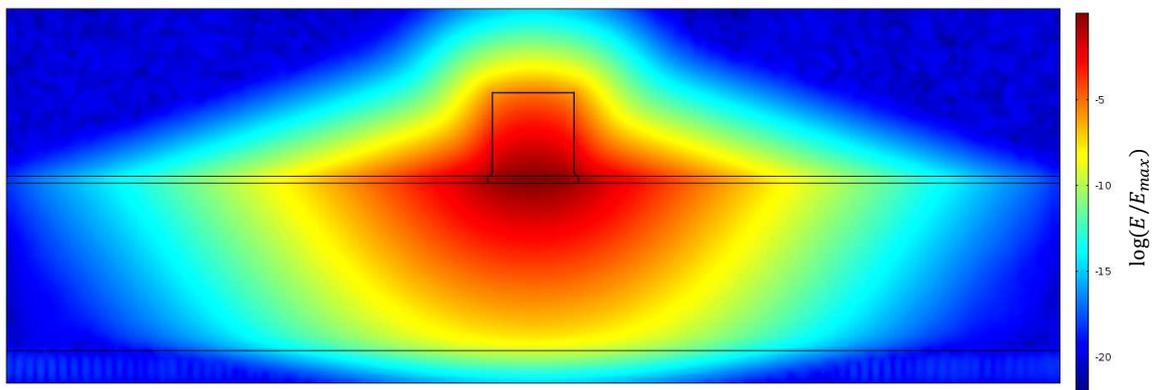
**Figure 2.12:** Mode intensity profile, normalized to the maximum, in logarithmic scale. The figure refers to an IR waveguide, where the mode is pushed out of the slab due to the sub-optimal slab thickness, providing with long evanescent tails that extend down in the cladding to the silicon.
