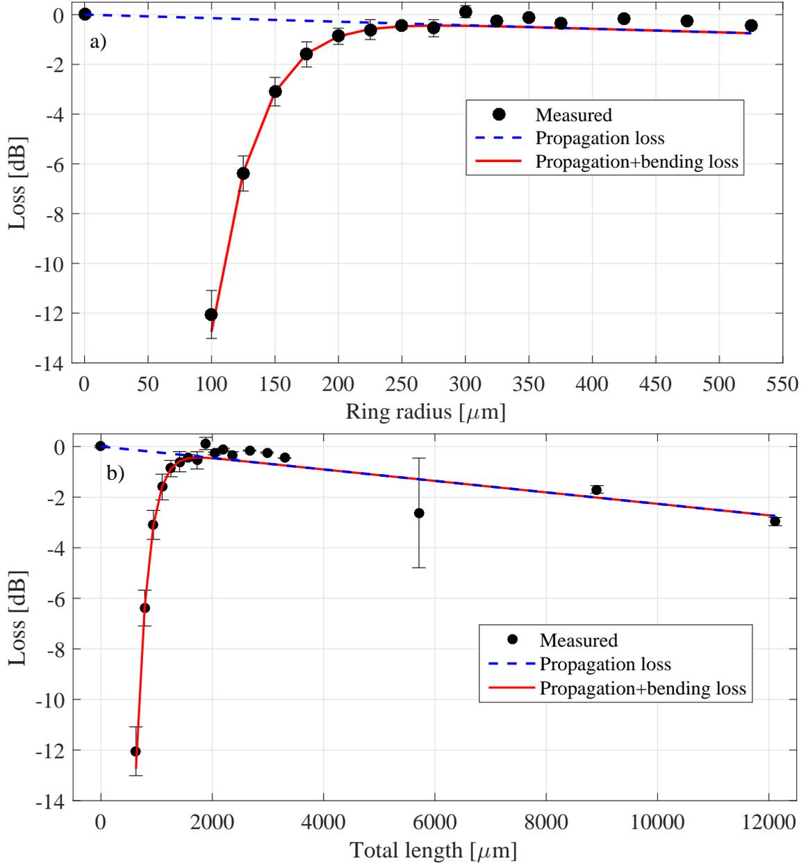
**Figure 2.20:** Transmission measurement of the S-bend waveguides samples for the TEOS-loaded samples in the IR region reported as a function of (top) curvature radius and (bottom) total waveguide length. The errorbars on the data represent the standard deviation over three samples. The red line represents the fit of the data using Eqs. 1.5 and 2.6. The result of the fit is reported in Tab. 2.4.
