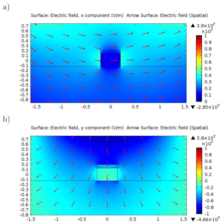
**Figure 4.6:** Electric field intensity and direction for the (a) TE and (b) TM configurations of the low-frequency electric field with an applied tension on the pads of 30V.
