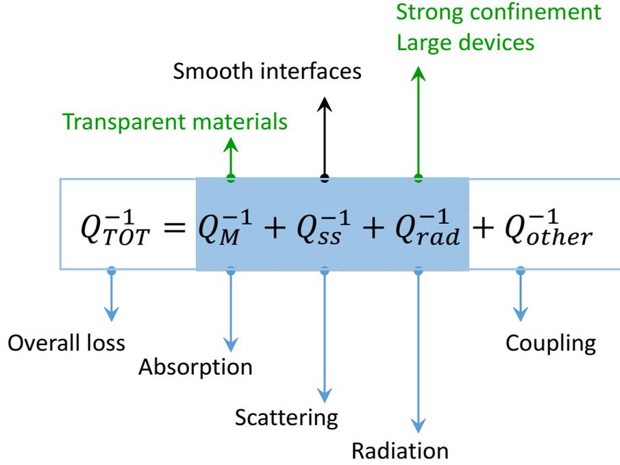
**Figure 2.1:** The total quality factor of a cavity may be expressed as an inverse sum of various contributions: material absorption, surface scattering, radiative losses, mainly due to bending and coupling losses. The first three terms, highlighted by the box, constitute the intrinsic quality factor, while the last contribution,  $Q_{other}$ , is controlled by the coupling design.
