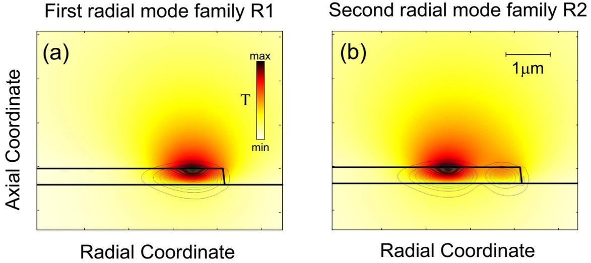
**Figure 3.9:** FEM simulations of the thermal fields  $\mathcal{T}(r)$  generated by (a) the first and (b) the second optical radial family modes. The contour lines show the electric field profiles of the respective optical mode, which are considered the source of heating within the resonator and the cladding materials. The color-map represents the temperature variation induced by the modes with respect to the room temperature.
