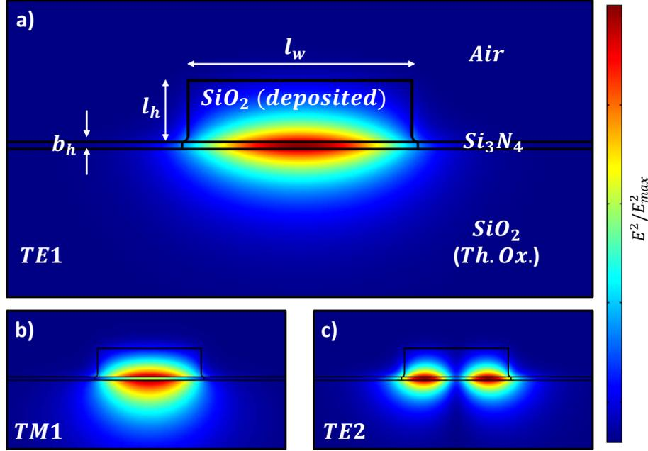
**Figure 2.9:** a) TE1 b) TM1 and c) TE2 SL-guided modes simulations. The images refer to the top-right point of Fig. 2.8 with waveguide parameters  $l_w = 4 \mu\text{m}$ ,  $b_h = 130 \text{ nm}$ , and  $l_h = 1.1 \mu\text{m}$  at a wavelength value of  $1550 \text{ nm}$ .
