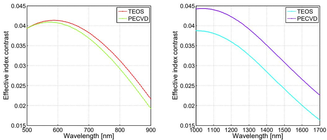
**Figure 2.18:** FEM simulations of  $\Delta_{\text{eff}}(\lambda)$  calculated using the geometrical parameters obtained from SEM imaging and considering both TEOS and PECVD dispersions.
