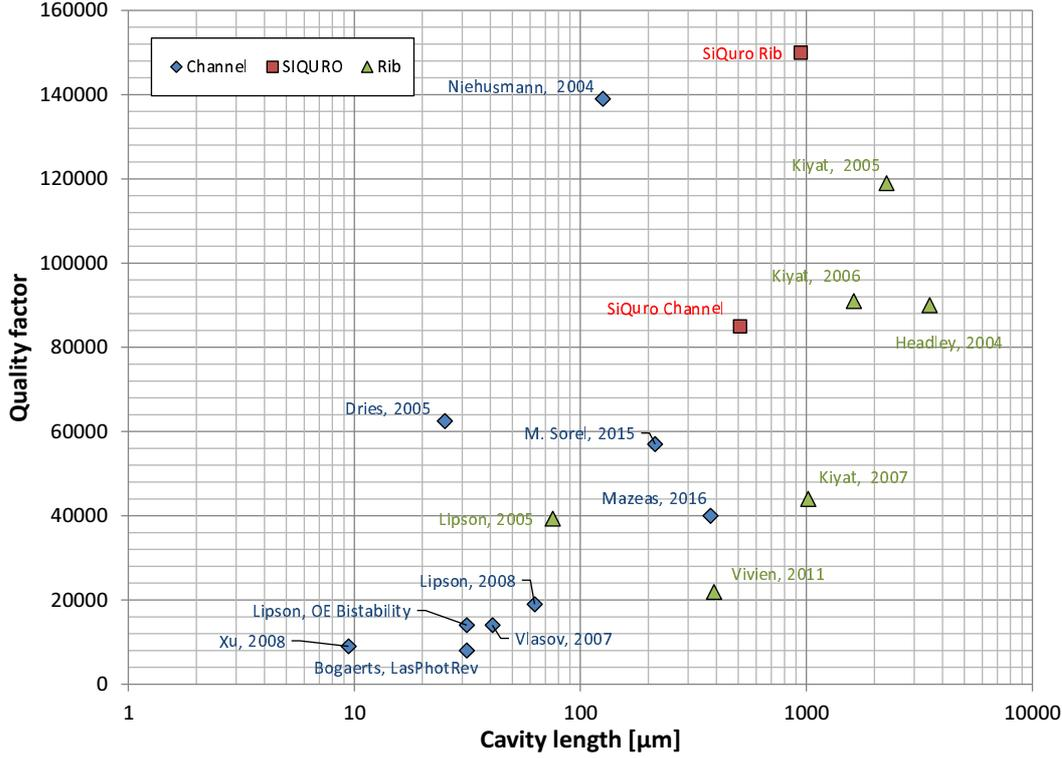
**Figure 1.26:** State of the art of the Q-factors for similar integrated devices as a function of the cavity length. The graph shows both (blue diamonds) channel and (green triangles) rib structures. The structures I developed during project SiQuro (red dots) fit in the frame.
