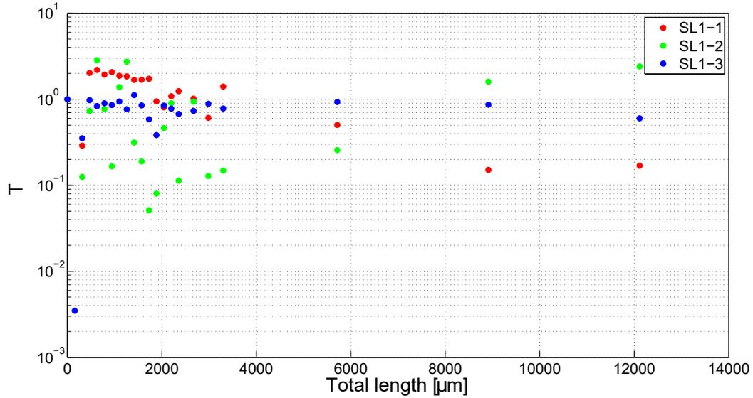
**Figure 2.22:** Transmission measurements on the S-bend waveguide structures in the NIR region. Due to mode hopping in the laser source the data is scattered, even reaching unphysical results of  $T > 1$ .
