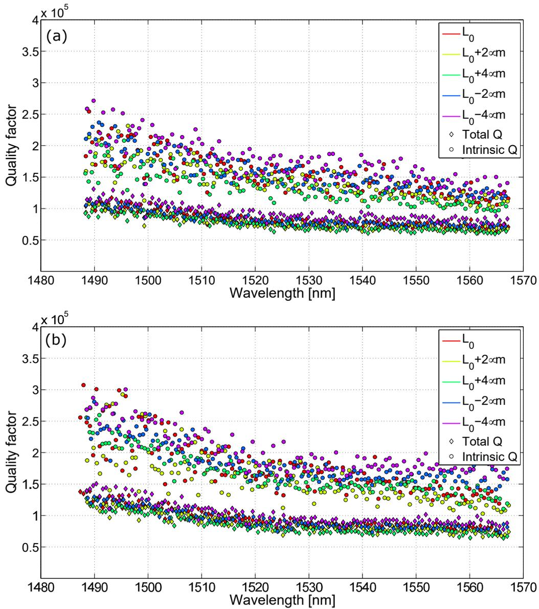
**Figure 2.26:** Quality factor estimations obtained by fitting the resonances of annealed (a) TEOS and (b) PECVD samples. The measure refers to series of five racetrack resonators with  $l_w = 2400 \text{ nm}$ ,  $R = 350 \mu\text{m}$  and  $2\mu\text{m}$  step variations around the designed critical coupling length designed for IR.
