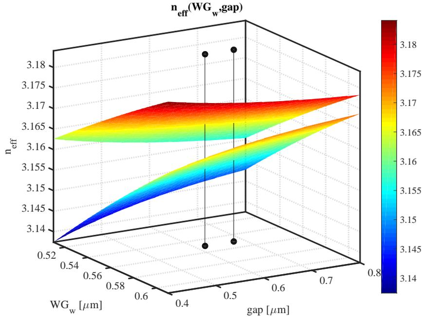
**Figure 1.28:** Effective refractive indices of the symmetric and anti-symmetric supermodes as a function of  $wg_w$  and  $gap$  for the designed directional coupler.
