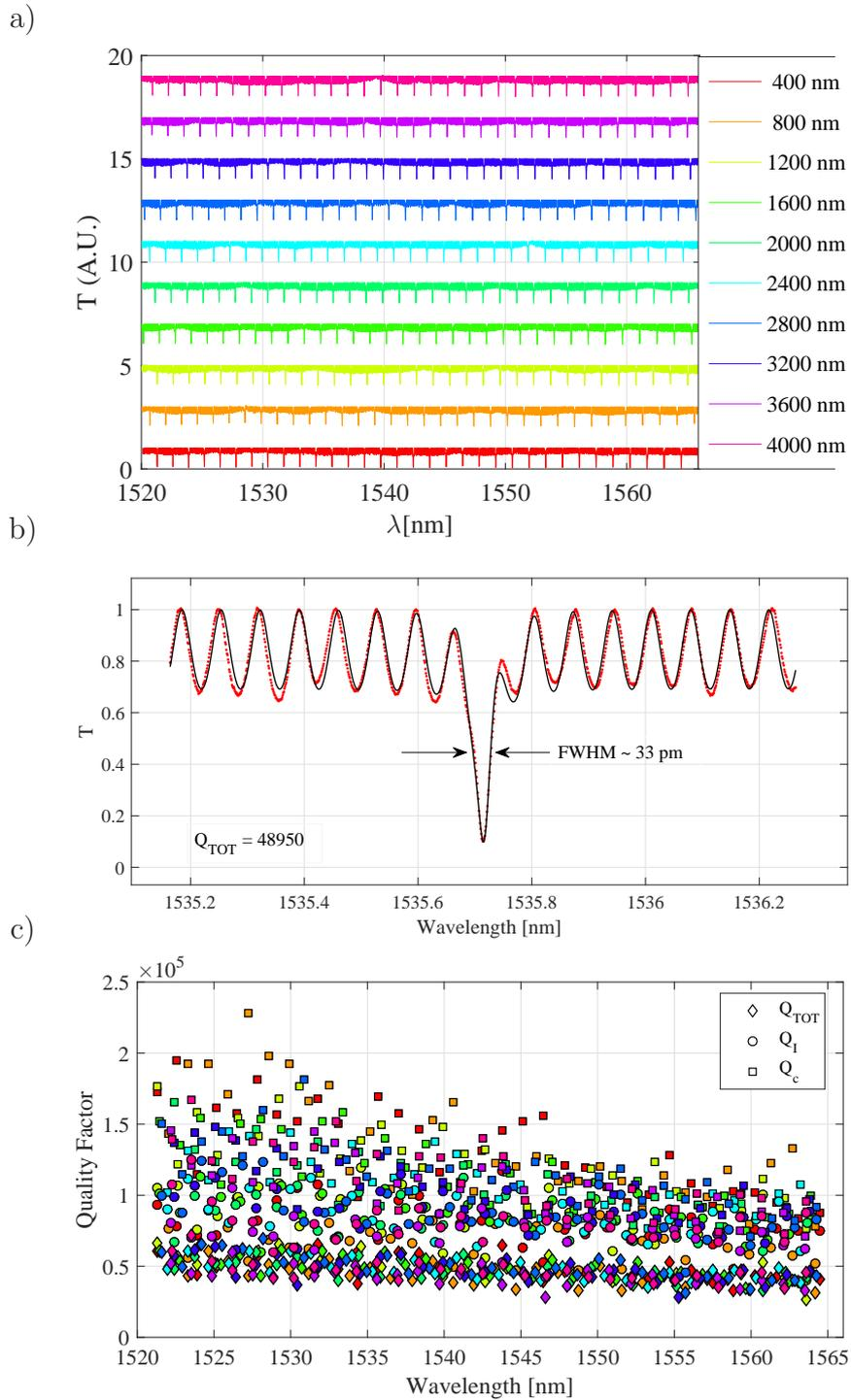
**Figure 4.10:** a) Normalized transmission spectra of ten resonators, with varying arm width. Using the routine that I developed during this thesis, the spectra are normalized on the baseline and the resonances are identified. b) each resonance is then fitted to accurately measure the Q-factor and the central position. c) the Q-factors of each resonance are reported using the same color convention as in a).
