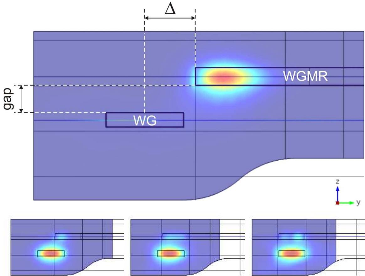
**Figure 3.3:** Simulation of the waveguide-resonator coupling using a full 3D model. (top) the waveguide is separated from the resonator through two parameters: the vertical gap and the horizontal shift  $\Delta$ . (bottom panels) The relative coupling between the first and the second RMF changes as the waveguide is pushed further under the resonator, with an increasing fraction being coupled to the  $R_2$  RMF.
