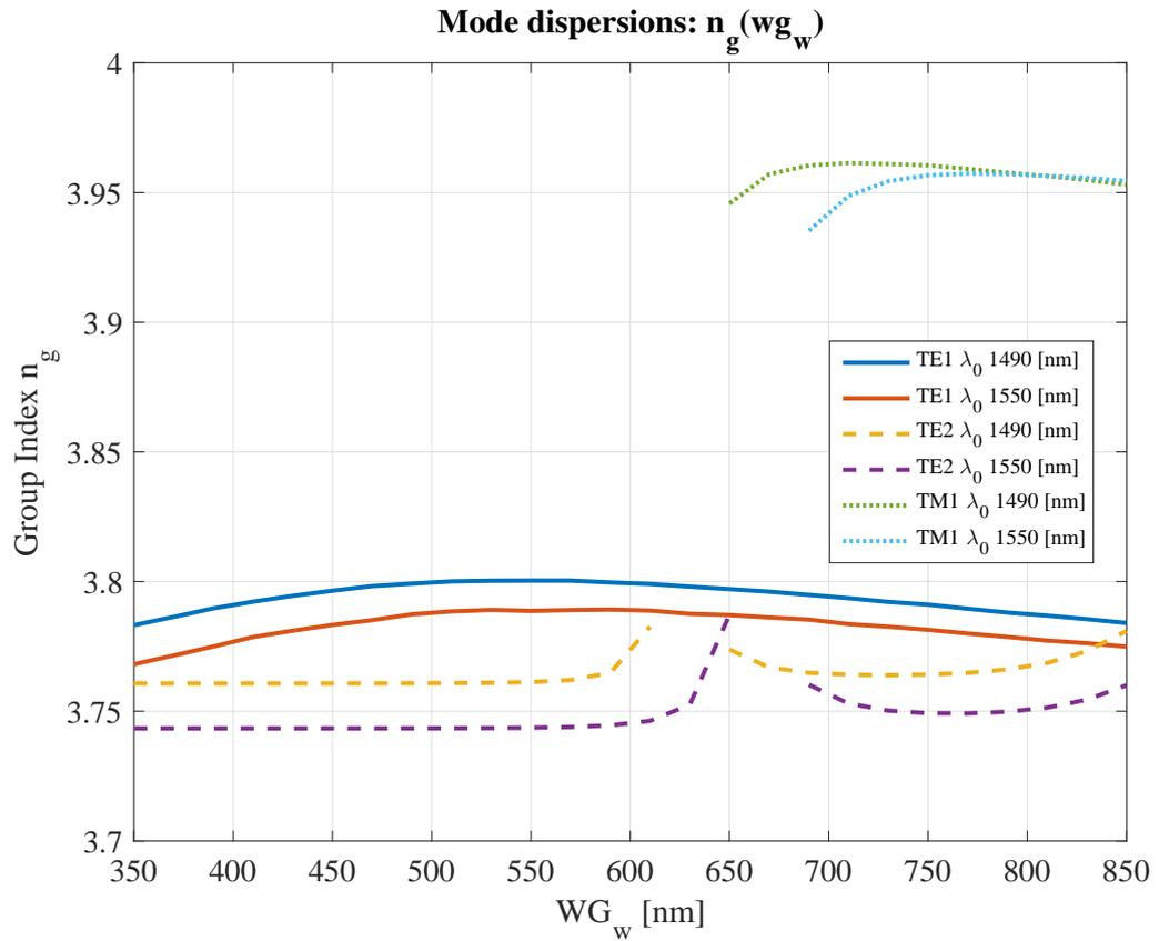
**Figure 1.8:** Group index dispersions  $n_g$  calculated from the simulated  $n_{\text{eff}}$  show that the TE1 mode has a flat region (with respect to the  $wg_w$ ) slightly around 550nm, making this value robust against fabrication tolerances. Here the mode crossing among the TE2 and TM1 mode is visible as two bumps in the group index
