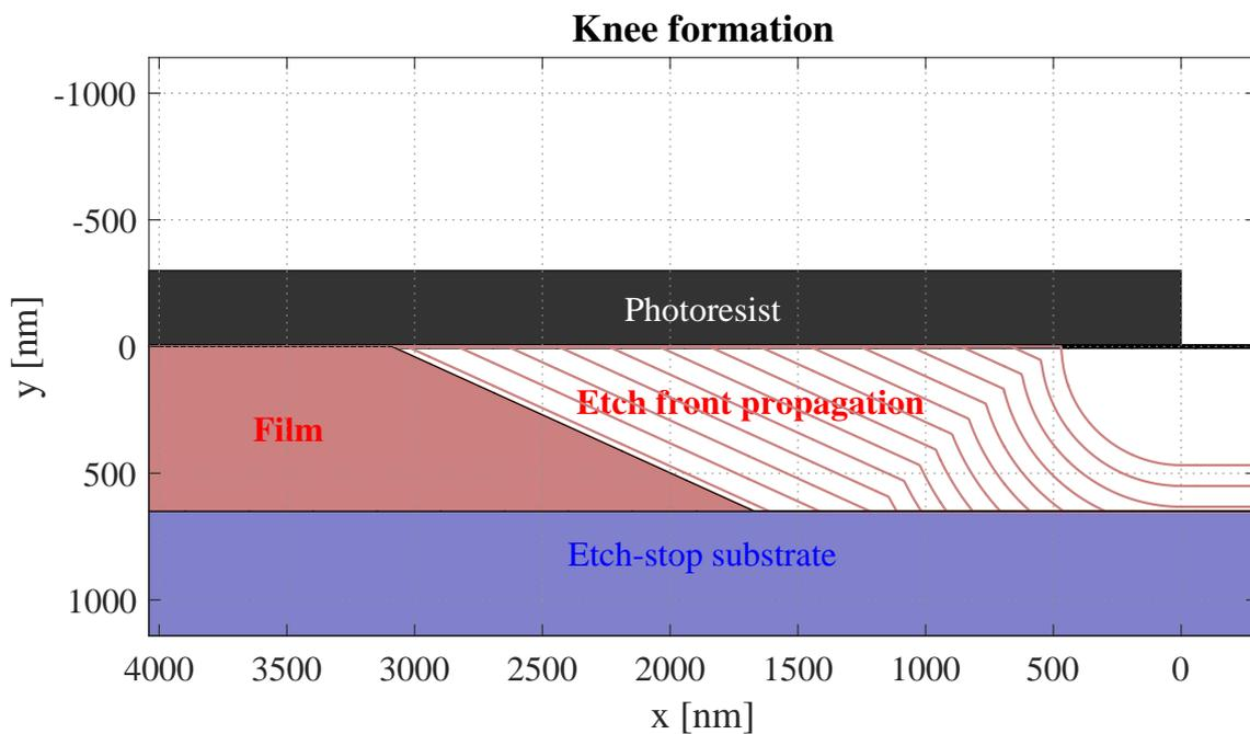
**Figure 5.4:** Formation of knees during the etching. The initial conditions are the same as in Fig. 5.1. At time  $t = t_0$  the photoresist commences detaching and a series of circular etching fronts propagates under the photoresist etch, generating angled fronts similar to Fig. 5.3. The retarded photoresist detachment produces a knee that propagates during the etching following Eq. 5.3. In this case, over-etching is advisable to get rid of the knee.
