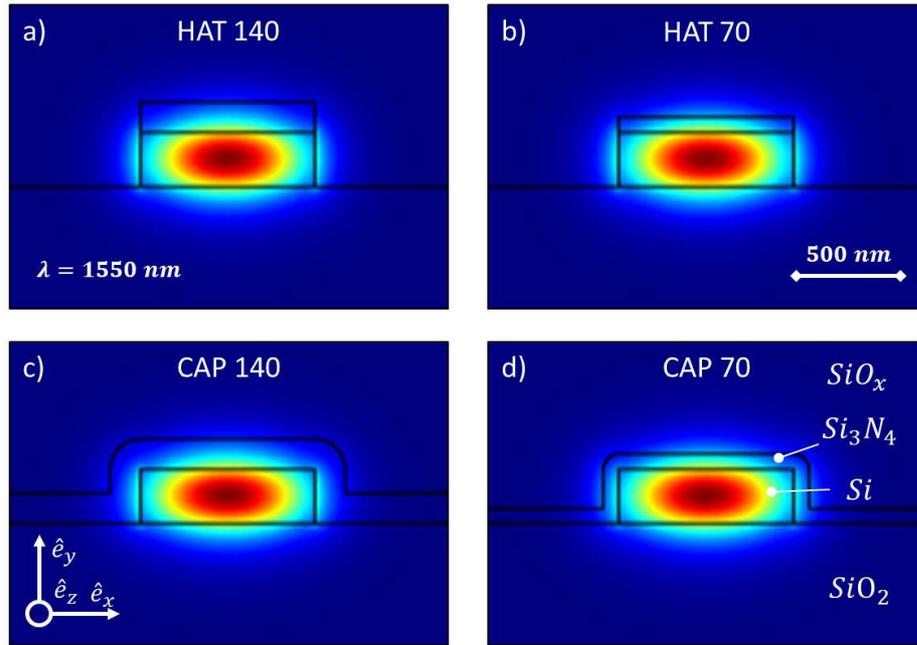
**Figure 4.5:** Color-map of the TE1 mode field distribution in the four stressing-layer configurations. Red color represents higher intensity. The waveguides were realized using two deposition schemes: conformal (c-d, CAP) and non-conformal (a-b, HAT). Both configurations have been realized with two layer thicknesses of 70 nm (b,d) and 140 nm (a,c).
