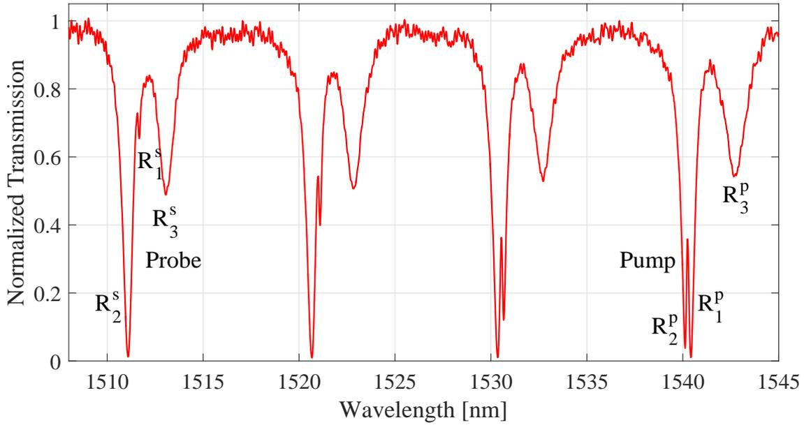
**Figure 3.12:** Cold cavity transmission spectrum of the peak-suppression pump and probe experiment, showing the whole spectral range between the pump and the probe. In this experiment, the pumped doublet is near 1540 nm, while the probe doublet at 1511 nm.
