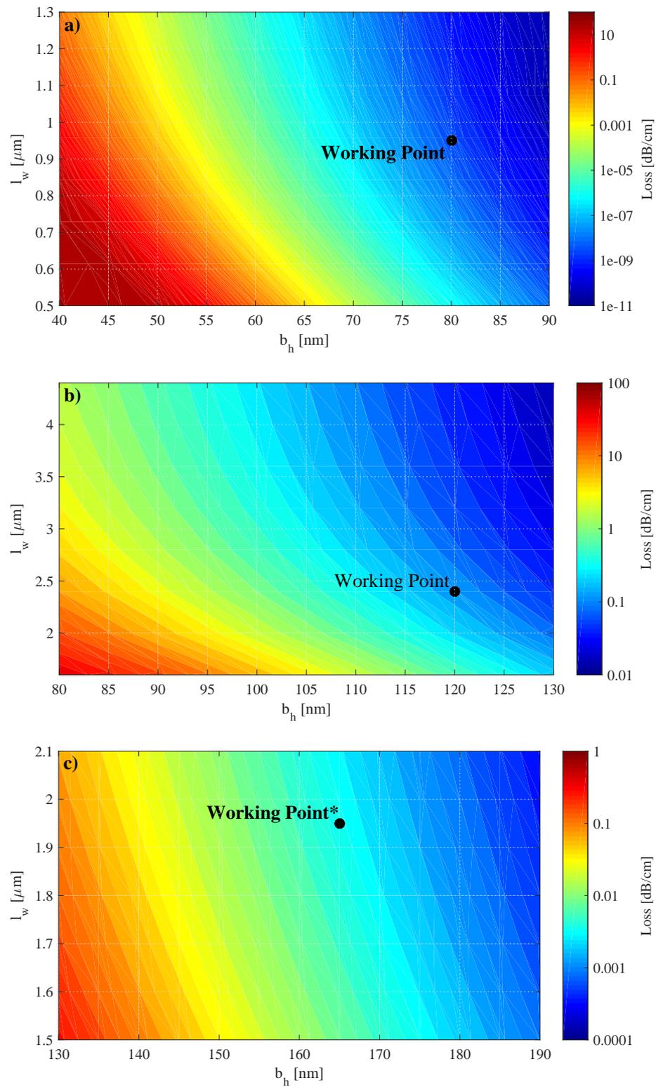
**Figure 2.13:** Simulated substrate leakage losses due to the finite bottom cladding for the a) NIR, b) IR and c) IR\* configurations. The losses, in units of dB/cm, are represented in logarithmic scale.
