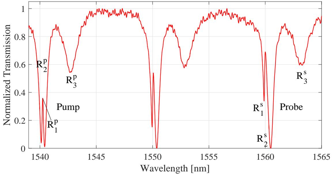
**Figure 3.14:** Cold cavity transmission spectrum of the peaks-crossing pump and probe experiment, showing the whole spectral range between the pump and the probe. In this experiment, the pumped doublet is near 1540 nm, while the probe doublet at 1560 nm.
