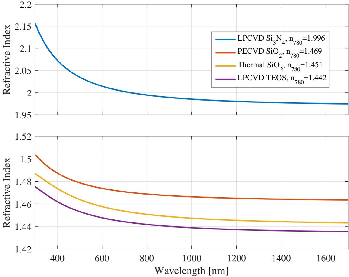
**Figure 2.5:** Bulk refractive index dispersion for the materials used for the bottom cladding (Thermal oxide), the guiding slab (LPCVD Si<sub>3</sub>N<sub>4</sub>), and loading rib (TEOS / PECVD SiO<sub>x</sub>).
