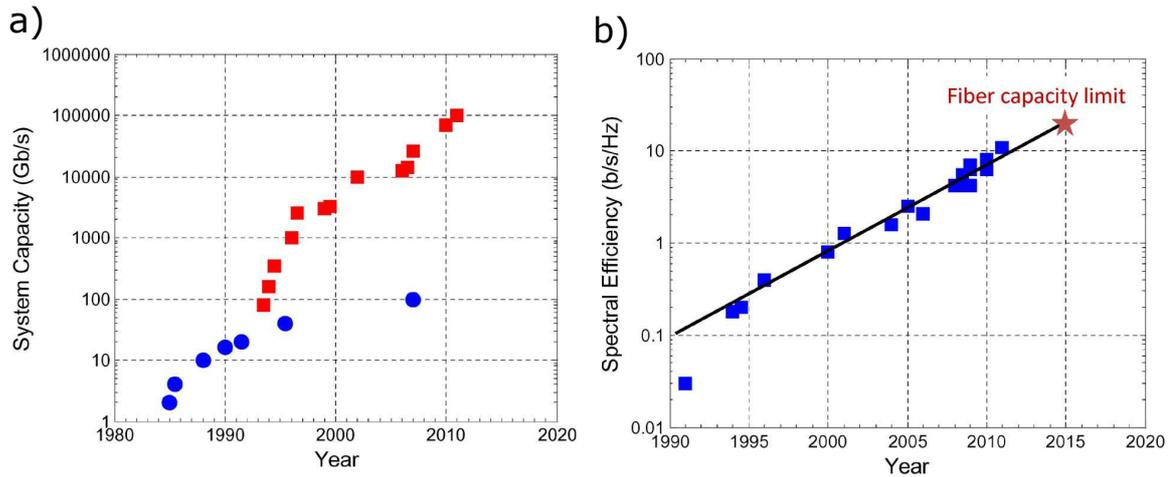
**Figure 2:** a) fiber system capacity during the years. The blue circles represent single-mode fibers for Time Division Multiplexing, while the red rectangles represent fibers engineered for Wavelength Division Multiplexing applications. b) evolution of the spectral efficiency of single fibers developed during the years. The red star corresponds to the maximum achievable spectral efficiency according to Shannon’s limit, set by the non-linear effects in optical fibers. Images from [3]
