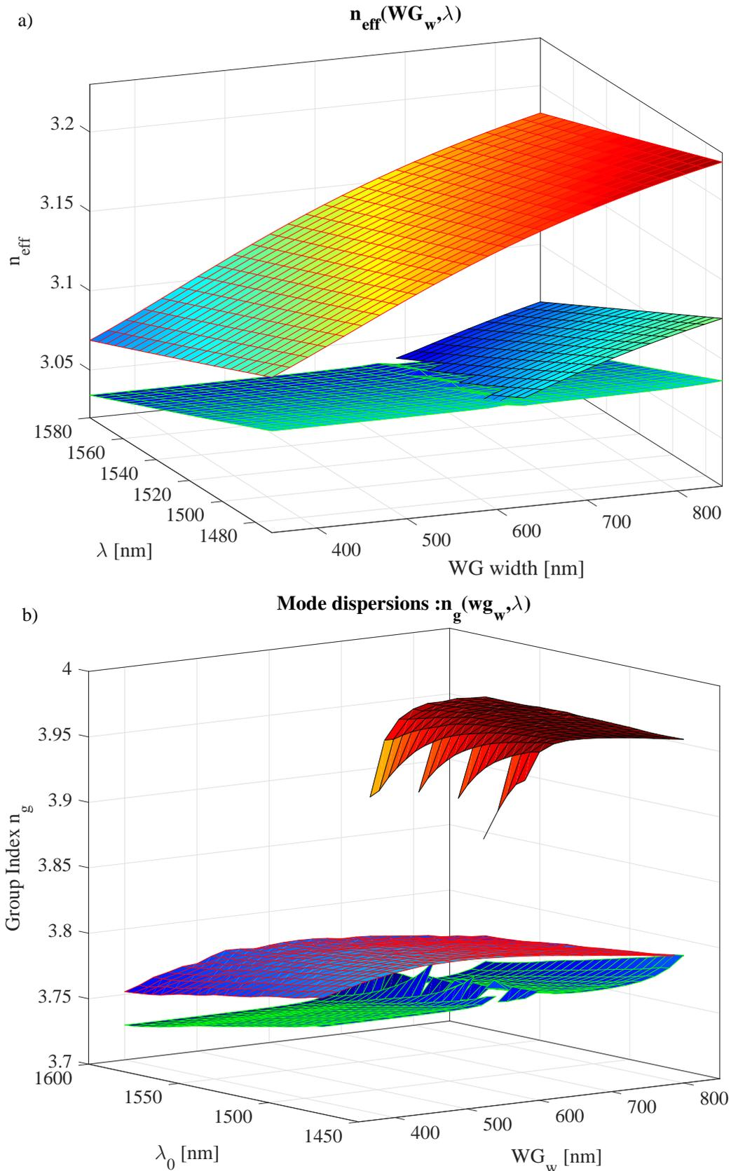
**Figure 1.5:** 3D plot of the a)  $n_{\text{eff}}$  and b)  $n_g$  dispersions as a function of waveguide width and wavelength, summarizing the results of the simulations. The surface color is proportional to the dispersion, while the grid colors red, black and green are for TE1, TM1 and TE2 modes respectively. The missing points on the TE2  $n_g$  surface were affected from a computational artifact due to the TM1 crossing and removed to avoid confusion.
