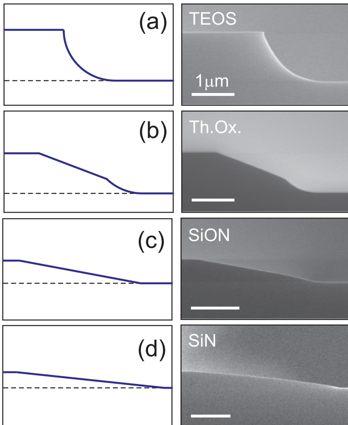
**Figure 5.5:** Selected SEM images of the etched profiles of various materials with the corresponding theoretical profiles for (a) TEOS, (b) Thermal Oxide, (c) PECVD silicon oxynitride and (d) PECVD silicon nitride.
