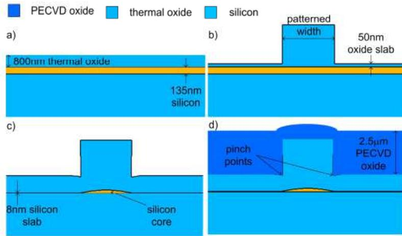
**Figure 1.9:** Waveguide definition through silicon oxidization results in an exceptionally smooth surface at the cost of a poor control over the waveguide shape. Image taken from [58].
