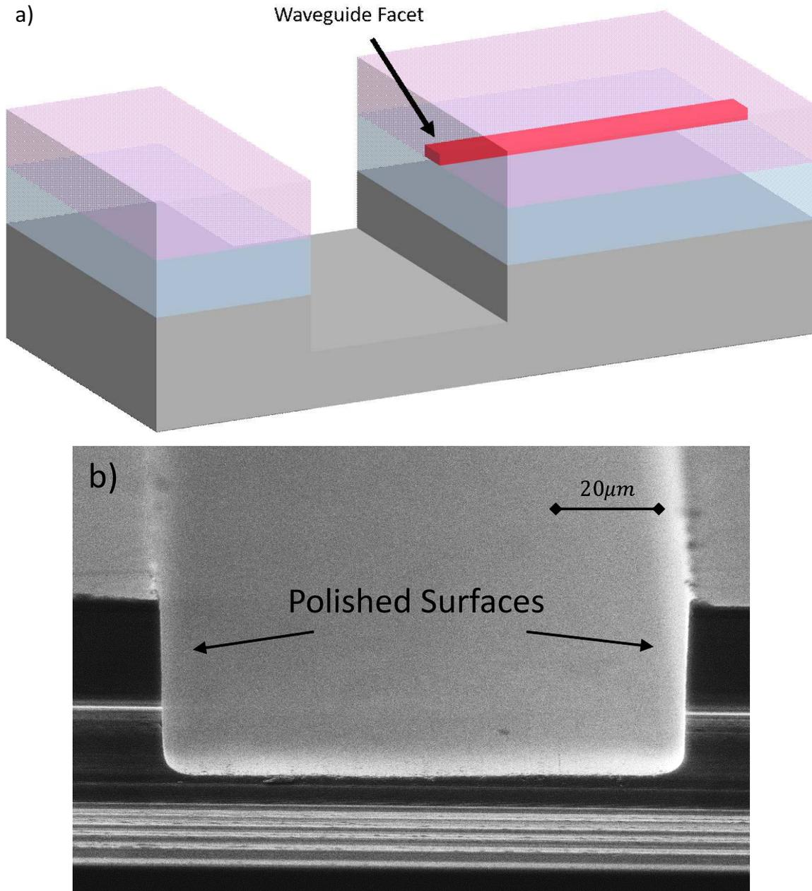
**Figure 1.15:** a) facet definition during the dicing process is achieved with a polishing-millstone-saw that abrades a 100 nm deep groove in the wafer, while polishing the sidewalls where the waveguide is present at the same time (image is not in scale). Proper dicing through the whole substrate is realized in a second step, with a thinner millstone that does not touch the polished walls. b) SEM image of a test groove before complete dicing.
