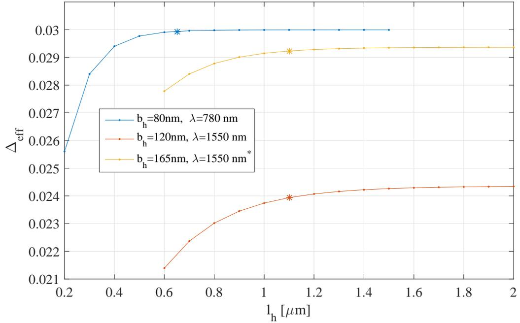
**Figure 2.11:** (blue) NIR, (orange) IR and (yellow) IR\*  $\Delta_{\text{eff}}(l_h)$  curves for the designed working points.
