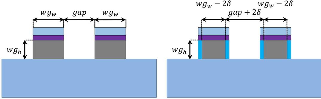
**Figure 1.29:** Waveguides in a DC(left) prior and (right) after a smoothing cycle. Each RCA cycle of the smoothing process consumes  $\delta = 5$  nm of silicon. The waveguides are therefore reduced by an amount  $2\delta$  and the gap in the DCs is increased accordingly. The image is not in scale.
