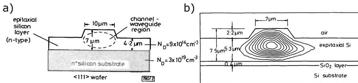
**Figure 6:** a) a silicon on doped silicon single-crystal waveguide used in Soref's experiments of 1985. The original paper, from which the image is taken, is [22].
