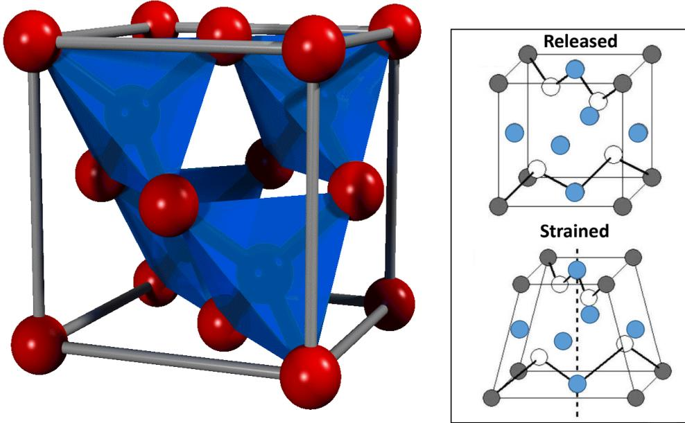
**Figure 4.2:** a) Face Centered Cubic crystalline structure of silicon. The orange tetrahedra highlight the symmetric environment in which each atom is immersed. b) by applying an inhomogeneous strain on the lattice it is possible to break the inversion symmetry.
