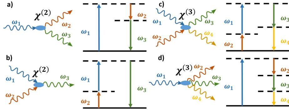
**Figure 4.1:** Feynman diagrams and virtual-level representations of some multi-photon processes. a) Spontaneous Parametric Down Conversion (SPDC) and b) Sum Frequency Generation (SFG) are  $\chi^{(2)}$  processes while c) and d) represent Four Wave Mixing (FWM) through  $\chi^{(3)}$  optical non-linearity.
