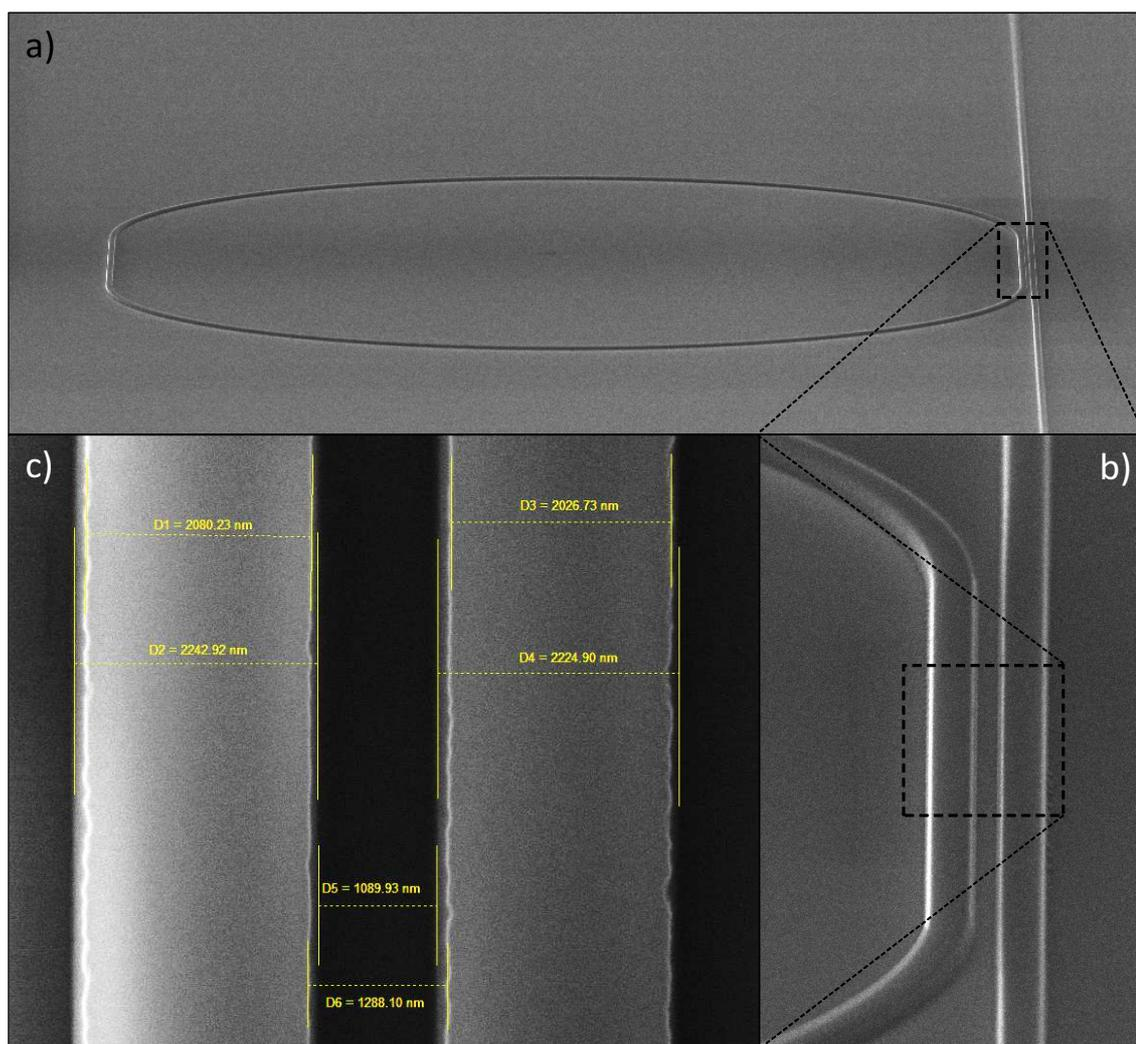
**Figure 2.16:** SEM images of the samples during the fabrication permitted to measure the actual dimensions of the structures. a) Fish-eye image of a strip-loaded racetrack resonator. The b) coupling region dimensions are crucial to obtain critically-coupled resonances, and are therefore c) verified through SEM imaging.
