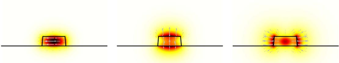
**Figure 9:** Cross sectional view of TE1, TM1 and TE2 modes in a Si channel waveguide. The color is darker where the field is stronger. The gray arrows represent the direction of the electric field.
