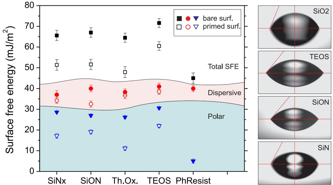
**Figure 5.8:** (left) Measured values of the total SFE and its dispersive and polar components for the different films and the photoresist. In the case of dielectric materials the measurements were performed both for bare and primed surfaces. (right) Examples of photographs of BHF droplets on dielectric films. Image from [178].
