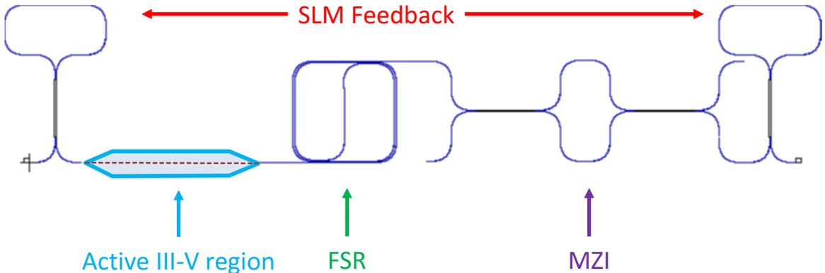
**Figure 1.1:** Schematic of the laser, under kind permission of III-V labs. The resonant cavity is created by two Sagnac Loop Mirrors (SLM) (red). The active region (cyan), vertically coupled to the underneath silicon waveguide, provides emission and amplification. The allowed bandwidth, tailored by a Mach-Zehnder interferometer, is shaped into a comb of peaks through the FP cavity. The optical path (green) determines the Free Spectral Range.
