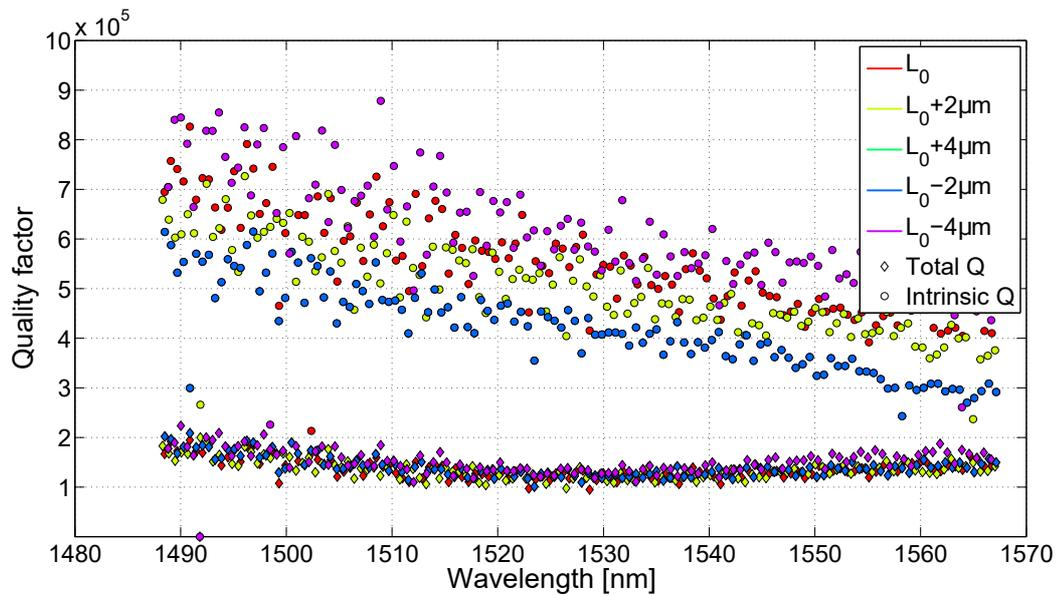
**Figure 2.28:** Q-factor estimations from the fit of the transmission measurement of large structures ( $l_w = 2.8 \mu\text{m}$ ) on a PECVD sample that was not annealed. The Q-factors of these structures exhibit the highest values in the IR range.
