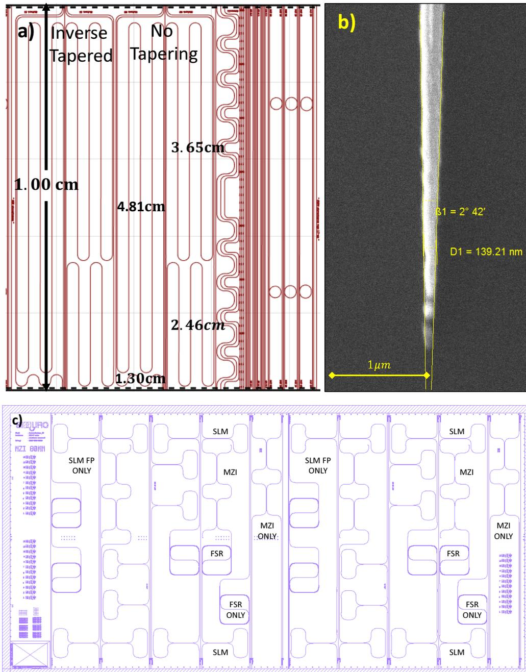
**Figure 1.20:** a) test layout of the WP1\_L1 process. (left) folded waveguides of different length are present in both inverse-tapered and straight termination configurations. Among the other test structures, All-Pass racetrack ring resonators with different coupling length are present on the layout.
