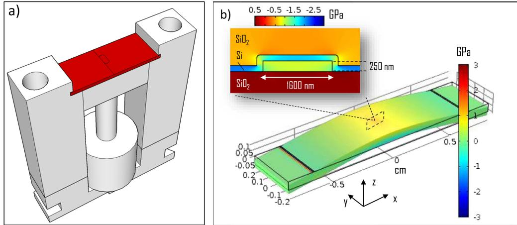
**Figure 4.13:** a) 3D model of the stressing sample holder. While two small indentations keep the sample borders in place, the cylinder in the middle acts on a screw that pushes against the center of the sample (red) stressing the resonator, sketched above the sample. b) FEM simulations of the stress distribution directed along the  $x$  direction inside the sample for a CAP waveguide near the half-course of the screw.
