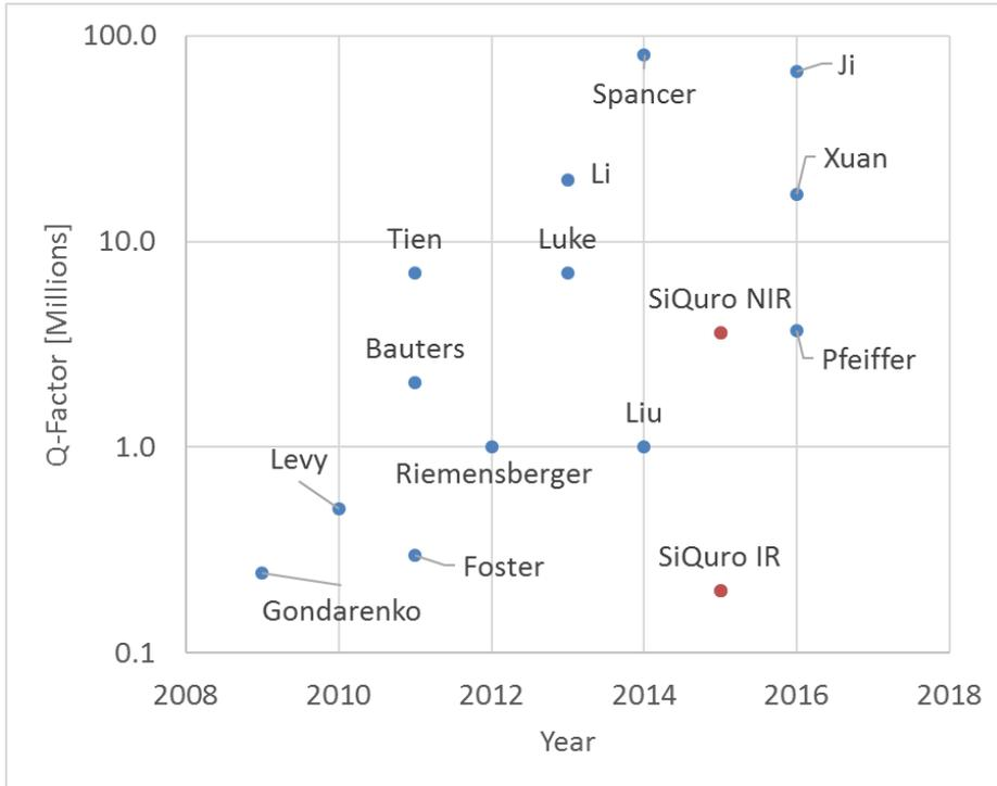
**Figure 2.29:** Quality factors of  $\text{Si}_3\text{N}_4$  micro-resonators found in literature. The cited works are reported in Tab. 6.
