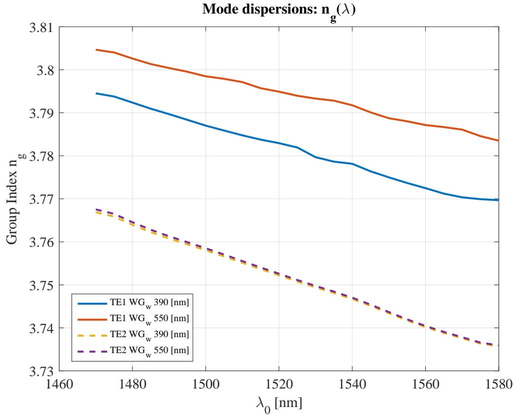
**Figure 1.6:** Modal dispersions a)  $n_{\text{eff}}$  and b)  $n_g$  as a function of wavelength in the range 1460nm-1580nm for sample widths of 390nm and 550nm. The dispersion of the TE1 mode for the two rib widths coincide, demonstrating that the mode is not confined in the rib and is therefore unaffected by its width. The TM1 are similarly not guided and omitted. The simulations give a value for  $n_g$  of 3.8 at 1490 nm for the waveguide width value of 550 nm.
