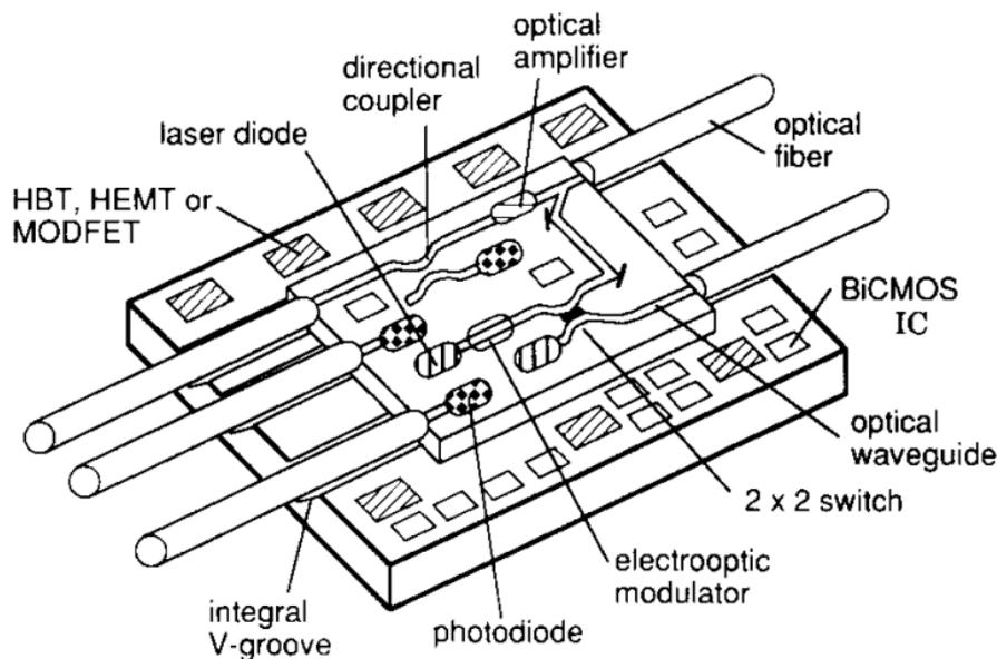
**Figure 7:** Soref's Opto Electronic Integrated Circuit (OEIC) "superchip" visionary idea, from [27].
