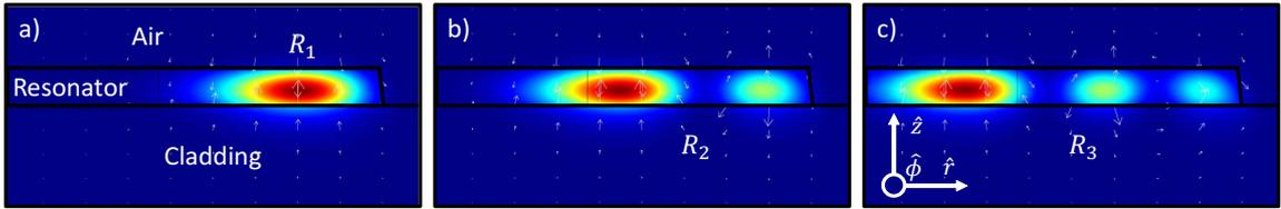
**Figure 3.1:** a) first, b) second and c) third radial modes electric field intensity distribution in an integrated microresonator. Red color corresponds to high value of field intensity, while deep blue corresponds to zero field. The white arrows represent the local direction of the electric field.
