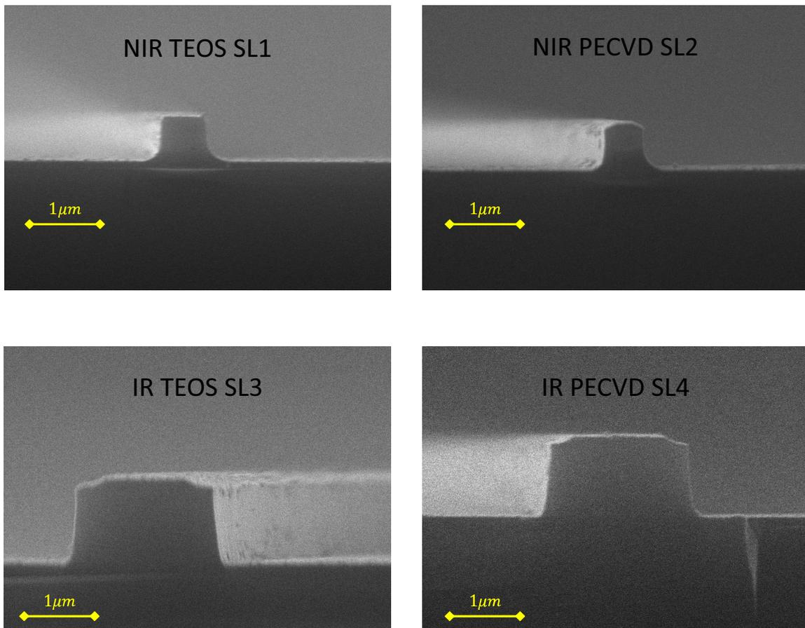
**Figure 2.17:** SEM images waveguides facets from the different realizations. In all samples the round foot at the base of the strip due to the wet-etching of the final 100 nm is visible. The waveguides are covered with a thin gold layer to avoid the accumulation of charges during SEM imaging, which is responsible for the visible roughness.
