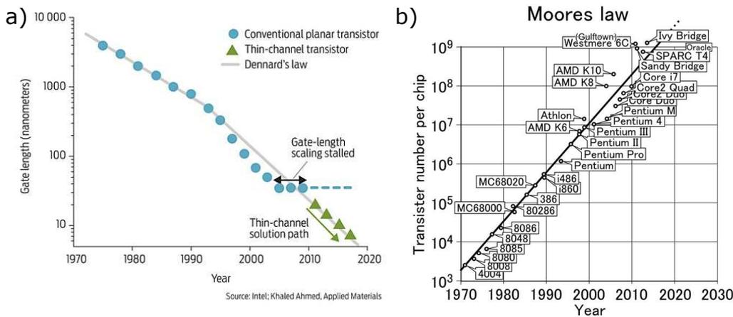
**Figure 4:** Evolution of the a) gate-length [12] and b) number of transistors per chip (from:[13]). The integration density of the processors realized in the past fifty years is in good agreement with the 1965 Moore’s law prediction.
