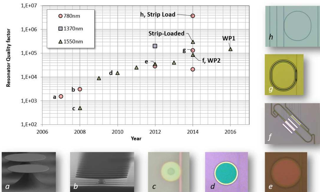
**Figure 11:** Resonators in various configurations realized at FBK and their Q-factor.
