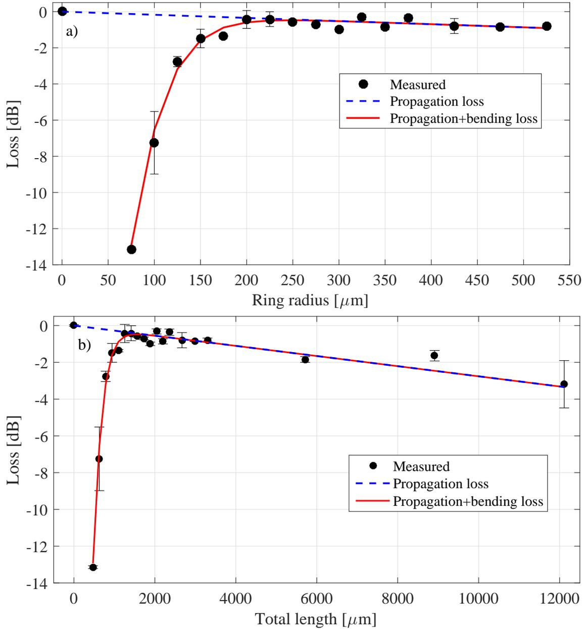
**Figure 2.21:** Transmission measurement of the S-bend waveguides samples for the PECVD oxide samples in the IR region reported as a function of (top) curvature radius and (bottom) total waveguide length. The errorbars on the data represent the standard deviation over three samples. The red line represents the fit of the data using Eqs. 1.5 and 2.6. The result of the fit is reported in Tab. 2.4.
