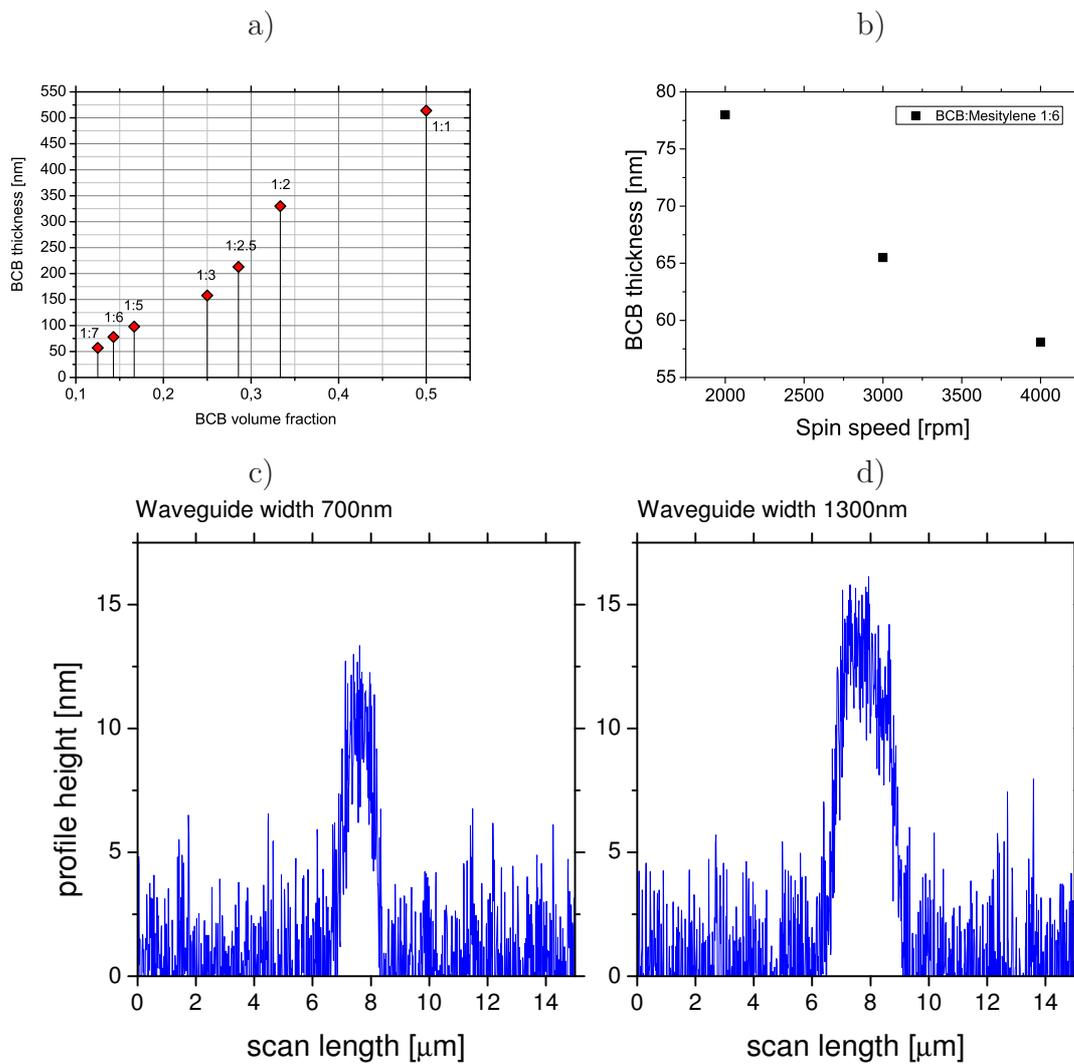
**Figure 1.33:** BCB thickness as a function of a) the dilution in mesitylene and b) the spinning speed. b,c) profile height measurements of the BCB above the waveguides demonstrates the achieved degree of planarization.
