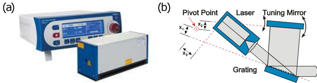
**Figure 2.19:** Sacher Lasertechnik LiON TEC-500 NIR laser source with external cavity. The cavity is controlled via a motor for long wavelength scans and via a piezoelectric actuator for accurate analysis in a small wavelength region.
