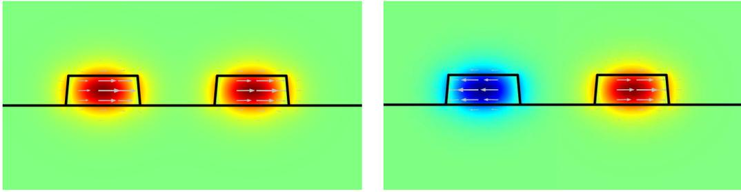
**Figure 10:** Symmetric and anti-symmetric supermodes of two coupled waveguides. The color represents the intensity of the  $E_x$  field component, which is the dominant. The gray arrows are samples of  $E$ , showing that  $E_x$  is the dominant component, that is opposite in the two waveguides for the asymmetric mode.
