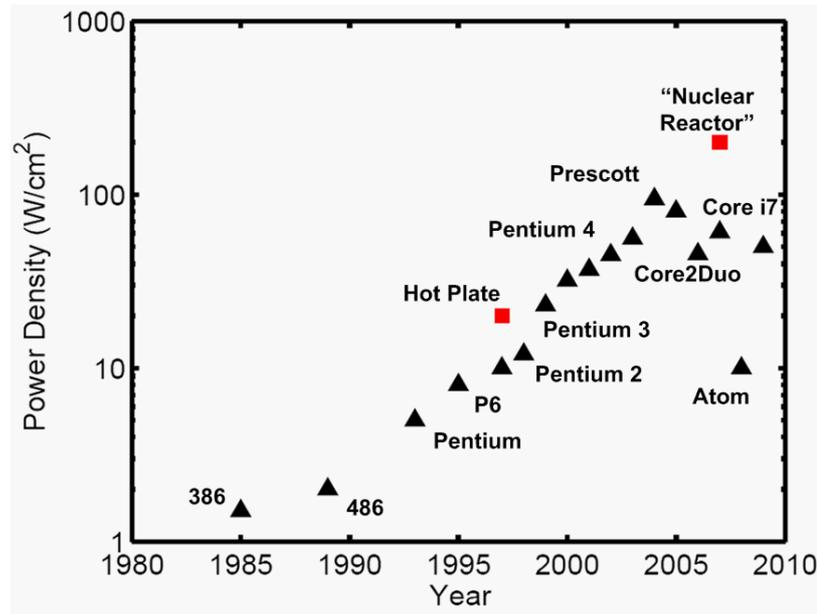
**Figure 5:** Time evolution of the power density in popular CPUs, compared to the same quantity in a hot plate and a nuclear reactor. Image from [18].
