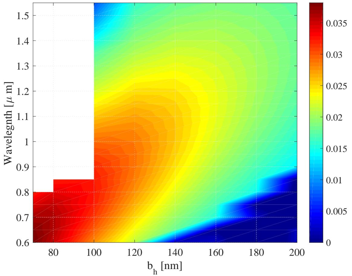
**Figure 2.3:** Effective index contrast  $\Delta_{\text{eff}}$  between the slab-guided and the strip-loaded guided modes as a function of the slab thickness  $b_h$  and the probe wavelength obtained from 2D FEM simulations.
