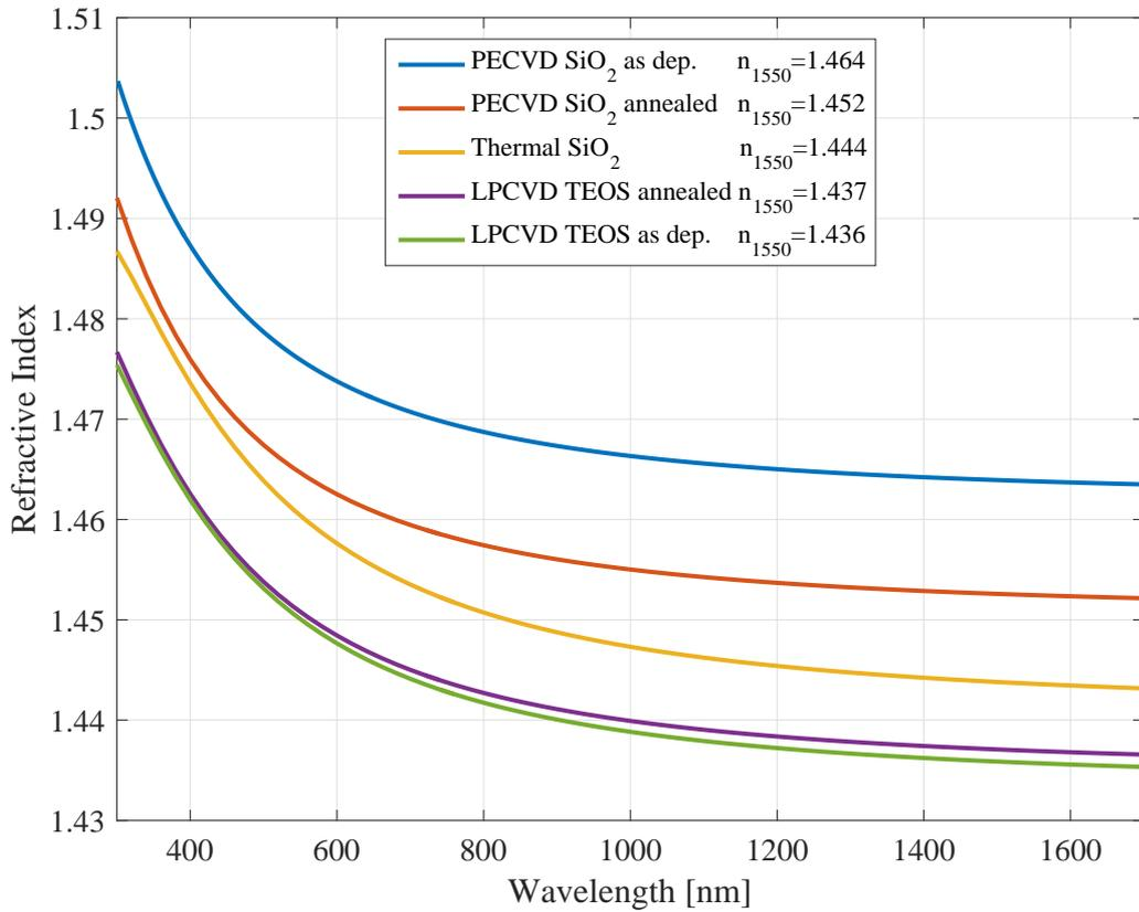
**Figure 2.27:** TEOS and PECVD oxide index dispersions before and after annealing, compared to that of thermally grown oxide.
