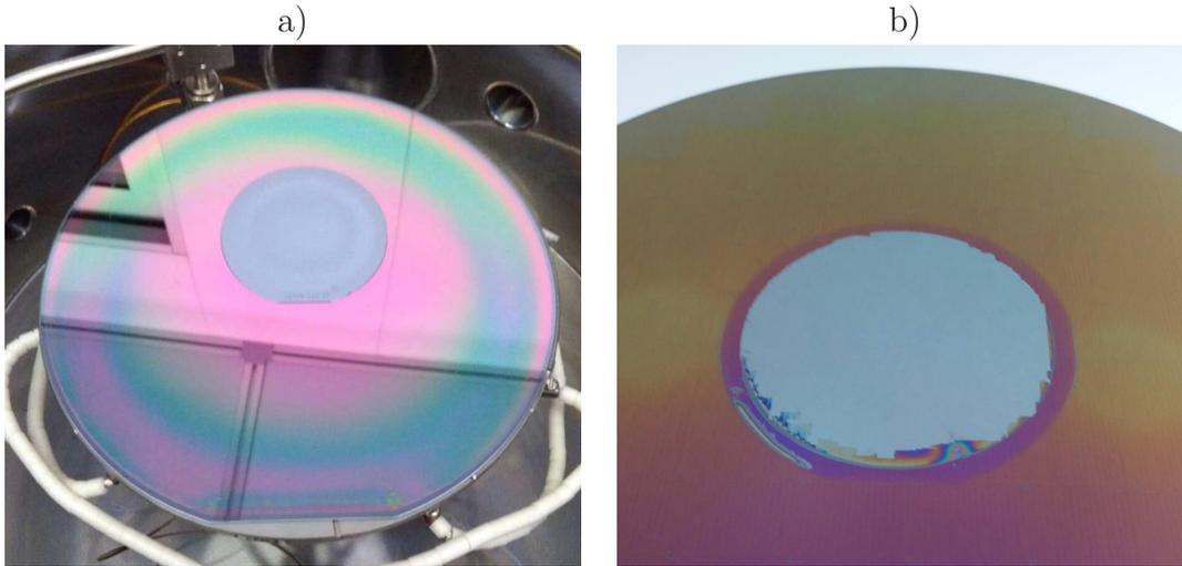
**Figure 1.35:** a) III-V wafer bonded on Si. b) III-V layer after the substrate removal. A small portion of the borders resulted ill-bonded and detached during the substrate etching. Over all, > 80% of the MQW surface remained after the substrate removal, although deformations of the layer are present on the edges, as shown in Fig.1.36.
