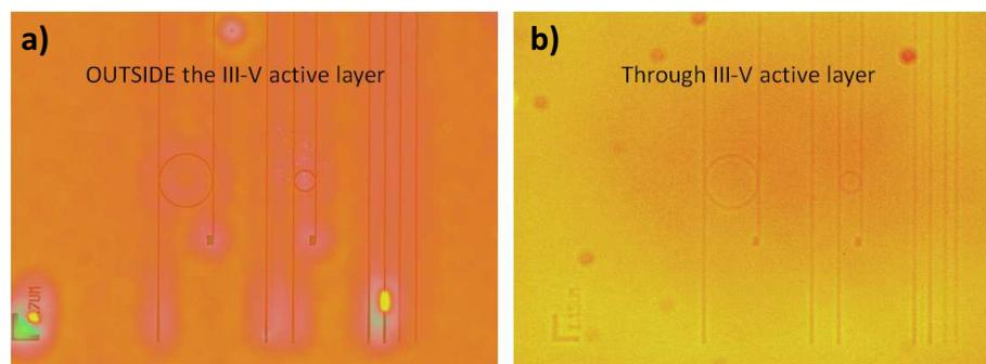
**Figure 1.37:** Optical images of the SOI PIC a) under the BCB layer and b) through the III-V active layer.
