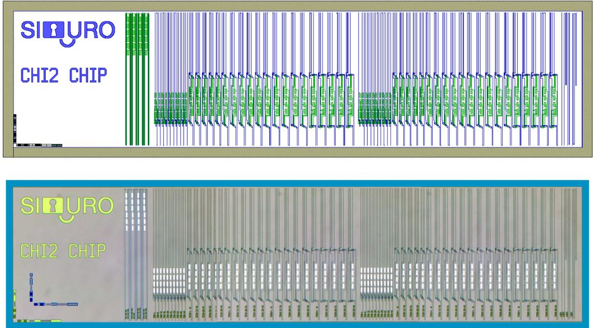
**Figure 4.7:** (top) image of the layout, compared to (bottom) a composed-optical image of the realized device. In the layout, the silicon device layer is represented in red, while in the optical image is yellowish. In green(gray) the aluminum pads realized for the contact-tip are well visible.
