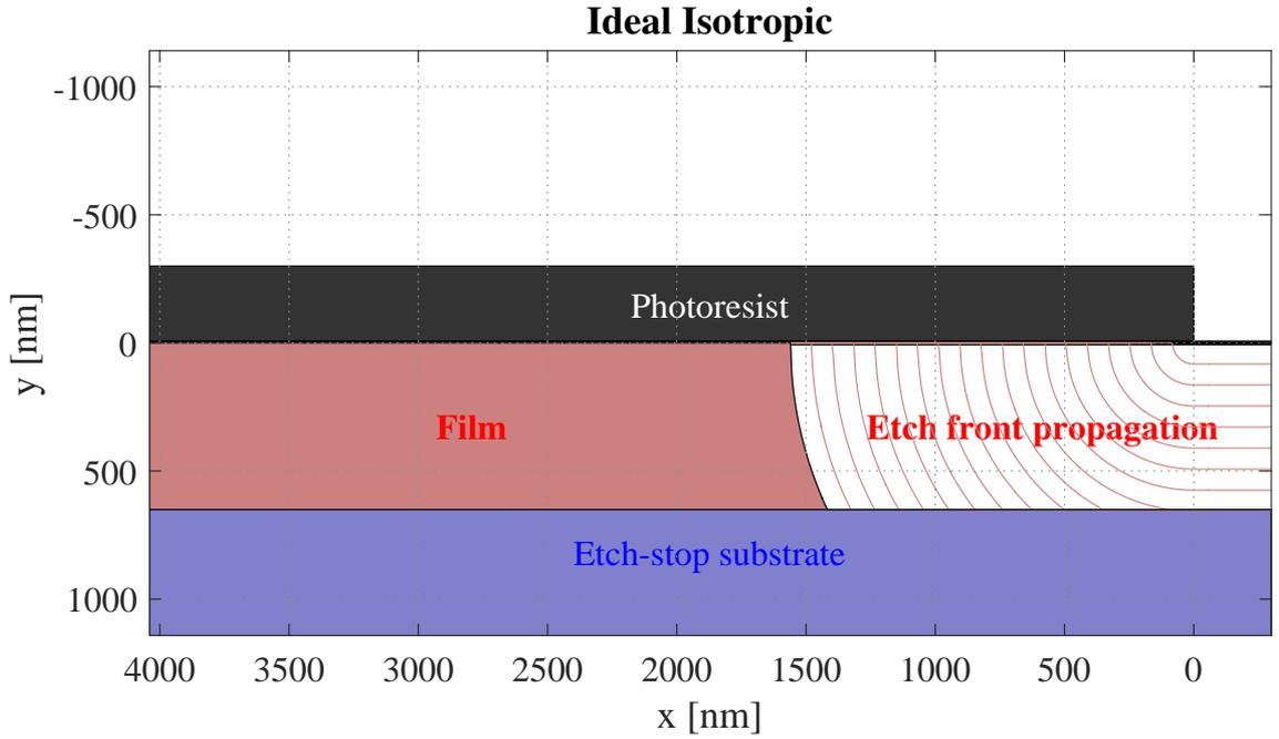
**Figure 5.1:** Isotropic etching profiles. The etched material (solid red) is covered by (solid black) patterned photoresist. When the etching begins, a circular etching front (red lines) propagates under the photoresist etch, while a flat front is created in the unprotected region. If the etching continues after reaching the (solid blue) etch-stop underneath material under the unprotected region, the circular front continues to expand between the photoresist and the etch-stopping material.
