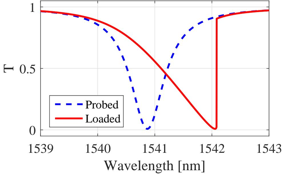
**Figure 3.10:** Resonant lineshape modification under a sweeping pump in the presence of optical non-linearity. The cold cavity spectrum (dashed line) is obtained with a weak probe. When sweeping the spectrum using a high power laser (solid line), the resonance shifts progressively due to the increasing non-linear effect, resulting in a spectrum with an apparent discontinuity, where the cavity mode de-locks from the pump laser.
