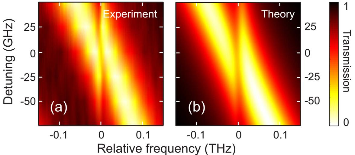
**Figure 3.8:** Color-map (a) of the doublets spectra against the detuning  $\delta$ . In the image is realized by interpolation of six spectra taken at different azimuthal number and centered around the position of the  $R_1$  peak. Color-map (b) of the analytical prediction for the same spectra.
