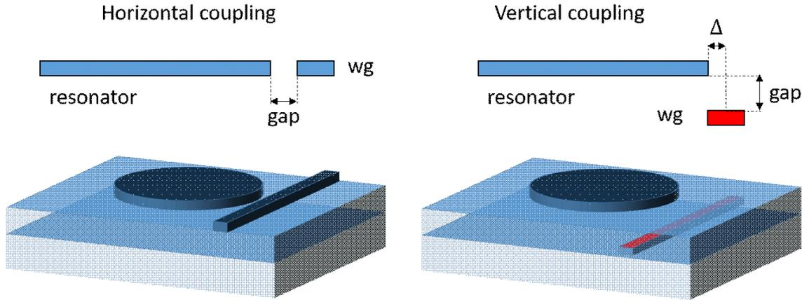
**Figure 3.2:** Typical (left) horizontal and (right) vertical coupling configurations for integrated microresonators. In the horizontal coupling the waveguide and the resonator are fabricated in the same material and the only parameter of the coupling is the gap among the two. In the vertical coupling configuration, both a vertical gap and a lateral shift,  $\Delta$ , are present.
