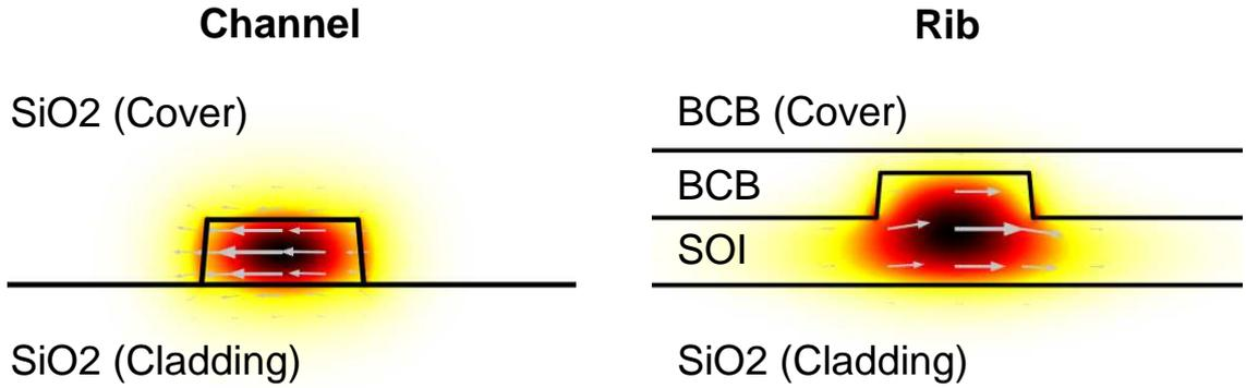
**Figure 1.2:** Normalized field intensity inside a (left) channel and a (right) rib waveguide for the fundamental TE<sub>1</sub> mode. In the channel waveguide the field is strongly confined within a small area, so that the intensity on the lateral surface of the waveguide is strong. In the rib geometry, on the other hand, the light is confined within the much larger silicon slab and only a small fraction of the field touches the shallow waveguide lateral edges.
