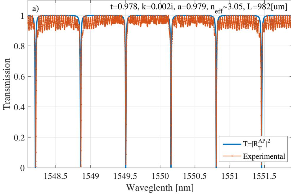
**Figure 13:** An example of All-Pass Through spectrum from the rib racetrack resonator FIGURE. The experimental points (orange) exhibit sharp quasi-critical resonances. The fast oscillating features near 1 transmission are spurious Fabry-Perot resonances due to the bus waveguide facets. The resonator parameters were then plugged in the All-Pass transfer function, leading to the transmittance (blue) which is  $|R_T^{AP}|^2$ .
