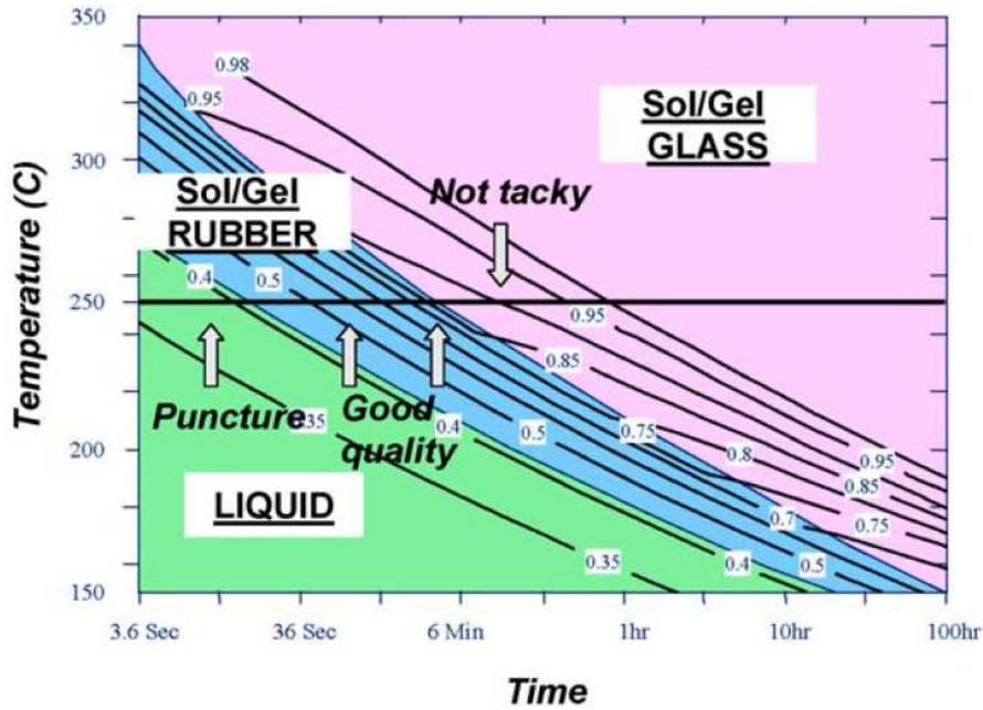
**Figure 1.38:** Time-Temperature transformation diagram of DVS-BCB. Image from [64]
