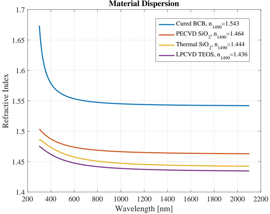
**Figure 1.4:** Bulk index dispersion of the used materials, fabricated in the FBK facility, measure with VASE.
