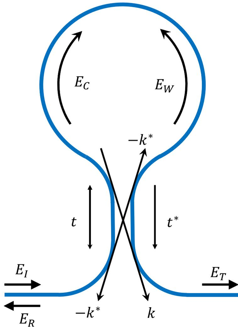
**Figure 1.27:** Coupling scheme of a Sagnac Loop Mirror. The notation used for the coupler is similar to that of Fig. 12. The input field  $E_I$  enters from the left. The couplers splits the amplitude into the clockwise and anticlockwise components  $E_c$  and  $E_w$ , which are in turn split again at the coupler. The interference between the split  $E_c$  and  $E_w$  gives rise to the transmission and reflection spectrum.
