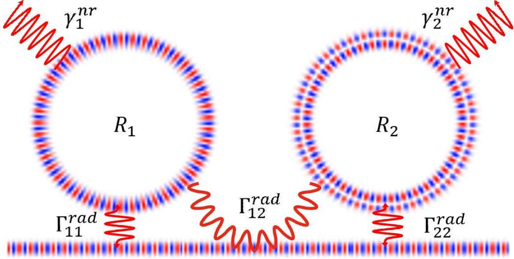
**Figure 3.5:** Representation of the various coupling terms of the resonator. Each RMF is coupled to the waveguide through the term  $\Gamma_{ii}^{\text{rad}}$  and to the environment with  $\gamma_i^{\text{nr}}$ . Furthermore,  $R_1$  and  $R_2$  are coupled together through the waveguide by the term  $\Gamma_{12}^{\text{rad}}$ . The two RMFs are actually inside the same resonator in partial spatial overlap.
