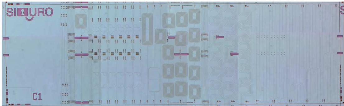
**Figure 1.12:** a) layout of the first test mask with b) an optical imaging of a realized device. The structures realized to measure the propagation losses are on the far right.
