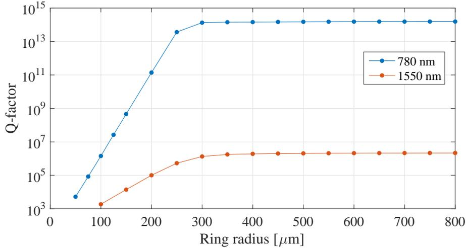
**Figure 2.14:** Simulated quality factors of SL-resonators for the (blue) NIR and (orange) IR SL-resonators as a function of the curvature radius. The resonators are simulated using an axisymmetric 2D scheme, where the losses that determine the Q-factor are simulated by a Perfect Match Layer absorber situated far from the SL structure.
