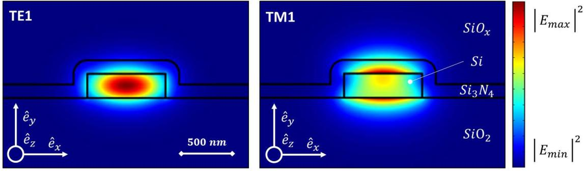
**Figure 4.3:** Simulated TE1 and TM1 modes optical field intensity inside a SOI waveguide covered by a conformal layer of  $\text{Si}_3\text{N}_4$  (CAP configuration).
