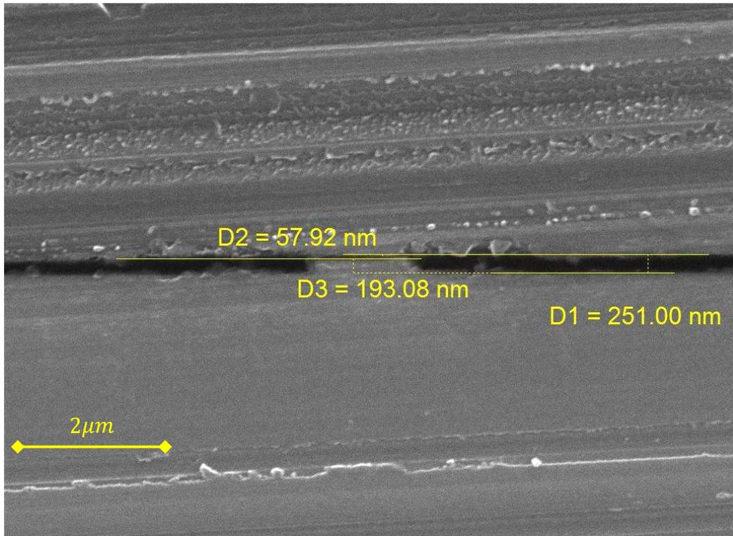
**Figure 1.34:** Cross section SEM image of a Si die bonded on a structured Si wafer. The image shows how the bonding may be realized with a residual BCB layer on top of the waveguides as thin as 60 nm.
