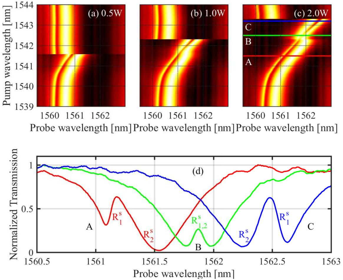
**Figure 3.15:** Pump and probe experiments demonstrating the complete crossing of the probe modes. Panels (a),(b) and (c) represent the same experiment repeated with different input power conditions of 0.5 W, 1 W and 2 W, respectively. (d) The selected cross-section spectra, under 2 W pump, demonstrate three cases of the relative detuning, which changes from positive (A) to negative (C) passing through the  $\delta\omega_0^{1,2} \approx 0$  condition (B).
