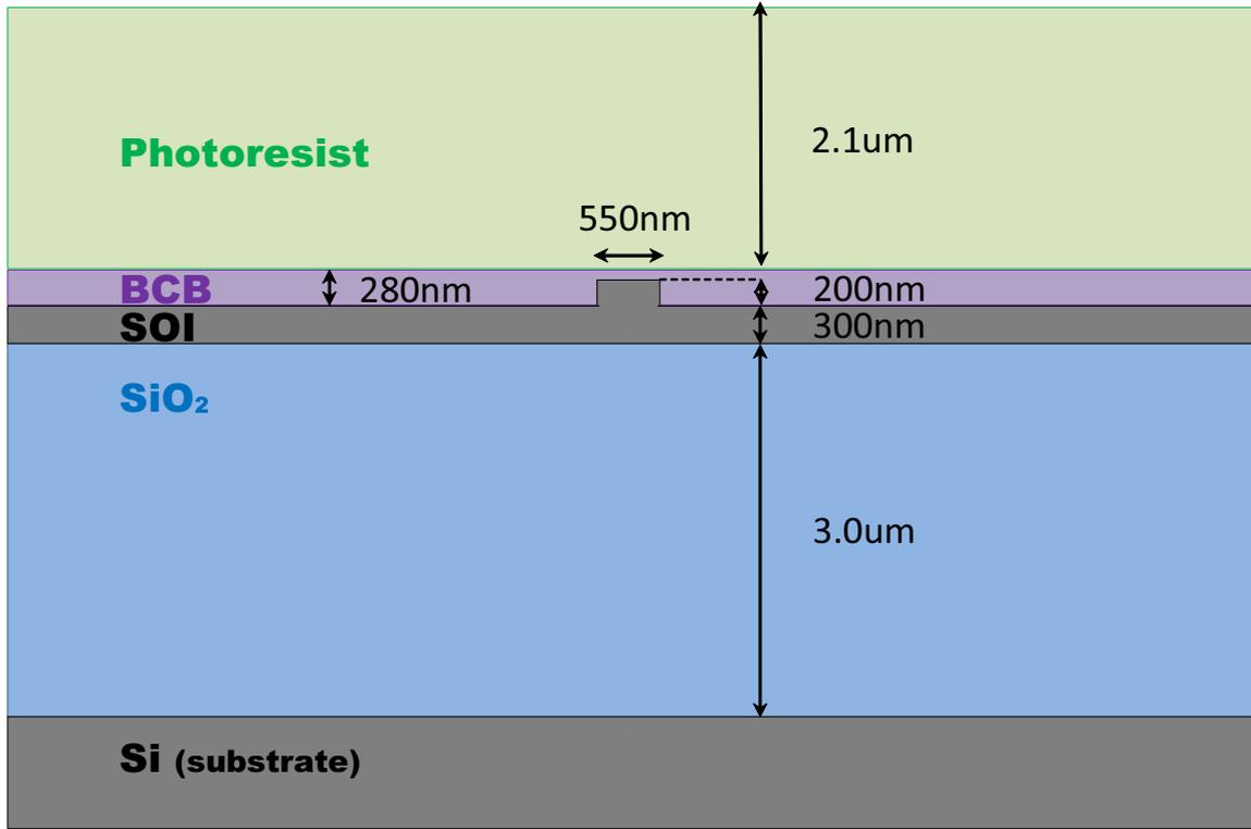
**Figure 1.3:** Schematic cross section of the used rib geometry (RIB500). The waveguides are obtained with a 200nm RIE on a 500nm SOI with a box of  $3\mu\text{m}$ . The structures are then covered with BCB polymer for bonding, and photoresist polymer for further protection.
