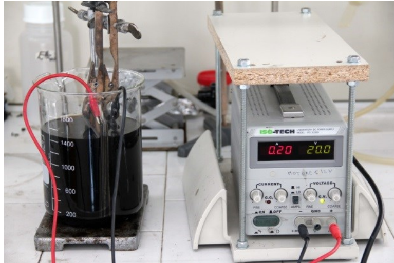
Figure 3.7. Electrophoretic deposition process, deposition of graphene oxide on glass fibers.
