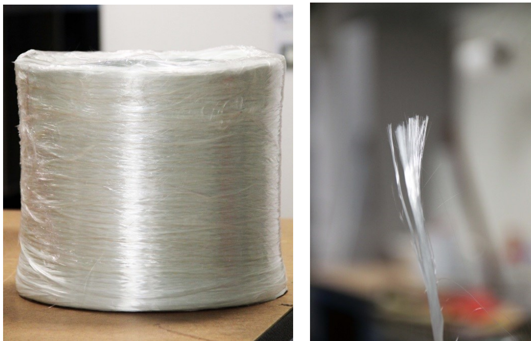
Figure 3.3. Left: PPG XG2089 Glass fiber roving, Right: close up of glass fibers.
