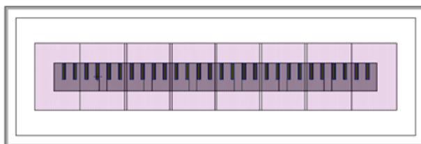
**Figure 3.13.** “Vector type” devices with beams in one row, used to evaluate reproducibility of beams over long rows. Overall chip dimensions: 7500 x 2500  $\mu\text{m}^2$ . Configuration: single well with 28 beams (300 x 60  $\mu\text{m}^2$  each).
