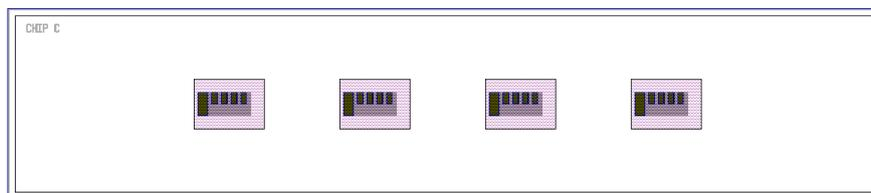
**Figure 3.11.** Main devices for sensitivity tests, compliant with Protiveris<sup>TM</sup> instrumentation for evaluation of beam deflection. Overall chip dimensions: 22400 x 5000  $\mu\text{m}^2$ . Configuration: 4 wells with 4 beams (300 x 150  $\mu\text{m}^2$  each).
