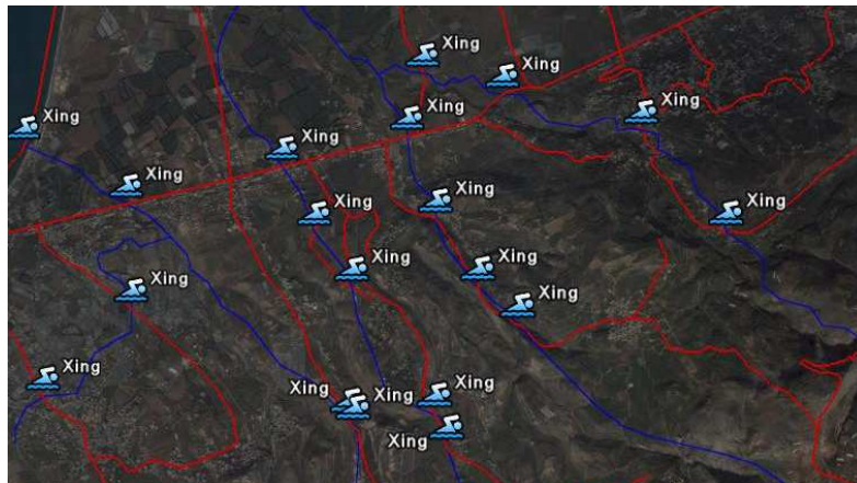
Figure 8.8: An example of automatic derived road-water crossings. The geospatial intersection function was applied to the road (red) and river (blue) networks resulting in the highlighted crossings. (Satellite image: © Space Imaging International Ltd. distributed by European Space Imaging GmbH, 2005.)
