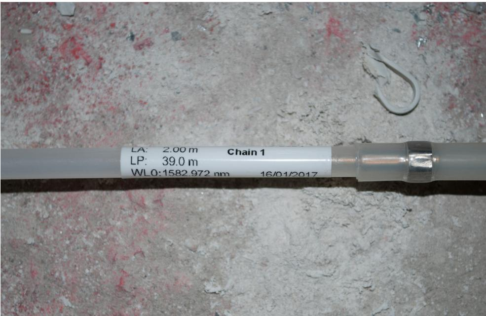
(b) Label on a FBG FOS showing an active length of 2.00 m, a passive length of 39.0 m and a nominal wavelength of 1582.972 nm
