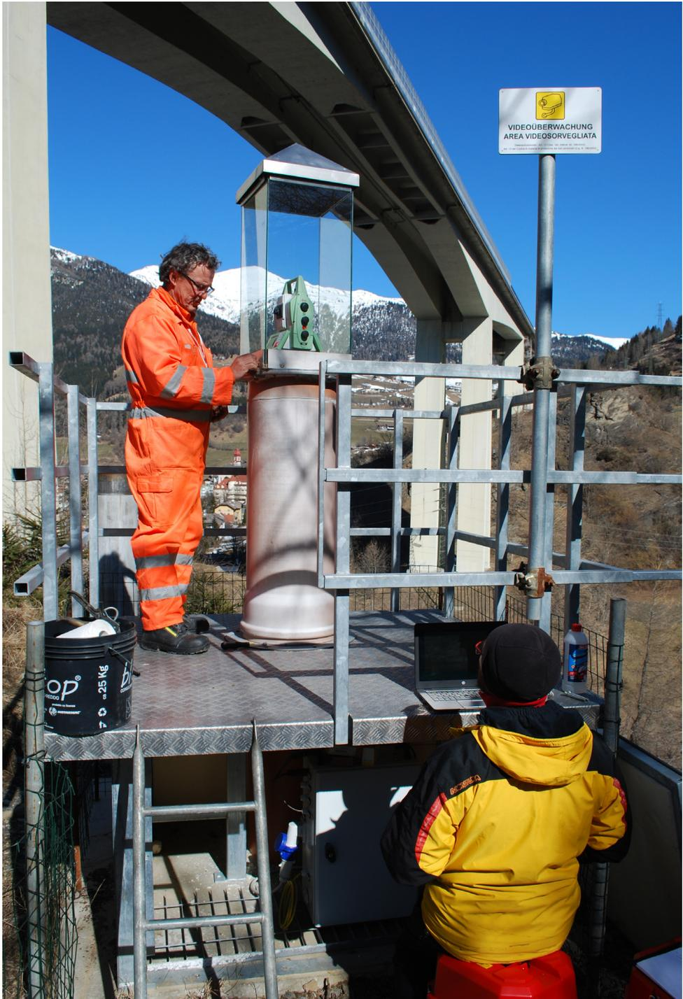
Figure 6.10. Setup of the north station Leica Nova TM50.
