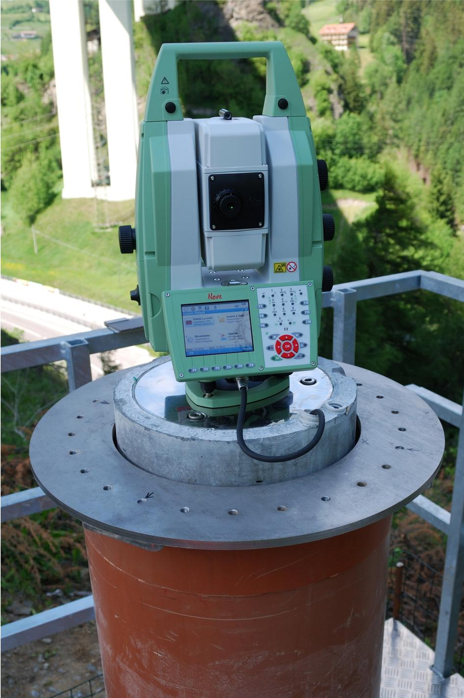
Figure 6.6. The south station, Leica Nova TM50.
