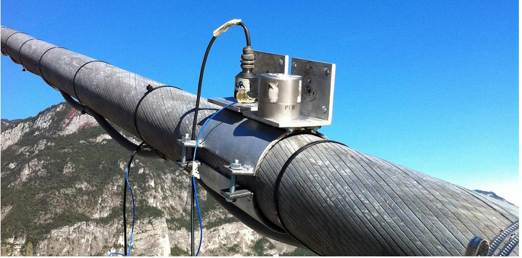
Figure 7.4. The monitoring system concept: the first natural frequency of cable 1BZ is observed using two accelerometers.
