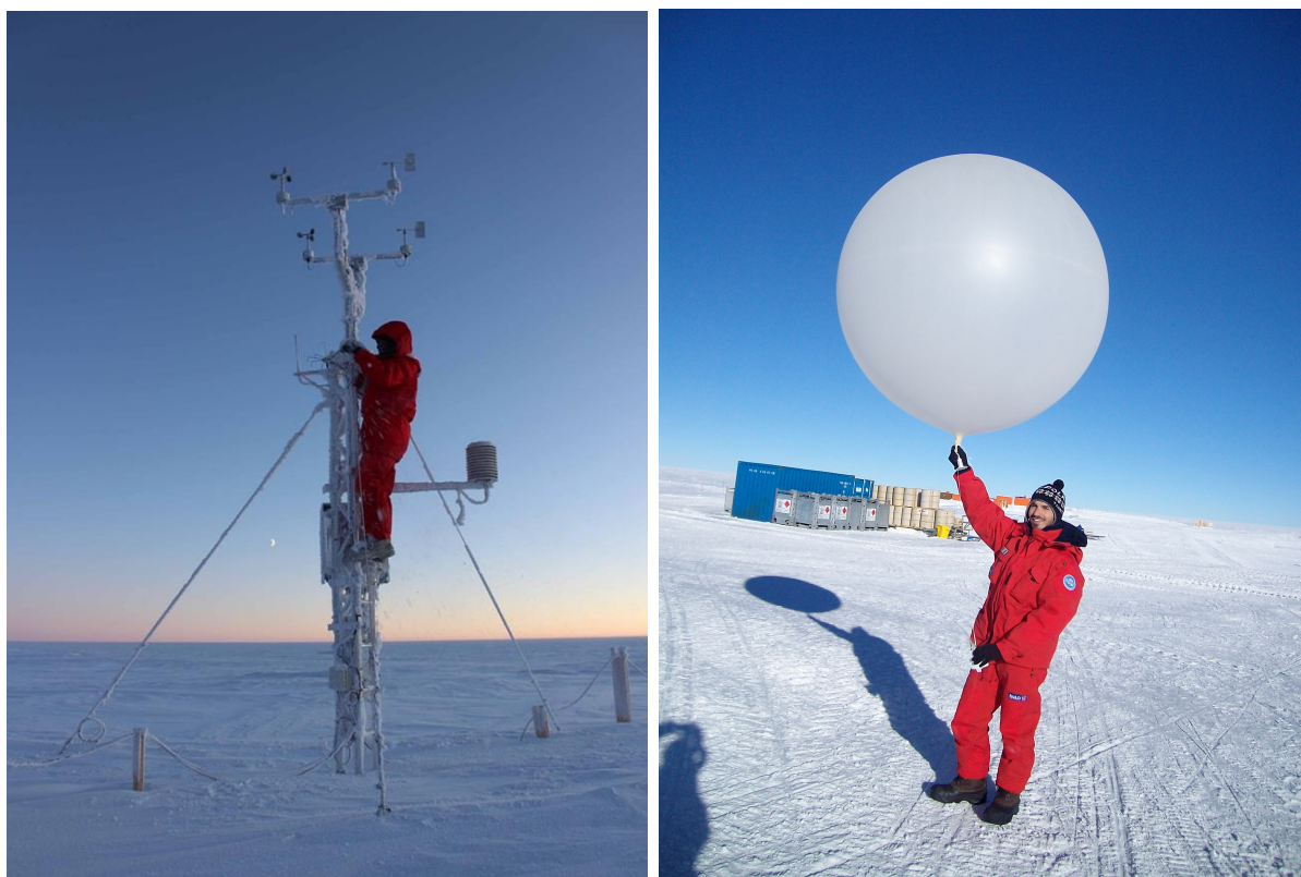
Figure 2.10: On the left: picture of routine operations on the automatic weather station Milos 520 (Vaisala) installed at Concordia station since 2005. On the right picture of a daily launch of the meteorological radiosounding for retrieving vertical profiles of meteorological variables above Concordia station (c) PNRA/IPEV
