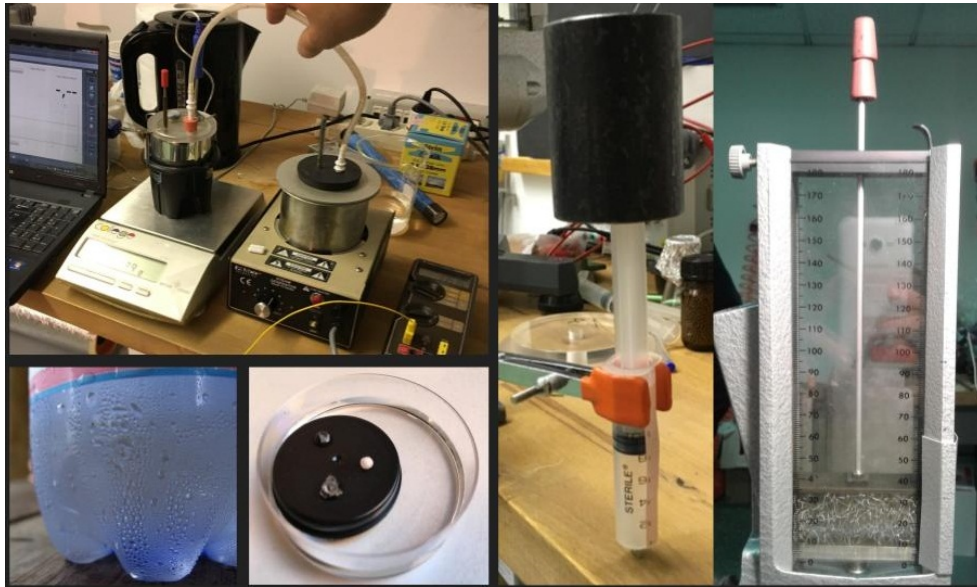
Figure 3.11: Some experimental activities: measuring the latent heat of condensation of water vapor, the dew point temperature, Boyle's law and a demonstrations of the role of hygroscopic particles and condensation nuclei.
