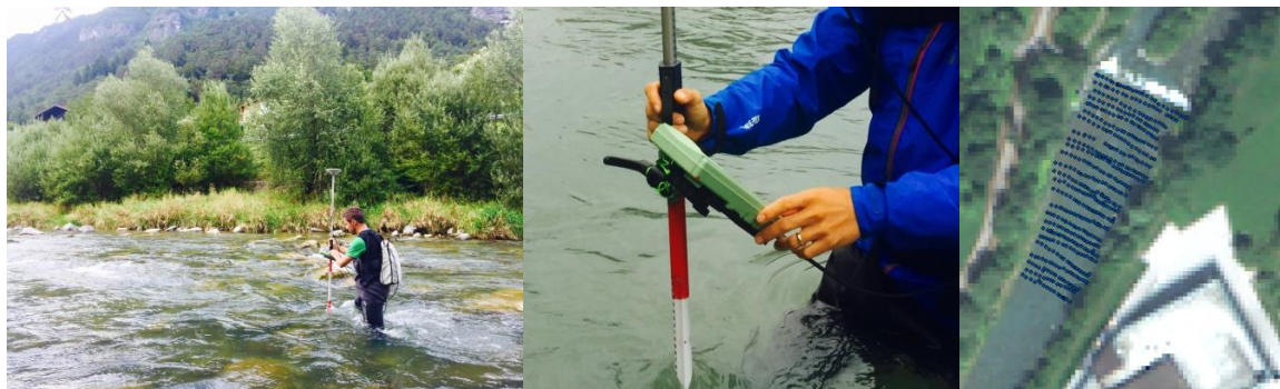
Figure 3.3 In-situ measurements of water depths in Sarca River using a RTK GPS along the cross-sections.
