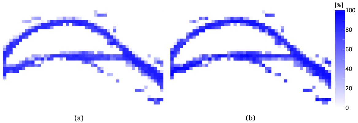
Figure 2.13 Water fractions of the WV-2 image obtained from (a) proposed OBA-NDWI method and (b) SPU algorithm.
