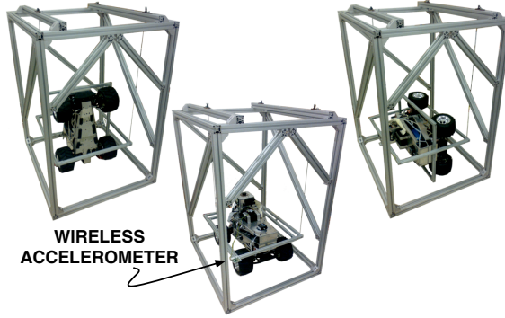
Figure 4.3: The 3-wires torsion pendulum. The frequency of oscillation around the vertical axis depends on the moment of inertia w.r.t. the same axis. By opportunely placing the vehicle on the pendulum and measuring the oscillation frequency, the moment of inertia tensor can be derived.
