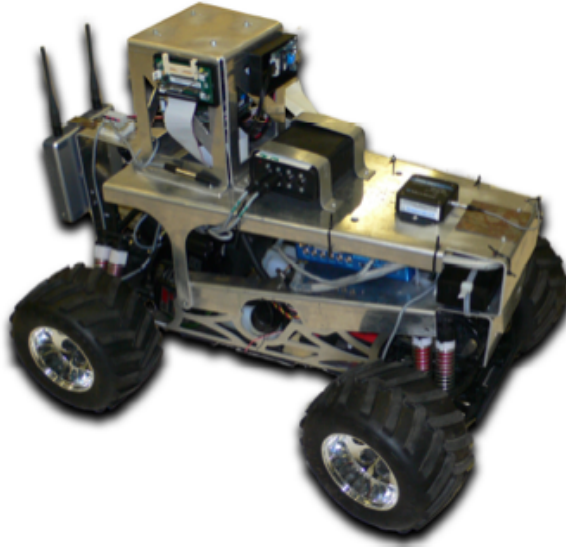
Figure 2.1: The experimental platform RUMBy. The project requirements forced the choice of a radio-controlled, 1:6 scale model of H2 Hummer, equipped with a 26 cm 3 two-strokes engine, centrifugal clutch and 4 disk brakes. The vehicle has been customized with an aluminium frame, in order to mount on the sensors, the PC104 embedded computer and the wireless router.
